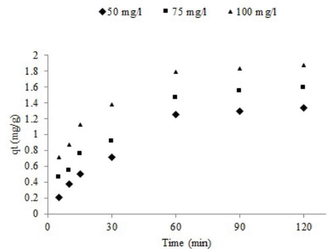
Fig. 3. Adsorbed concentration vs. adsorption time for dye removal by TAC.
