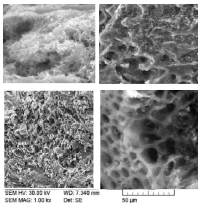
Fig. 1. SEM micrographs of the tire activated carbon.
