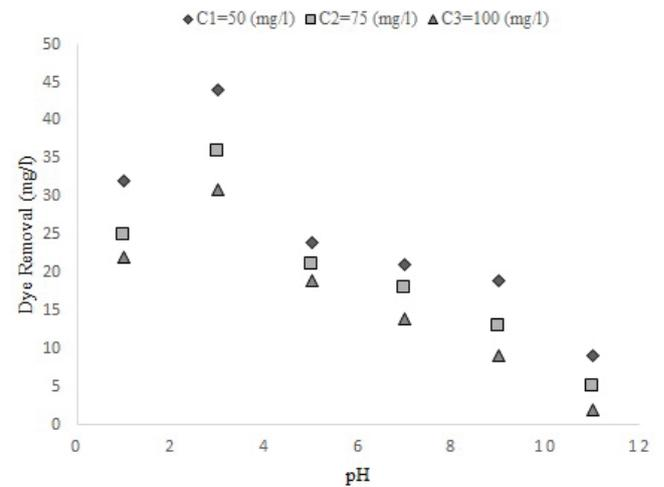
Fig. 2. Effect of pH on the removal of dye by TAC at 20°C.
