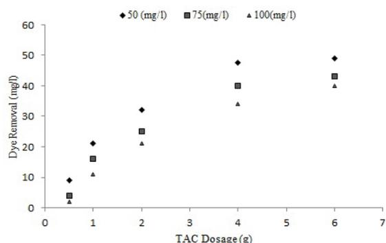
Fig. 4. Effect of sorbent mass on the dye removal by TAC.
