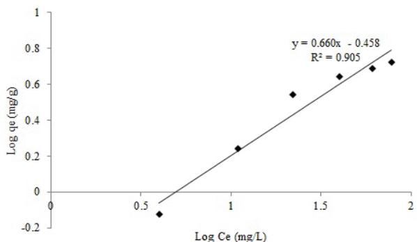
Fig. 5. Freundlich and Langmuir adsorption isotherms for the dye removal.
