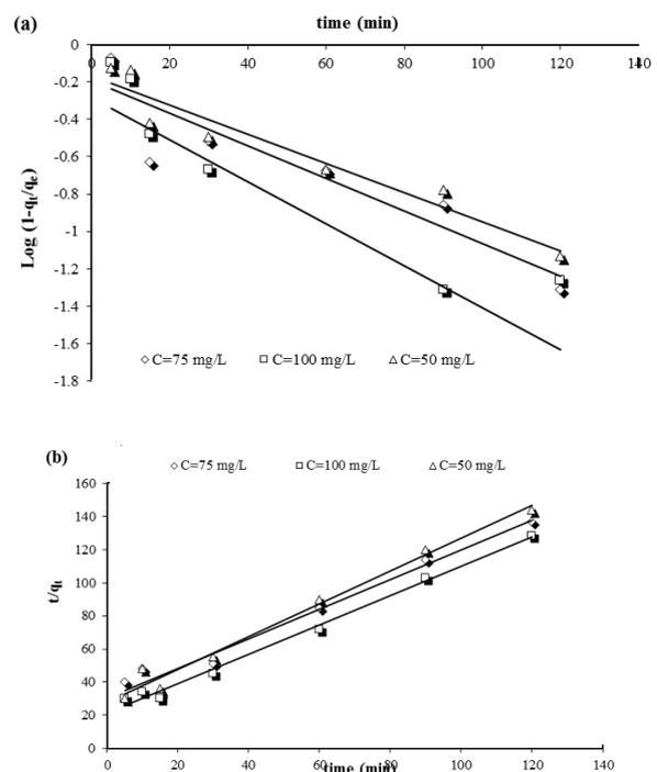
Fig. 6. Plots for kinetic models for the adsorption of Methylene blue onto TAC.
