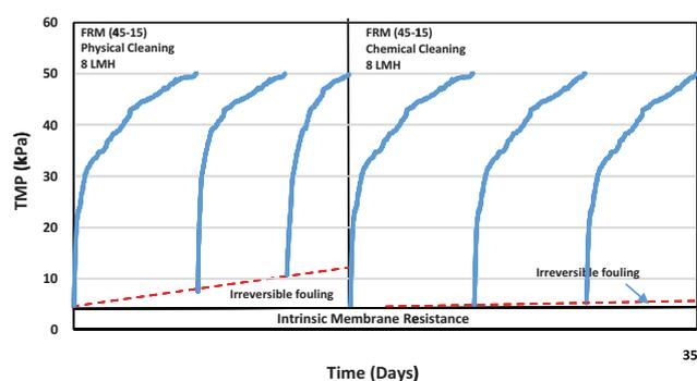
Fig. 3. TMP profile with physical and chemical cleaning.
