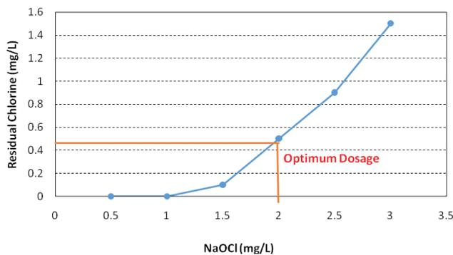
Fig. 5. Optimum dosage of chlorine for water disinfection.
