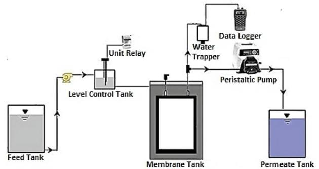
Fig. 1. Schematic diagram of membrane-based septic tank (MBST).
