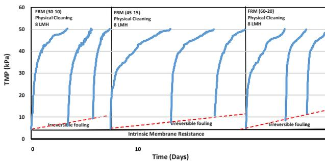
Fig. 2. TMP profiles under filtration to relaxation modes (FRM) with physical cleaning.
