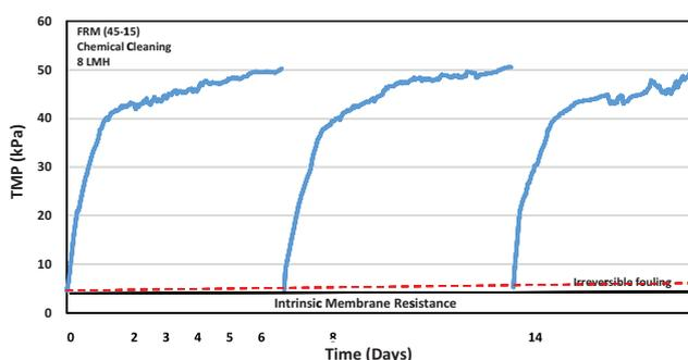
Fig. 4. TMP profile of WFMF membrane using an on-site water treatment technology.
