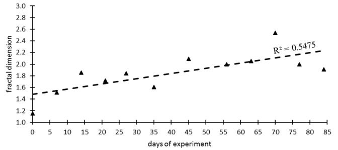
Fig. 5. Fractal dimension of particles in the tank with PET bottles.
