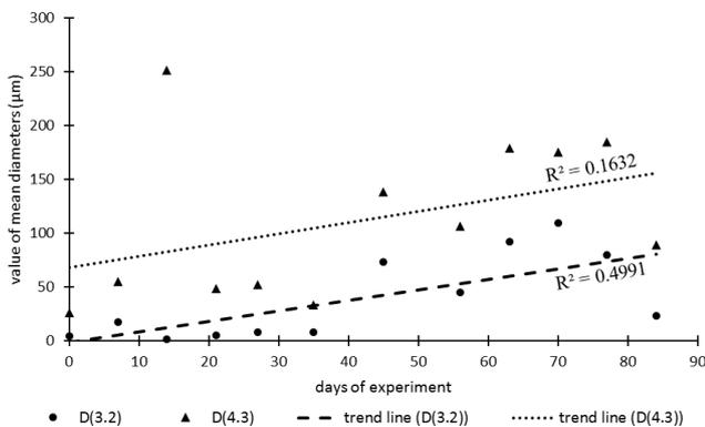
Fig. 9. Mean diameters D(3.2) and D(4.3) determined for particle size distribution of suspension in the tank with anti-erosive mats.
