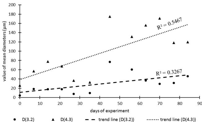
Fig. 10. Mean diameters D(3.2) and D(4.3) determined for particle size distribution of suspension in the tank with mixed substrates.
