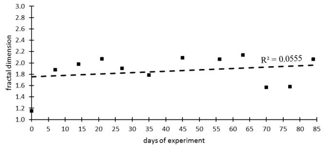
Fig. 7. Fractal dimension of particles in the tank with mixed substrates.
