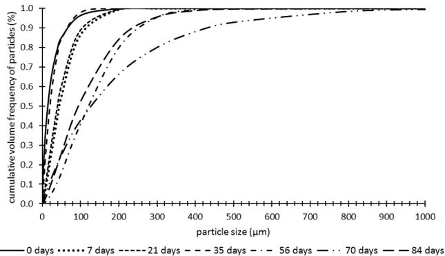
Fig. 4. Cumulative volume frequency of particles diameter in the tank with mixed substrates.
