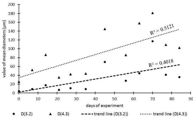
Fig. 8. Mean diameters D(3.2) and D(4.3) determined for particle size distribution of suspension in the tank with PET bottles.
