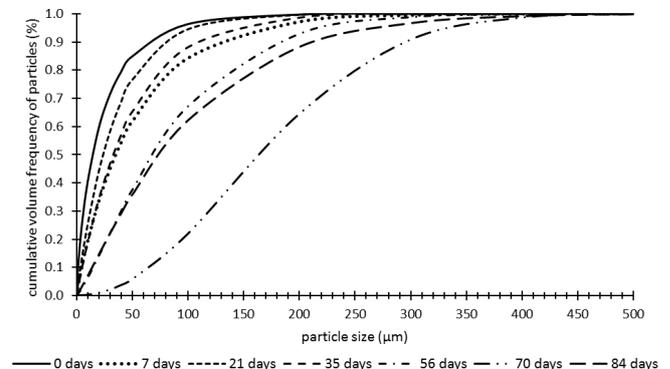
Fig. 2. Cumulative volume frequency of particles diameter in the tank with PET bottles.
