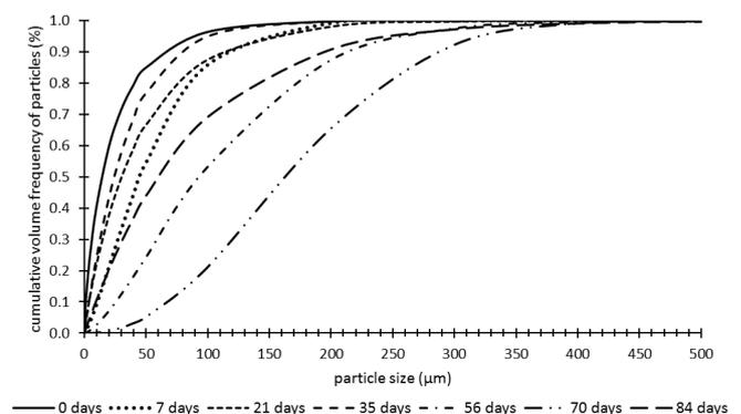
Fig. 3. Cumulative volume frequency of particles diameter in the tank with anti-erosive mats.
