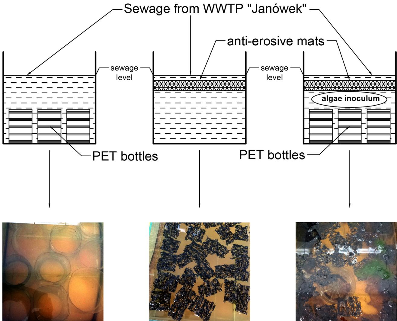
Fig. 1. Plan of the experimental setup. Tanks with sewage and types of artificial substrates for the immobilization of algae.
