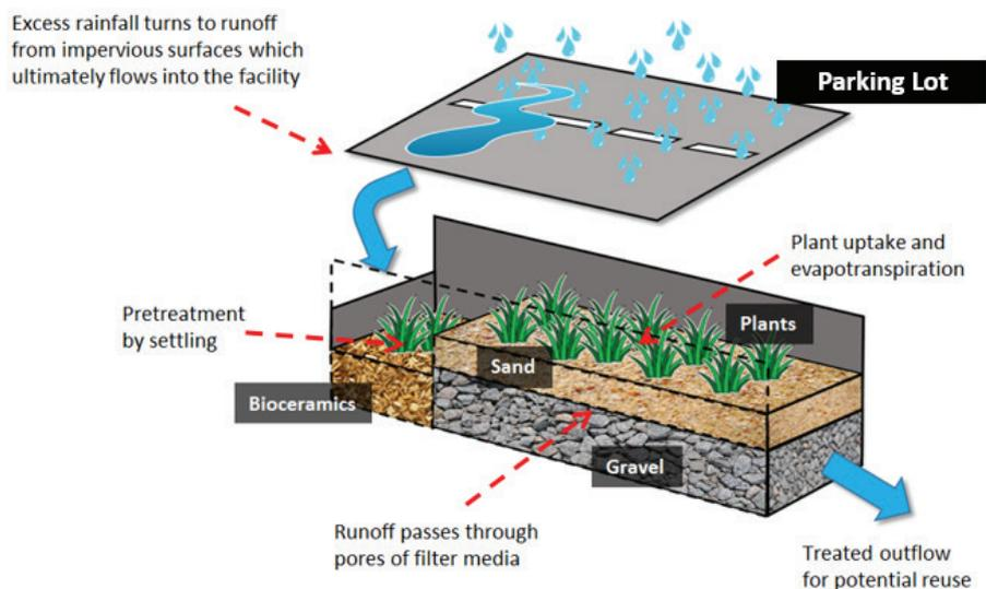
Fig. 1. Schematic diagram and design strategy of the HSSF wetland.
