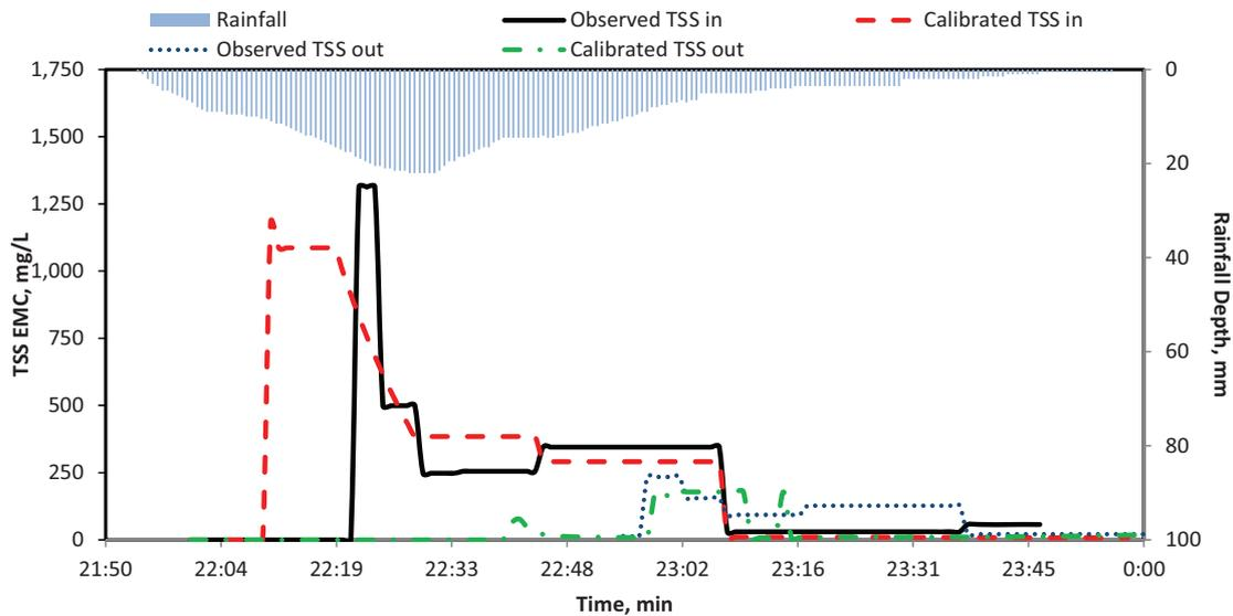
Fig. 4. Representative TSS polluto-graph for water quality calibration model of the HSSF wetland.
