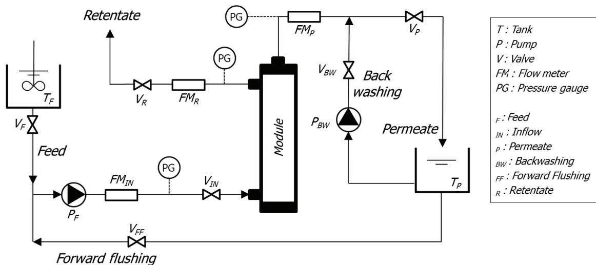
Fig. 1. Experimental setup of pressurized UF membrane system.
