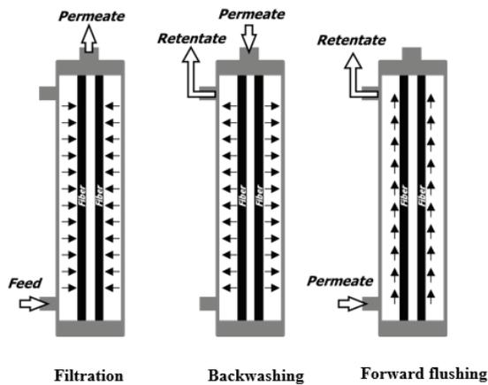
Fig. 2. Schematic description of the filtration, backwashing and forward flushing.
