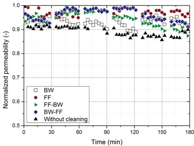
Fig. 3. Normalized membrane permeability registered with a permeate flux of 50 LMH for different cleaning strategy.
