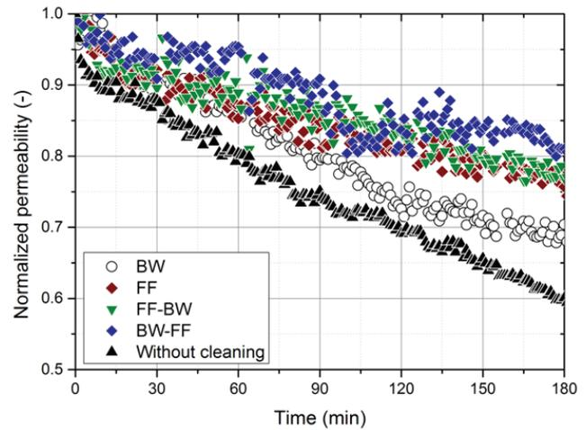
Fig. 4. Normalized membrane permeability obtained at a permeate flux of 100 LMH for different cleaning strategies.
