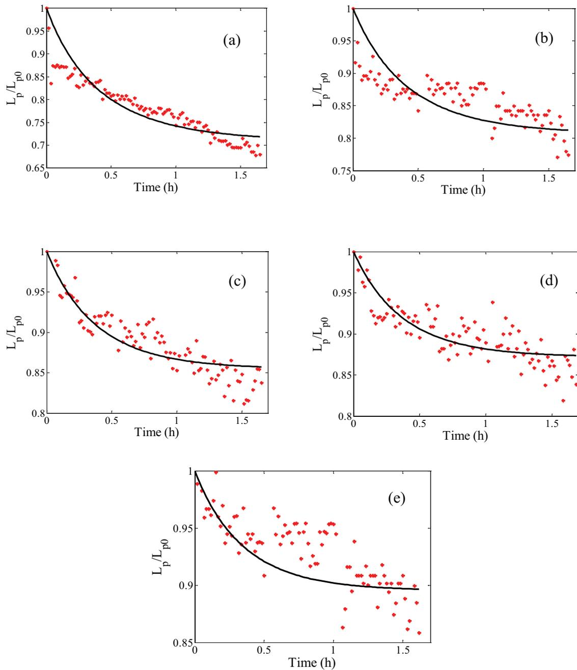
Fig. 5. Comparison of model simulations and normalized permeability experimental data for different cleaning strategies (a) without cleaning, (b) F/BW (30 min/60 s), (c) F/FF (30 min/60 s), (d) F/FF/BW (30 min/30 s/30 s), (e) F/BW/FF (30 min/30 s/30 s).
