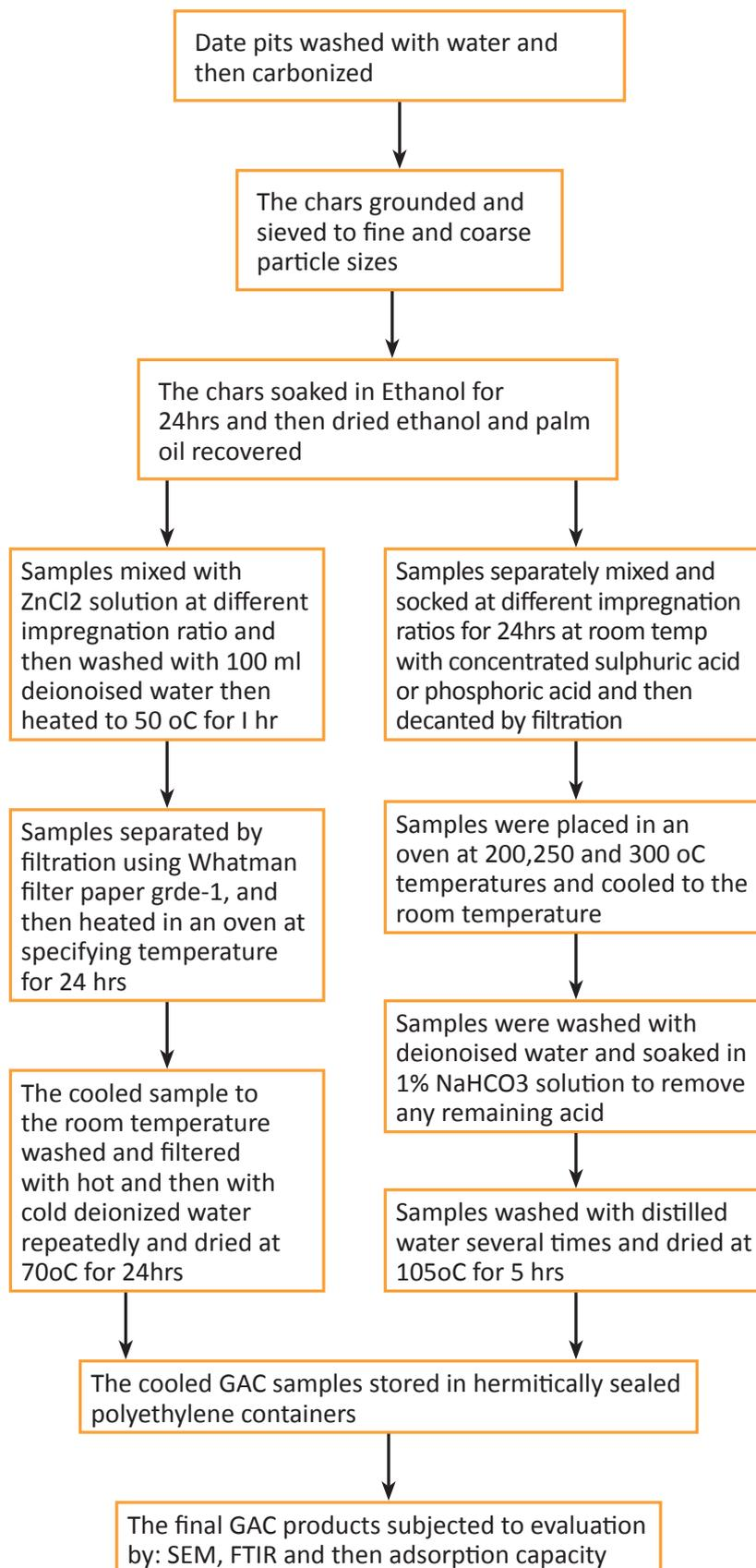
Fig. 2. Activation procedure of dates pits to produce GAC.
