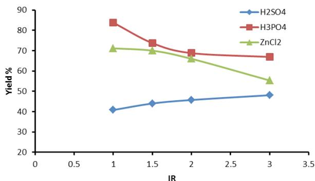
Fig. 10. Variations of GAC percentage yield with IR using sulphuric acid, phosphoric acid and zinc chloride, with 48 h activation time and heated at 200°C.
