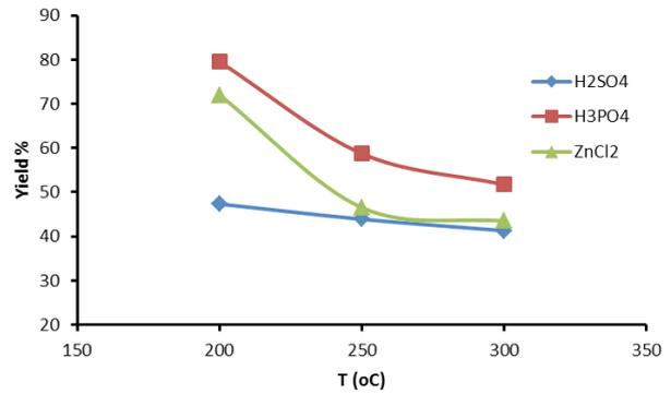
Fig. 5. Variations of GAC percentage yield with the activation temperature when using sulphuric acid, phosphoric acid and zinc chloride as dehydrating agents, IR = 2, heated for 24 h.
