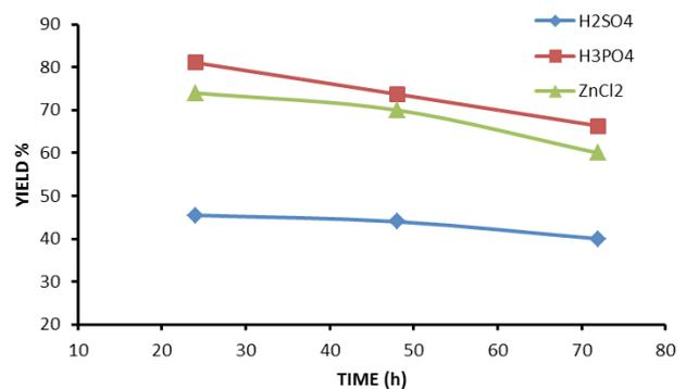
Fig. 7. Variations of GAC percentage yield with activation time using sulphuric acid, phosphoric acid and zinc chloride at IR = 1.5 and at 200°C.
