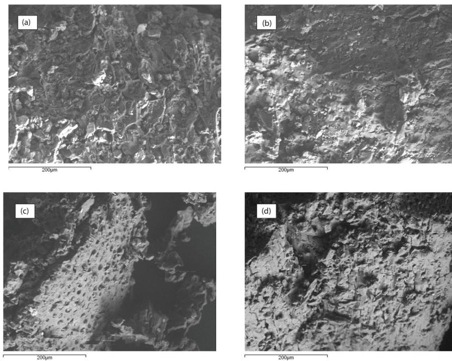
Fig. 15. SEM micrographs of GAC activated by  $ZnCl_2$  at different conditions. (A) GAC activated at IR=1, activation temperature = 200°C, activation time = 24 h; (B) GAC activated at IR = 2, activation time = 24 h, activation temperature = 200°C; (C) GAC activated at IR = 1, activation temperature = 300°C, activation time = 24 h; (D) GAC activated at IR = 1; activation time = 24 h, activation temperature = 200°C, fine chars (<0.5 mm particle size).
