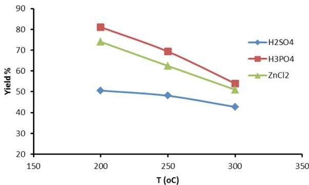
Fig. 4. Variations of percentage yield of GAC with the activation temperature using sulphuric acid, phosphoric acid and zinc chloride as dehydrating agents, IR = 1.5, heated for 24 h.
