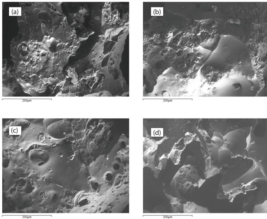
Fig. 14. SEM micrographs of GAC activated by  $H_3PO_4$  at different conditions. (A) GAC activated at IR = 1, activation time = 24 h, activation temperature = 200°C; (B) GAC activated at IR = 2, activation time = 24 h, activation temperature = 200°C; (C) GAC activated at IR = 1, activation temperature = 300°C, activation time = 24 h; (D) GAC activated at IR = 1, activation time = 24 h, activation temperature = 200°C, fine chars (<0.5 mm particle size).
