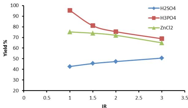
Fig. 9. Variations of GAC percentage yield with IR using sulphuric acid, phosphoric acid and zinc chloride, with 24 h activation time and heated at 200°C.
