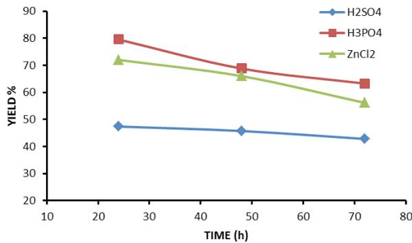
Fig. 8. Variations of GAC percentage yield with activation time using sulphuric acid, phosphoric acid and zinc chloride, at IR = 2 and at 200°C.
