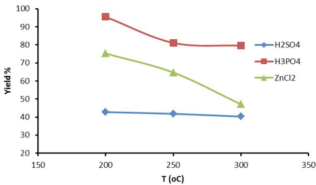
Fig. 3. Variations of percentage yield of GAC with activation temperature when using sulphuric acid, phosphoric acid and zinc chloride, IR = 1 and heated for 24 h.
