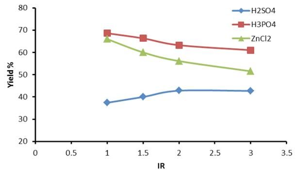
Fig. 11. Variations of GAC percentage yield with IR using sulphuric acid, phosphoric acid and zinc chloride, with 72 h activation time and heated at 200°C.
