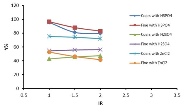
Fig. 12. Char particle size effect on GAC yield percentage when activated at temperature 200°C and time 24 h for all dehydrating agents.
