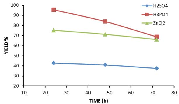
Fig. 6. Variations of GAC percentage yield with activation time using sulphuric acid, phosphoric acid and zinc chloride, at IR = 1 and at 200°C.
