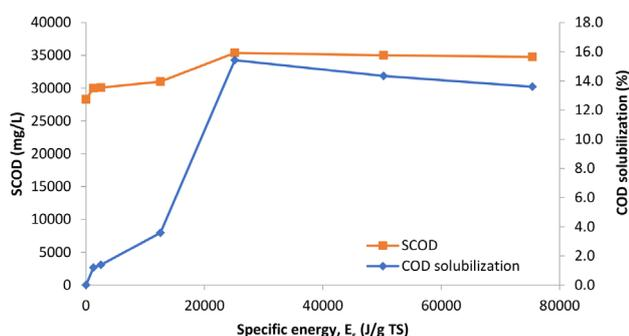
Fig. 6. Disintegration of POME using various sonication energies.
