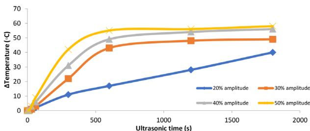
Fig. 3. Temperature profile with different ultrasonication time and amplitude.
