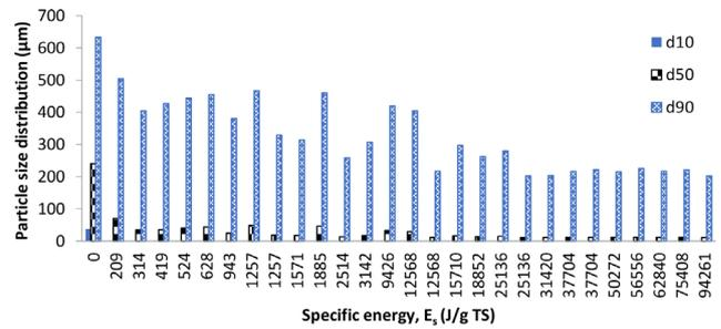
Fig. 2. Influence of specific energy on particle size distribution.
