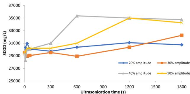
Fig. 5. Effect of ultrasonication parameters on the solubilization of POME in terms of SCOD.
