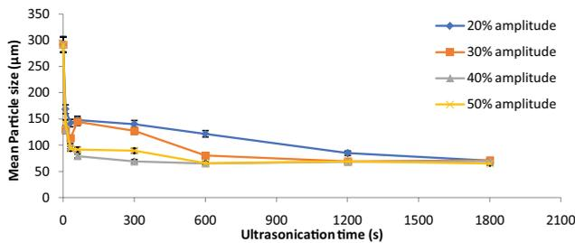
Fig. 1. Effect of ultrasonication amplitude on mean particle size.
