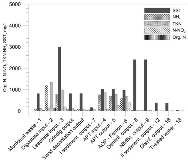
Fig. 6. Nitrogen and SST concentrations along the treatment line.
