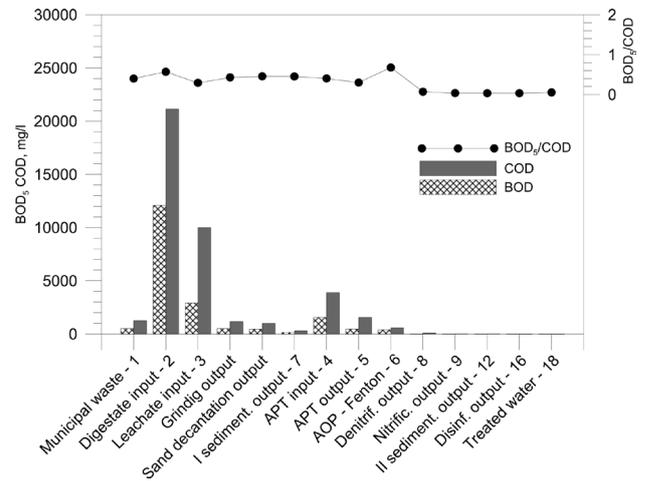
Fig. 5. BOD<sub>5</sub>, COD and their ratio along the treatment line.
