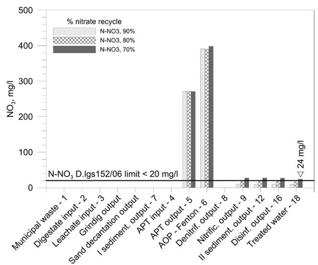
Fig. 9.  $N-NO_3$  concentration as a function of percentage nitrate recycle.
