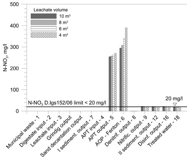
Fig. 8.  $N-NO_3$  concentration as a function of leachate volume.
