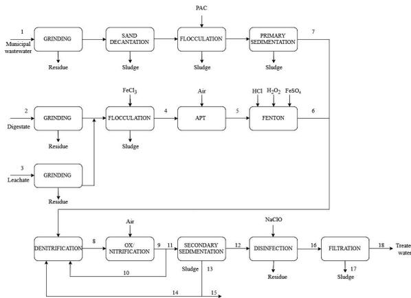
Fig. 4. Block scheme of the simulated process.
