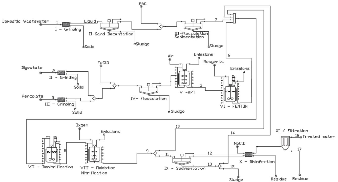
Fig. 3. Process scheme simulated by SuperPro Designer.
