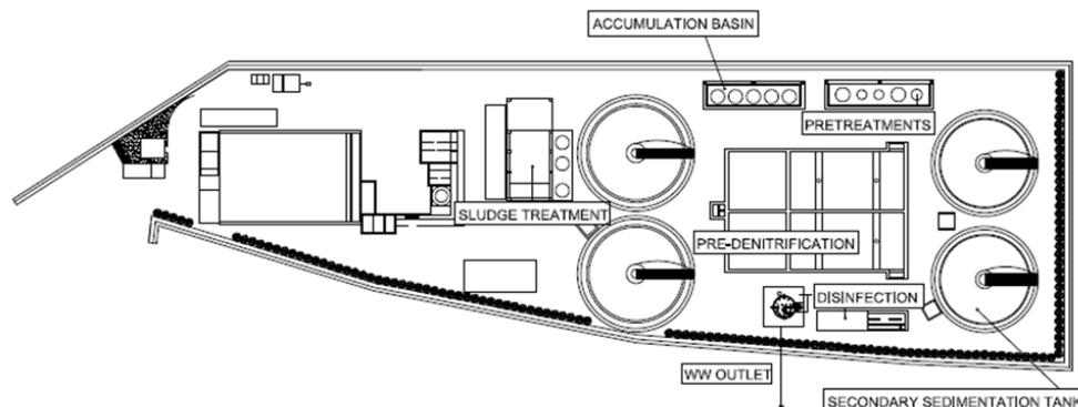
Fig. 1. Current configuration of wastewater treatment plant in Calabritto.
