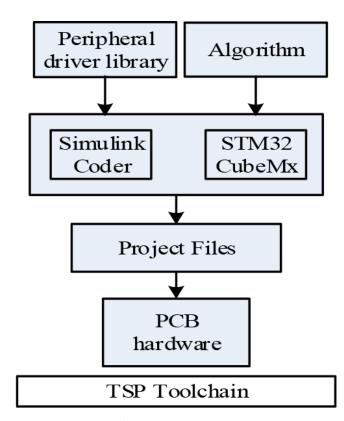
Fig. 3. TSP structure diagram.
