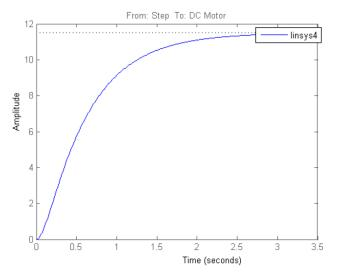
Fig. 6. Motor simulation curve.
