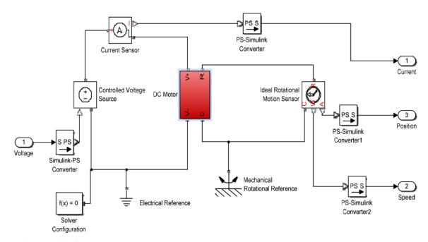
Fig. 5. Simulation model of DC motor simscape.
