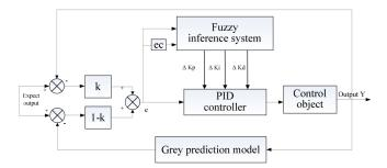
Fig. 7. Structure of grey prediction fuzzy-PID control for irrigation.
