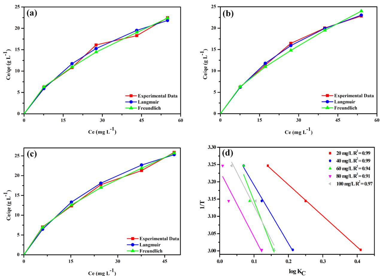
Fig. 5. Adsorption of DCR at different temperature isotherm comparison ((a) 310 K, (b) 318 K and (c) 333 K) and (d) Van't Hoff plot for DCR adsorption on CIFIC.
