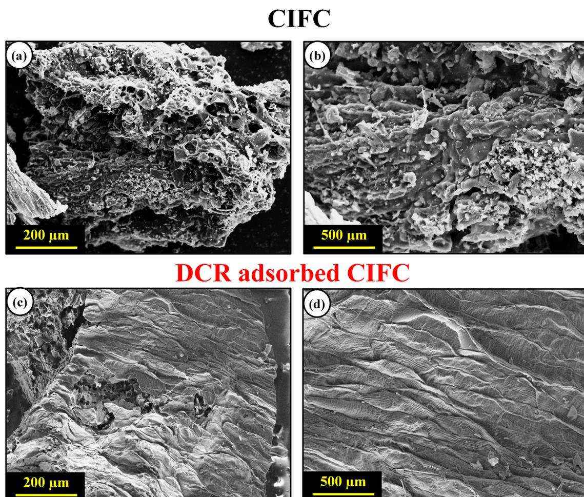
Fig. 2. SEM image of CIFIC unloaded DCR (a, b), CIFIC loaded DCR (c, d).
