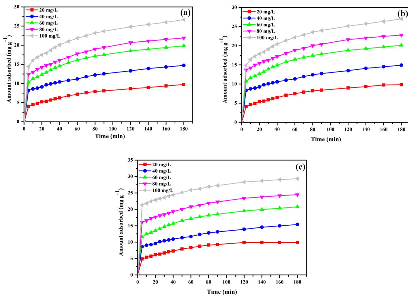
Fig. 4. Contact time and dyes initial concentration at different temperature (a) 310 K, (b) 318 K and (c) 333 K.
