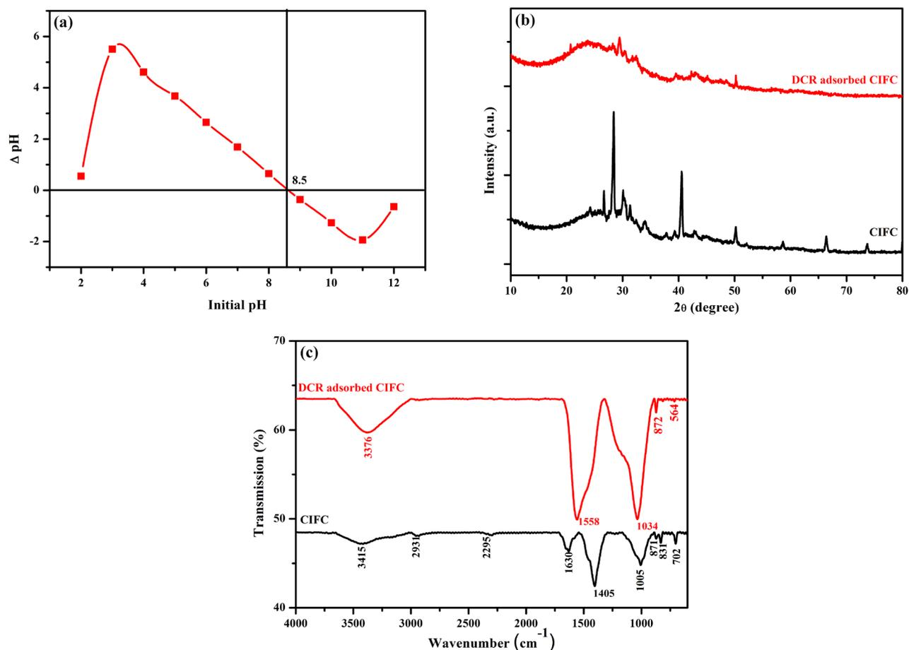
Fig. 1(a) Determination of zero-point charge, (b) XRD pattern and (c) FT-IR spectrum of CIFIC and DCR adsorbed CIFIC.
