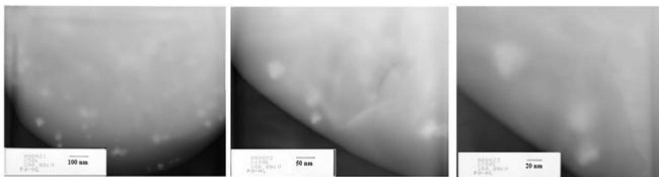
Fig. 5. TEM images of metal nanoparticles from p(AA)-Pd (white spots can be considered as Pd nanoparticles).
