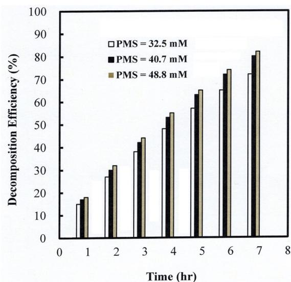
Fig. 5. Decomposition efficiency of peroxymonosulfate anions in a variety of peroxymonosulfate concentrations during the experiments under the conditions of electrode potential = 6 V,  $T = 318$  K and initial pH = 3.0.
