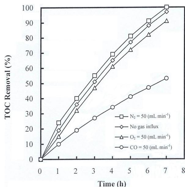
Fig. 3. Effect of dosage of nitrogen, oxygen and carbon monoxide gases on the TOC removal percentage by electro-activated peroxymonosulfate oxidation under the conditions of electrode potential = 6 V, T = 318 K, peroxymonosulfate anion concentration = 40.7 mM and initial pH = 3.0.
