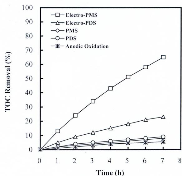
Fig. 1. Time-dependent patterns of TOC removal percentage by means of peroxydisulfate alone, peroxymonosulfate alone, anodic oxidation, electro-activated peroxydisulfate and electro-activated peroxymonosulfate oxidation respectively under the conditions of electrode potential = 6 V, T = 303 K, peroxydisulfate anion concentration = 105.0 mM, peroxymonosulfate anion concentration = 40.7 mM and initial pH = 3.0.
