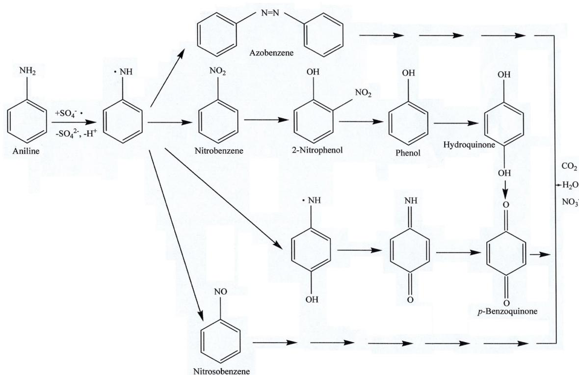
Fig. 7. Plausible reaction pathways of aniline in aqueous solution by electro-activated peroxymonosulfate oxidation.
