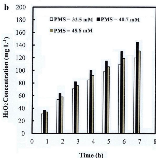
Fig. 4. (a) Effect of peroxymonosulfate anion concentrations on the TOC removal percentage by electro-activated peroxymonosulfate oxidation under the conditions of electrode potential = 6 V, T = 318 K and initial pH = 3.0. (b) Hydrogen peroxide concentrations generated in deionized water by electro-activated peroxymonosulfate anions with various peroxymonosulfate anion concentrations under the conditions of electrode potential = 6 V, T = 318 K and initial pH = 3.0.
