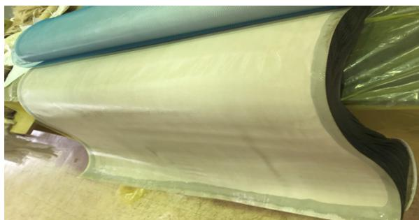
Fig. 14. Membrane discoloration from feed (right) to product (left) end.
