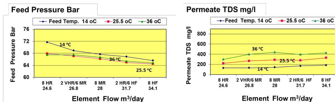
Fig. 5. The effect of SWRO membrane properties on permeate TDS and feed pressure in hybrid and non-hybrid designs.
