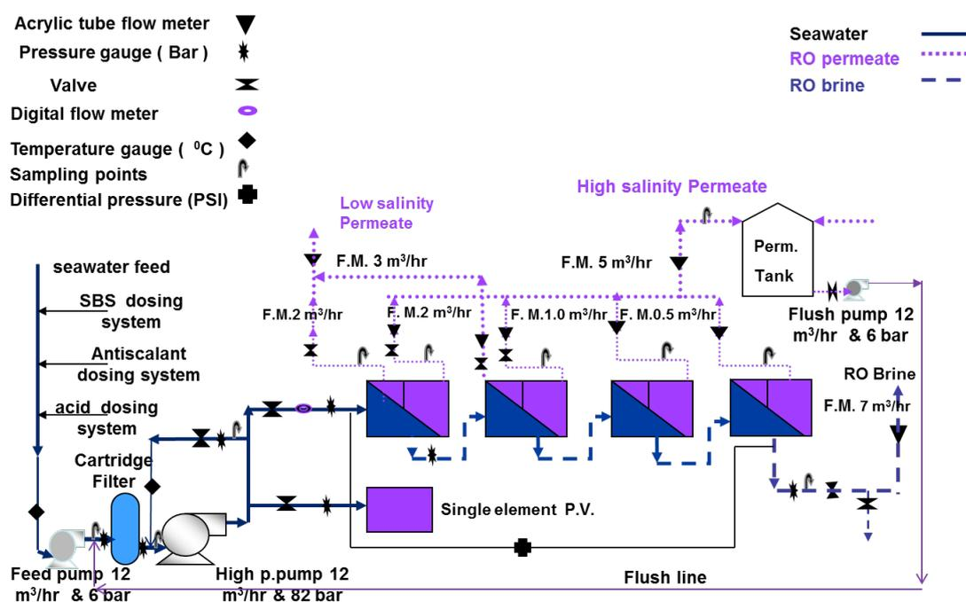
Fig. 1. SWRO unit (four pressure vessels connected in series, each containing two SWRO elements of 8" × 40").
