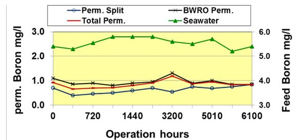
Fig. 12. Boron concentration in seawater feed and different permeates.
