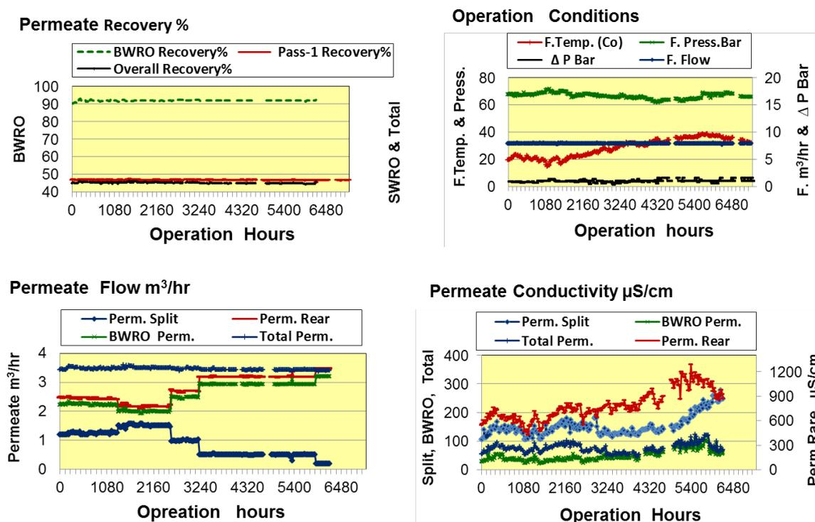
Fig. 7. Operation and performance parameters of Hybrid-1 (split partial two pass design) for 6100 hours of operation.
