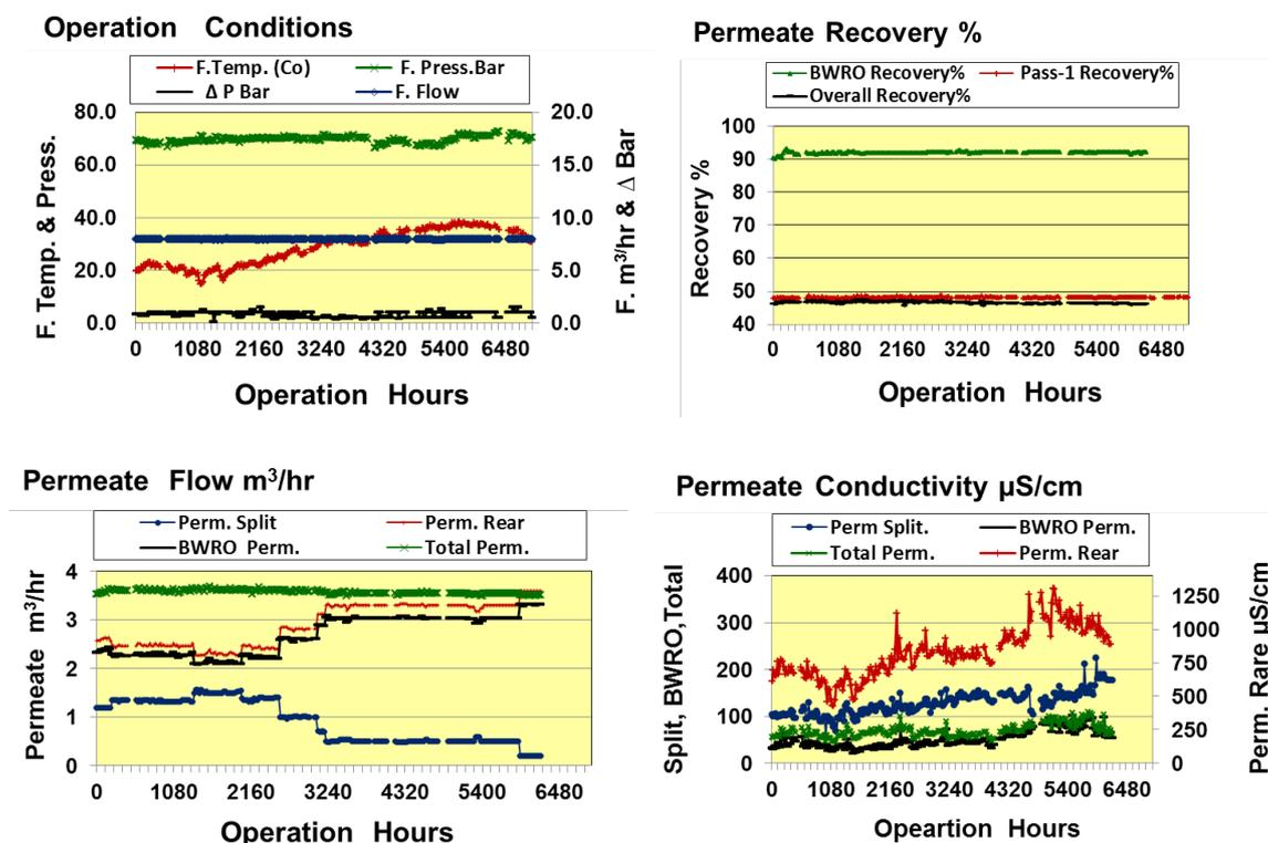
Fig. 8. Operation and performance parameters of Hybrid-2 (split partial two pass design) for 6100 h of operation.
