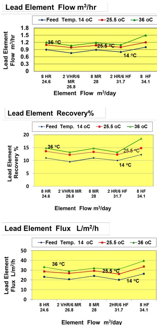
Fig. 6. Lead element flux rate, recovery and flow for various hybrid and non-hybrid designs.
