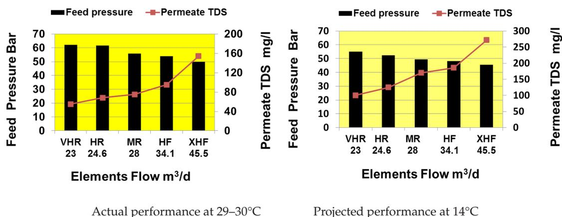
Fig. 3. Comparison of the actual and projected performances of five different SWRO elements.
