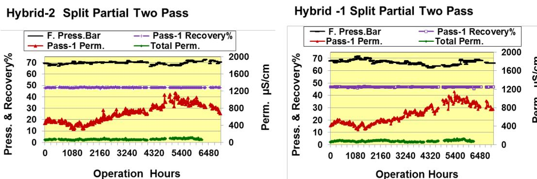
Fig. 10. Comparison of the performances of Hybrid-1 and Hybrid-2 split partial two pass designs for 6100 h of operation.
