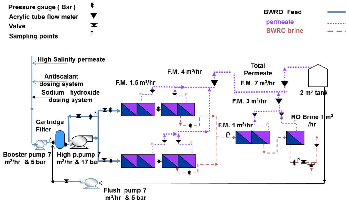
Fig. 2. BWRO unit (2×8 BWRO elements of 4" × 40" in the first stage and 6 elements in the second stage).
