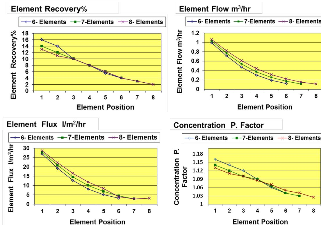
Fig. 4. Projected individual element flow, recovery, and flux and concentration polarization of 3 different configurations.
