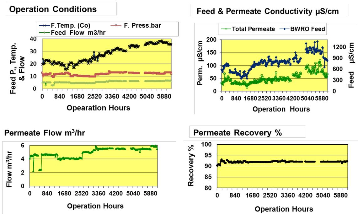
Fig. 9. Operation and performance parameters of second pass BWRO for 6100 h of operation.
