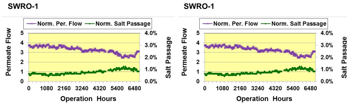
Fig. 11. Normalized salt passage and permeate flow of SWRO-1 and SWRO-2.
