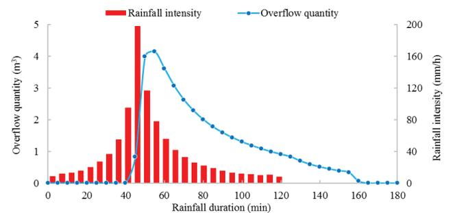
Fig. 9. Rainfall process and stimulation of overflow quantity.
