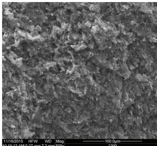
Fig. 1. SEM image of the NJ sludge.
