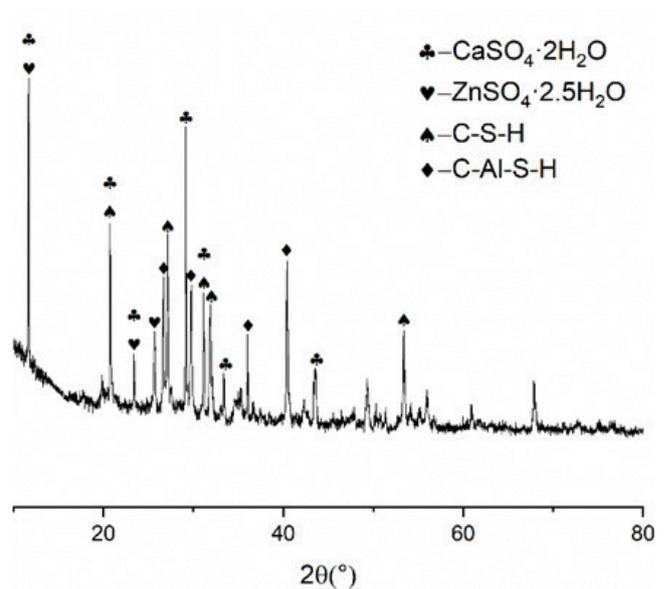
Fig. 5. XRD spectra of the S/S solid of the NJ sludge after curing with HAS.
