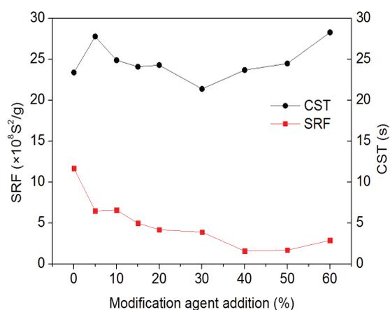
Fig. 3. SRF and CST of the GZ sludge change with the addition of modification agent.
