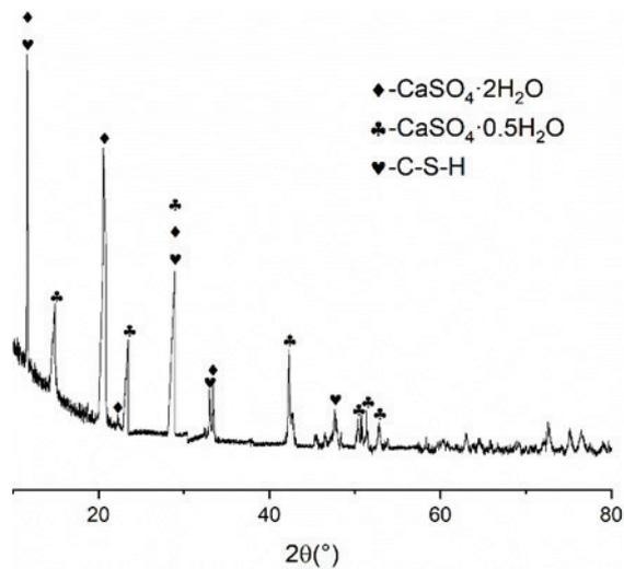
Fig. 6. XRD spectra of the S/S solid of the GZ sludge after curing with HAS.
