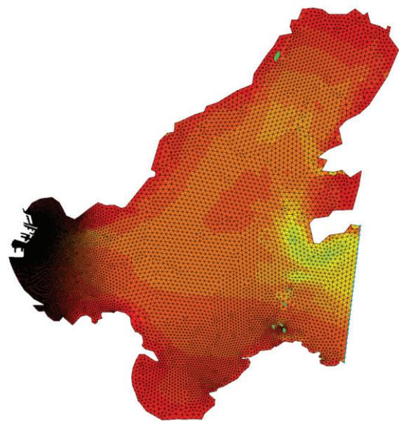
Fig. 1. Mesh generation of 2-d numerical model for tidal current in Bohai Sea.
