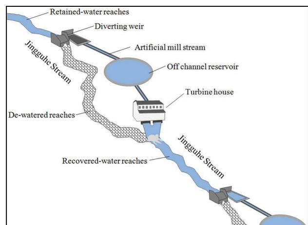
Fig. 1. Scheme of typical bypass-type hydropower stations.
