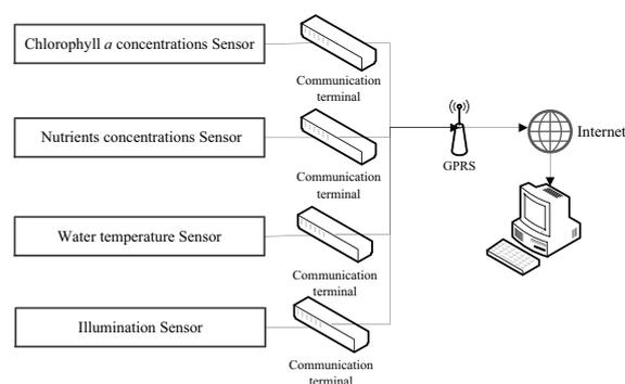
Fig. 2. Structural diagram of algae bloom multi-sensor monitor system.
