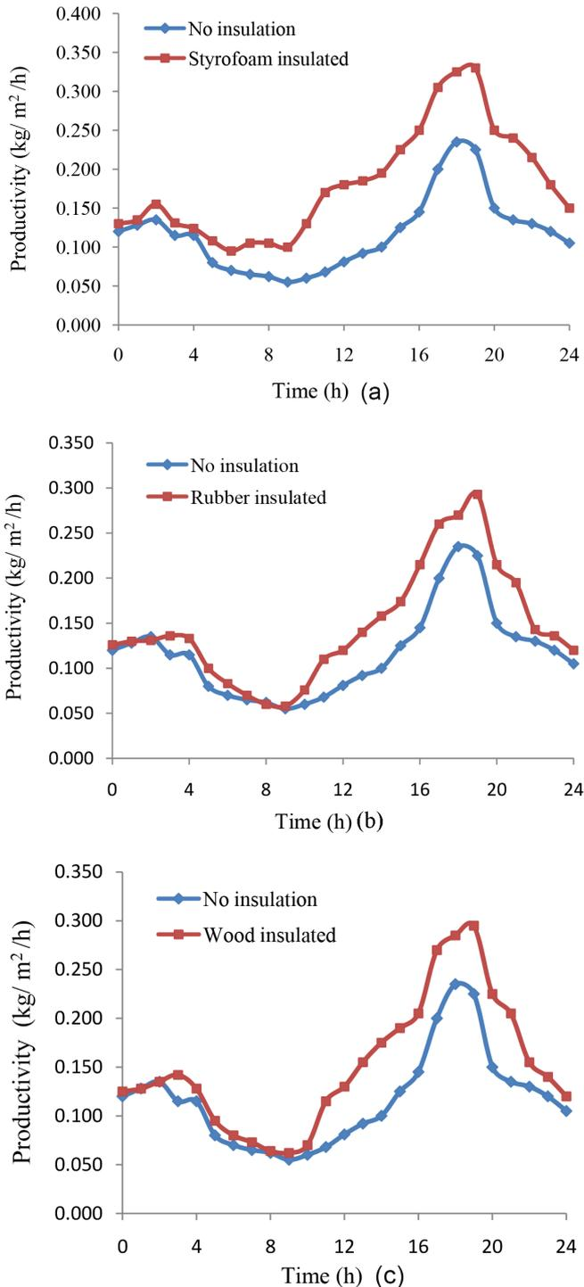
Fig. 5. Comparison of productivity of the solar still with insulation and without insulation.
