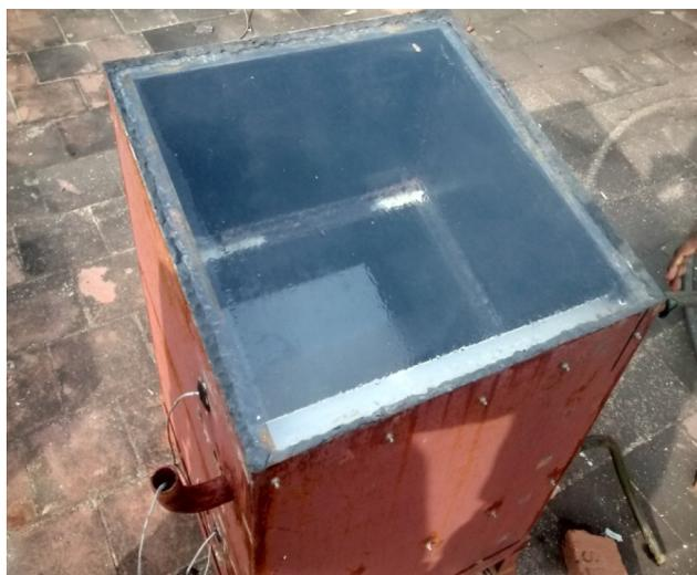
Fig. 2. Photographic view of Stacked solar still.
