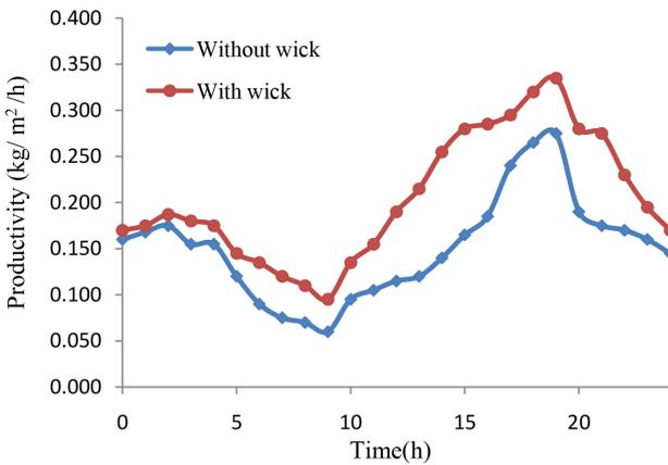
Fig. 9. Effect of wick material on the productivity of solar still.
