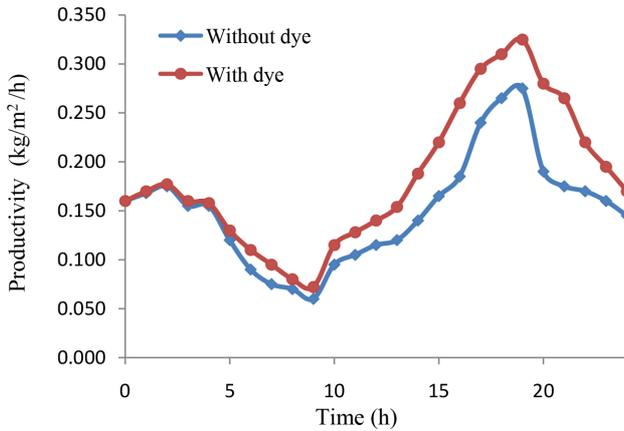
Fig. 7. Effect of dye on the productivity of the solar still.
