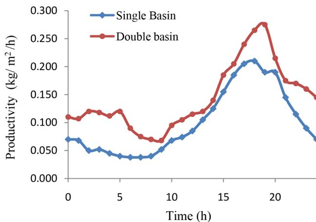
Fig. 3. Comparison of the productivity of single basin and stacked solar still.
