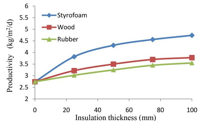
Fig. 6. Effect of insulation thickness on the productivity of the solar still.
