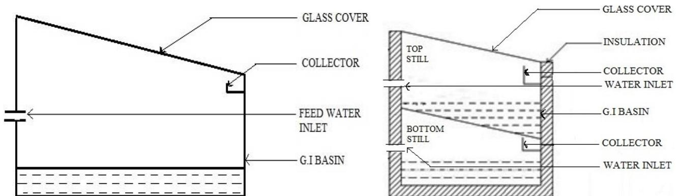
Fig. 1. Schematic representation of a solar still (a) Single basin solar still (b) Stacked solar still.
