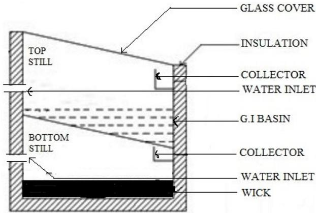
Fig. 8. Schematic diagram of solar still with wick material.
