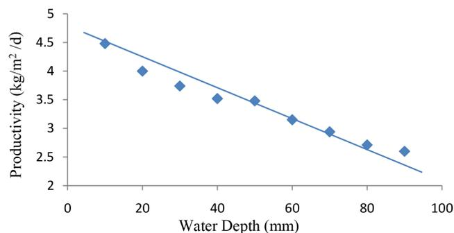
Fig. 4. Effect of water depth on the productivity of stacked solar still.
