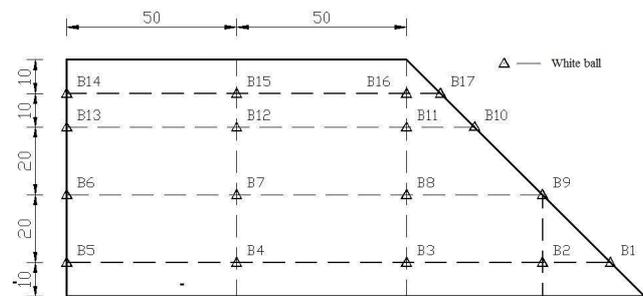
Fig. 3. Layout of white ball in slope model (dimensions are in cm).
