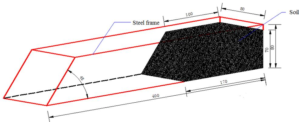
Fig. 1. Slope model (dimensions are in cm).
