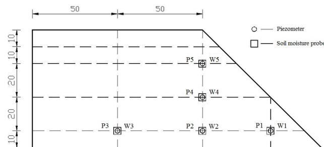
Fig. 4. Layout of piezometer and soil moisture probe in slope model (dimensions are in cm).
