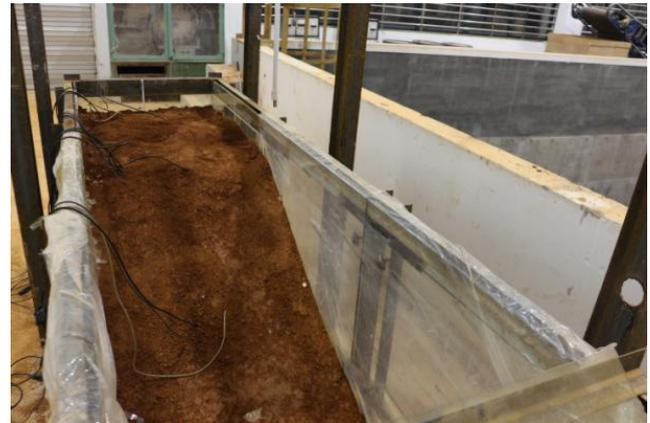
Fig. 2. Overview of the slope model after construction.
