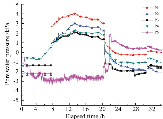
Fig. 6. Variation of the pore water pressure with elapsed time.
