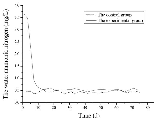
Fig. 5. Changes of ammonia nitrogen in A/O effluent.
