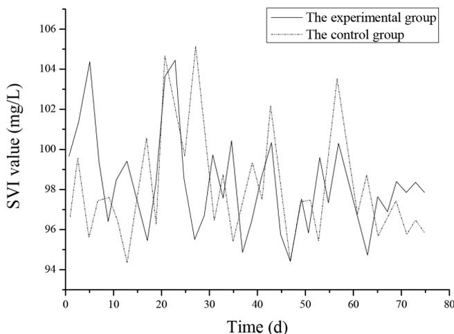
Fig. 8. Change of sludge settling performance in A/O system.
