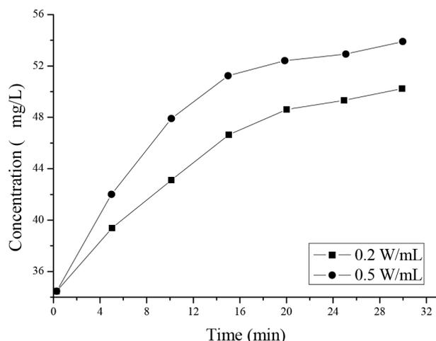
Fig. 2. Change of total nitrogen concentration of residual sludge in ultrasonic treatment.
