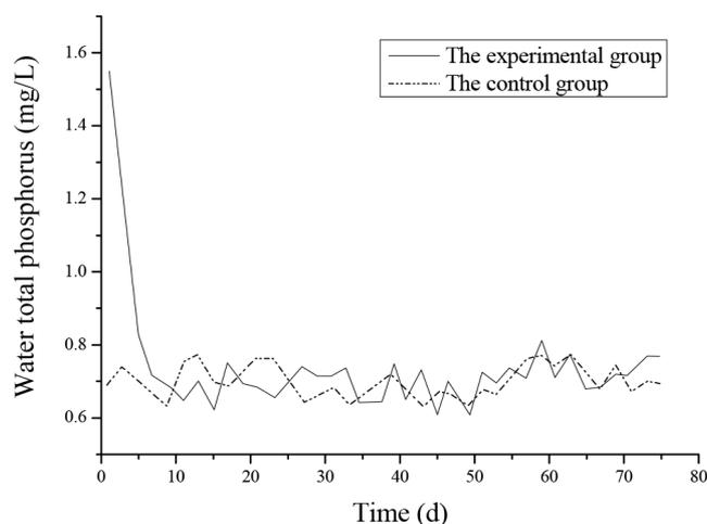
Fig. 7. Change of total phosphorus in A/O effluent.
