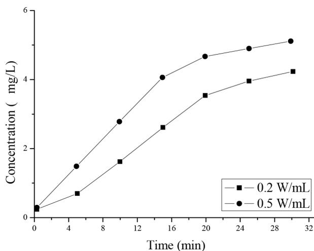
Fig. 3. Change of total phosphorus concentration of residual sludge in ultrasonic treatment.
