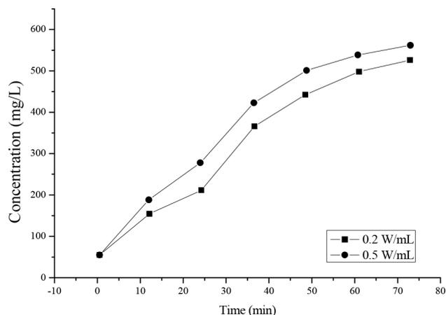
Fig. 1. Change of residual sludge SCOD in ultrasonic treatment.
