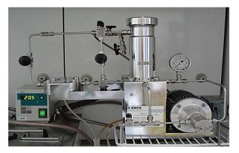
Fig. 1. KMS Cell CF1 laboratory-scale membrane filtration unit.
