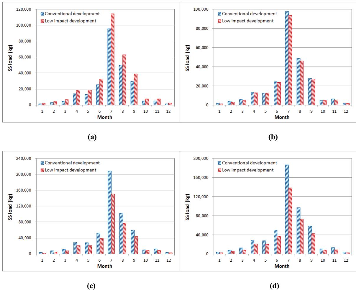
Fig. 6. Comparison of monthly SS pollutant load for the different development methods. (a) outfall ①, (b) outfall ②, (c) outfall ③, and (d) outfall ④.
