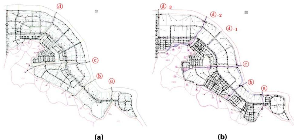
Fig. 3. SWMM compositions for the Songsan Green City. (a) Conventional development and (b) low impact development.
