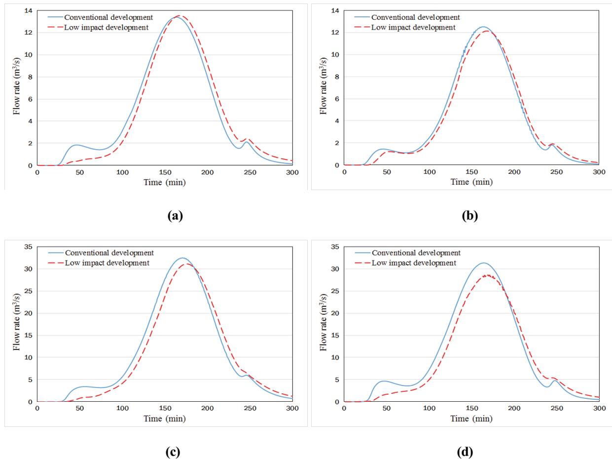
Fig. 4. Flood hydrographs for the different development methods. (a) Outfall (a), (b) outfall (b), (c) outfall (c), and (d) outfall (d).
