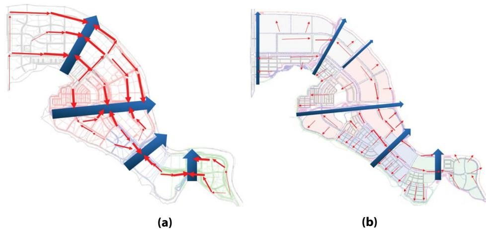
Fig. 2. Comparison of stormwater drainage systems. (a) Conventional development and (b) low impact development.
