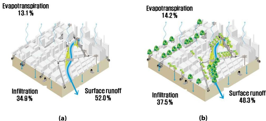
Fig. 5. Results of the hydrologic cycle analysis. (a) Conventional development and (b) Low impact development.
