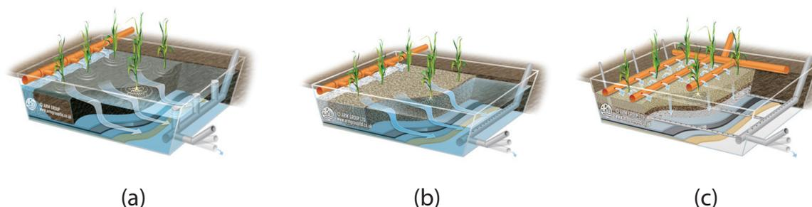
Fig. 1. (A) Free water surface constructed wetland. (B) Horizontal flow constructed wetland. (C) Vertical flow constructed wetland [1].
