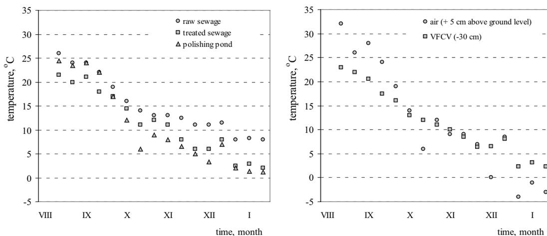
Fig. 4. Seasonal variability of temperature measured for influent, effluent and water in polishing pond as well as air temperature and thermic conditions 30 cm inside the filter bed.
