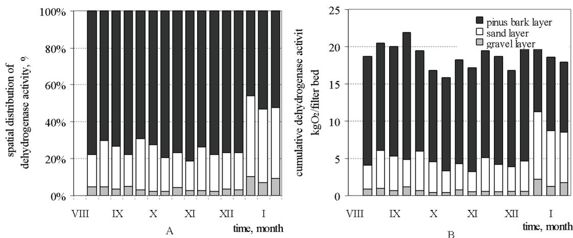
Fig. 8. Spatial contribution of dehydrogenase activity for different filtration layers (A) and cumulative dehydrogenase activity measured in filter bed (B).
