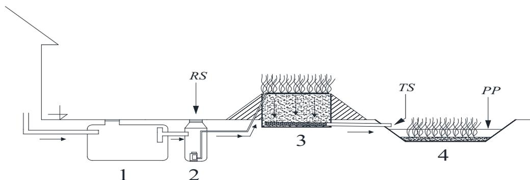
Fig. 2. Cross section of treatment system analyzed in the research ((1) – settler, (2) – pumping station, (3) – root filter, (4) – polishing pond, RS – raw sewage, TS – treated sewage, PP – sewage from polishing pond).
