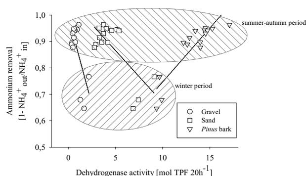
Fig. 9. Impact of dehydrogenase activity on the removal effectiveness of ammonium nitrogen.
