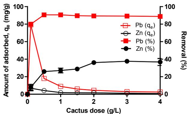
Fig. 1. Effect of dose on the  $\text{Pb}^{2+}$  and  $\text{Zn}^{2+}$  adsorption capacities and removal efficiencies of *Opuntia* adsorbent (Initial concentration: 10 mg/L; dose: 0.1–4.0 g/L; temperature: 25°C; pH: 4; contact time: 1,440 min).
