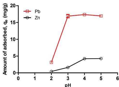
Fig. 6. Effect of initial solution pH on Pb<sup>2+</sup> and Zn<sup>2+</sup> adsorption capacities of *Opuntia* adsorbent (Dose: 0.5 g/L; initial concentration: 10 mg/L; temperature: 25°C; pH: 2–5; contact time: 1,440 min).
