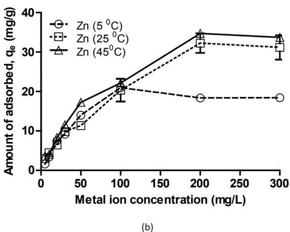
Fig. 8. Effect of temperature on (a)  $\text{Pb}^{2+}$  and (b)  $\text{Zn}^{2+}$  adsorption capacities of *Opuntia* adsorbent (Dose: 0.5 g/L; contact time: 1,440 min; temperature: 5, 25, or 45°C; pH: 4; initial concentration: 5–300 mg/L).
