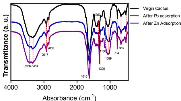
Fig. 2. FTIR spectra of virgin and used *Opuntia* adsorbents.
