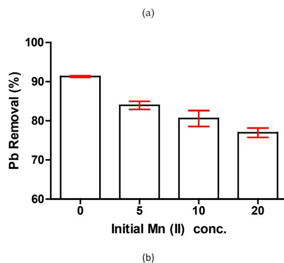
Fig. 9. Trends in  $\text{Pb}^{2+}$  removal efficiency by *Opuntia* adsorbent: removal with  $\text{Pb}^{2+}$  present as a single metal and in binary systems with (a)  $\text{Fe}^{2+}$  and (b)  $\text{Mn}^{2+}$  ions in increasing initial concentrations (Dose: 0.5 g/L; contact time: 1,440 min; temperature: 25°C; pH: 4; initial concentration: 0, 5, 10, 20 mg/L).
