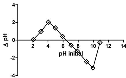
Fig. 7.  $\text{pH}_{\text{pzc}}$  plot for *Opuntia* adsorbent (Dose: 0.5 g/L; contact time: 1,440 min; temperature: 25°C; pH: 2–11; solvent: 0.01 mol/L NaCl solution).
