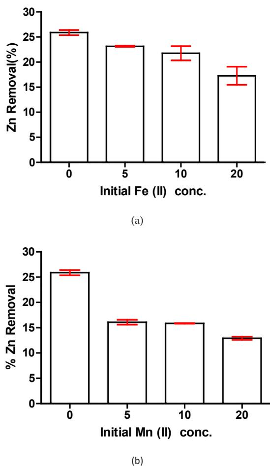
Fig. 10. Trends in Zn<sup>2+</sup> removal efficiency by *Opuntia* adsorbent: removal with Zn<sup>2+</sup> present as a single metal and in binary systems with (a) Fe<sup>2+</sup> and (b) Mn<sup>2+</sup> ions in increasing initial concentrations (Dose: 0.5 g/L; contact time: 1,440 min; temperature: 25°C; pH: 4; initial concentration: 0, 5, 10, 20 mg/L).
