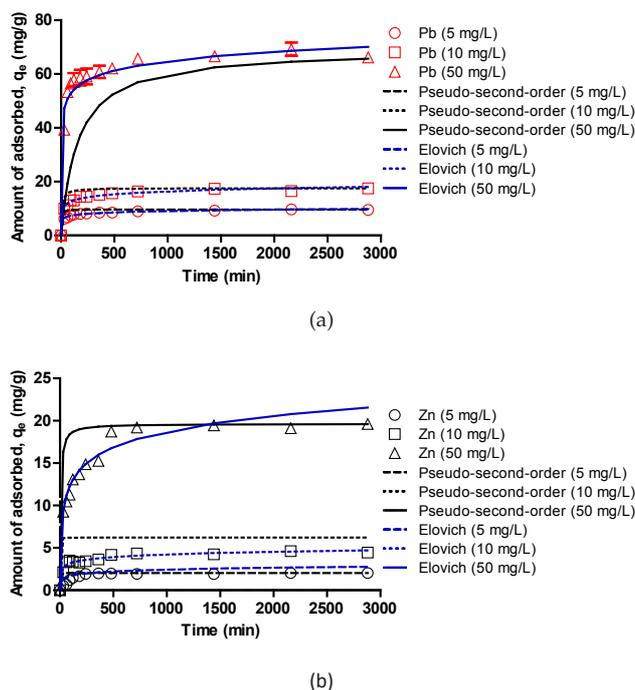
Fig. 4. Effect of contact time on the adsorption of (a)  $Pb^{2+}$  and (b)  $Zn^{2+}$  onto *Opuntia* adsorbent (Dose: 0.5 g/L; contact time: 30–2,880 min; temperature: 25°C; pH: 4; initial concentration: 5, 10, or 50 mg/L).
