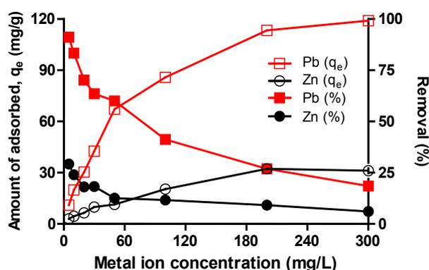
Fig. 5. Effect of initial ion concentration on the removal efficiency of (a)  $Pb^{2+}$  and (b)  $Zn^{2+}$  by *Opuntia* adsorbent (Dose: 0.5 g/L; initial concentration: 5–300 mg/L; temperature: 25°C; pH: 4; contact time: 1,440 min).
