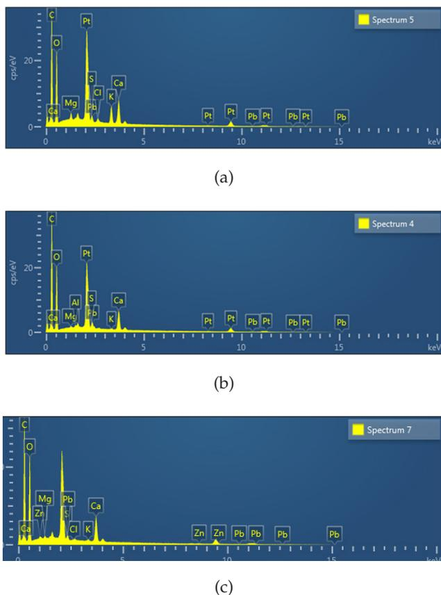
Fig. 3. EDS spectra of (a) virgin *Opuntia* adsorbent and (b, c) *Opuntia* adsorbents after adsorption of (b)  $Pb^{2+}$  and (c)  $Zn^{2+}$ .
