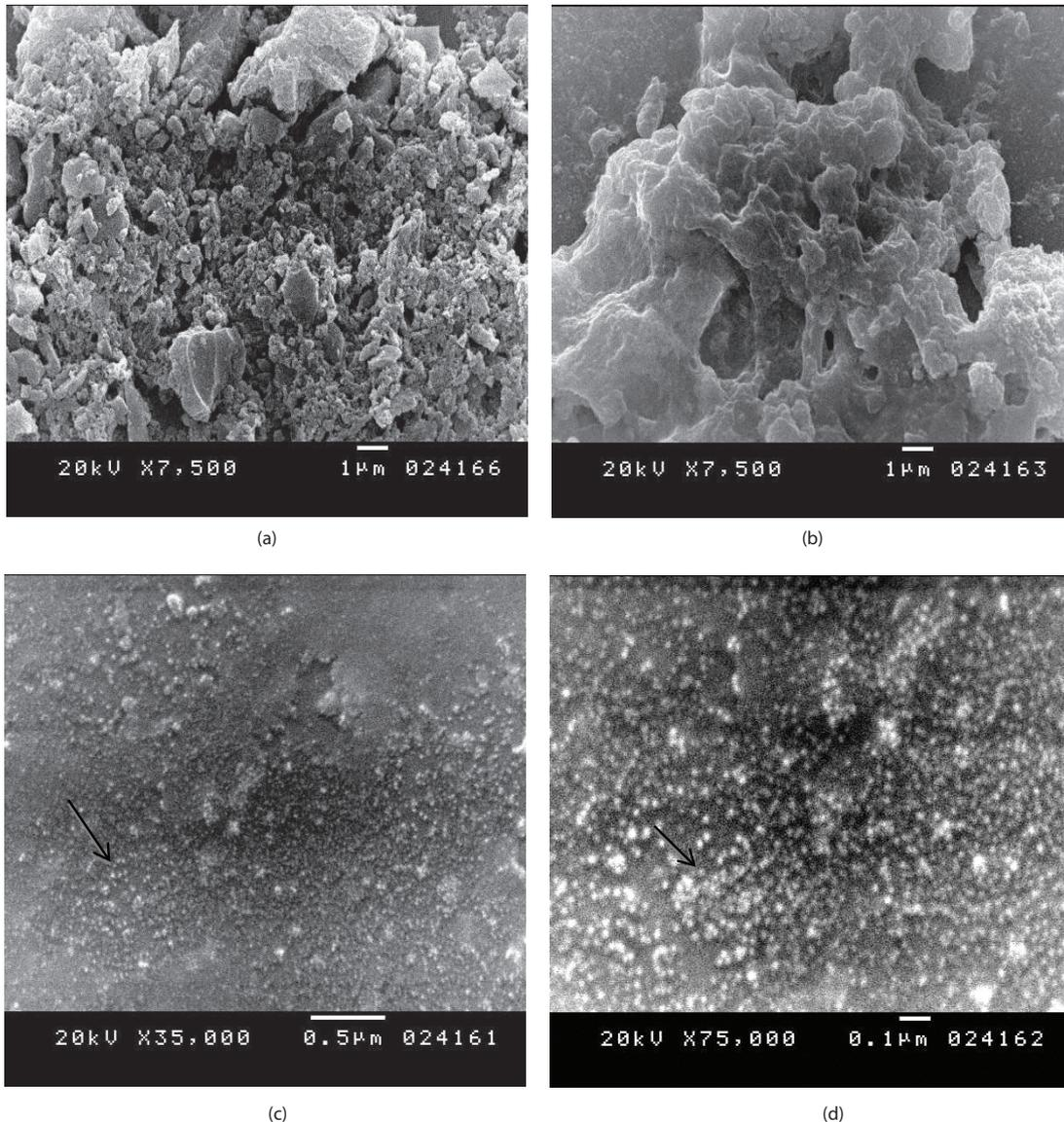
Fig. 4. SEM images of Ac only (a) and Au/Ac at different magnifications (b, c, d).
