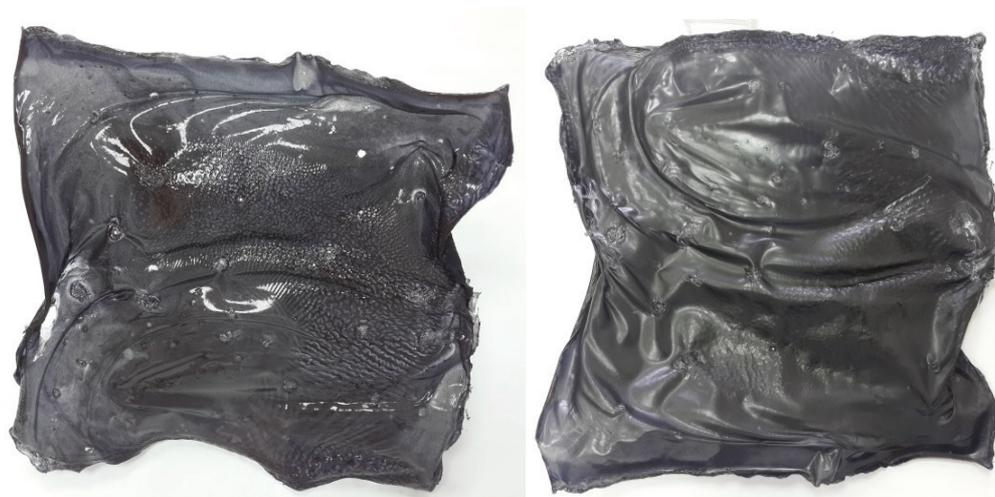
Fig. 6. Gold nanoparticles/Activated charcoal/Polyvinyl alcohol sheets.
