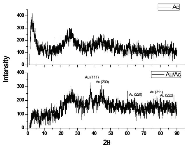
Fig. 5. XRD Bragg reflections of AuNPs adsorbed on Ac compared to Ac only.
