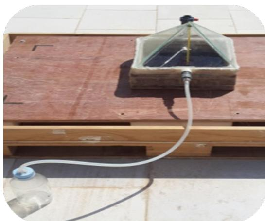
Fig. 1. A designed pyramid solar still.
