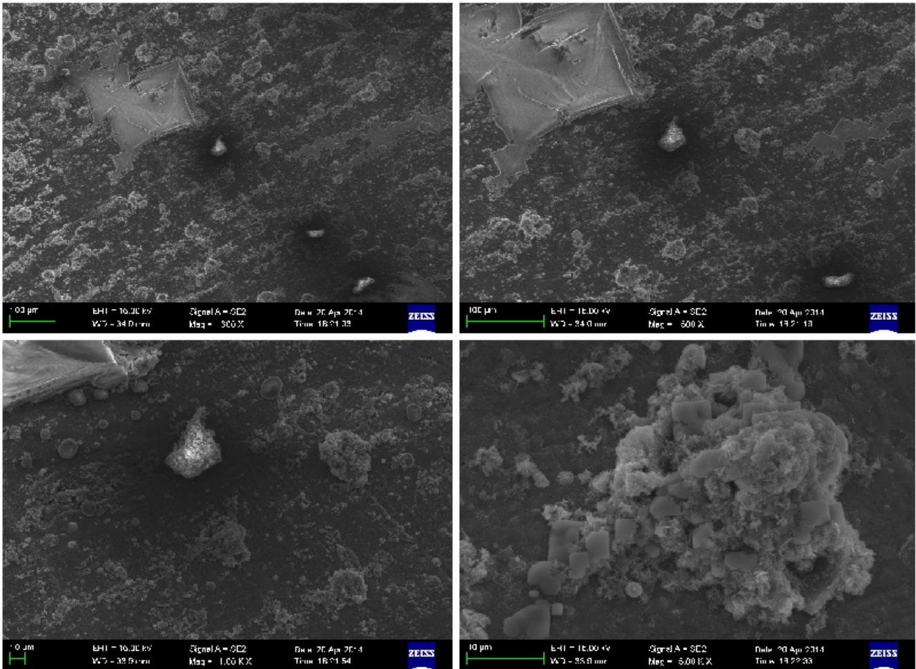
Fig. 8. The SEM images under the tube surface temperature of 70°C, the seawater concentration of 3.5%, and the spray density of 0.06 kg/(m•s), 10 h running.
