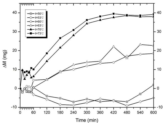
Fig. 3. The growing curves of scale under different tube surface temperatures with the spray density of 0.06 kg/(m•s) and the seawater concentration of 3.5%.
