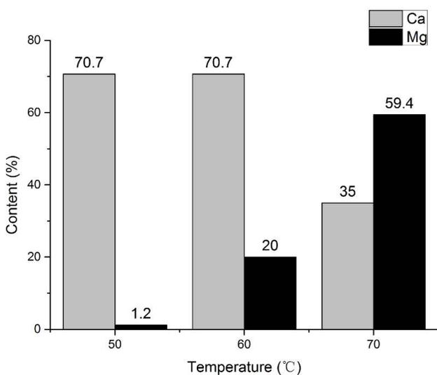
Fig. 9. The calcium and magnesium percentages in scale layer under the seawater concentration of 3.5%, the spray density of 0.06 kg/(m•s), and the tube surface temperatures of 50°C, 60°C and 70°C.
