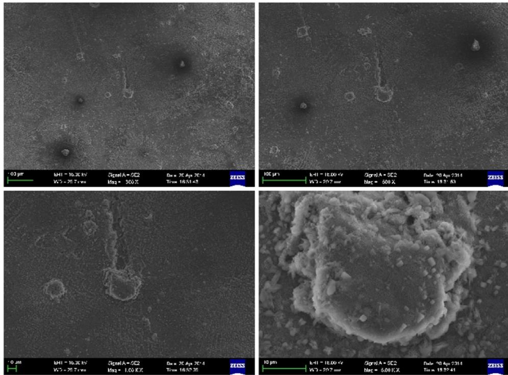
Fig. 6. The SEM images under the tube surface temperature of 50°C, the seawater concentration of 3.5%, and the spray density of 0.06 kg/(m<sup>2</sup>·s), 10 h running.
