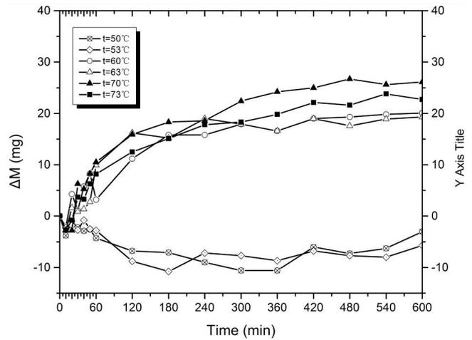
Fig. 4. The growing curves of scale under different tube surface temperatures with the spray density of 0.08 kg/(m•s) and the seawater concentration of 3.5%.
