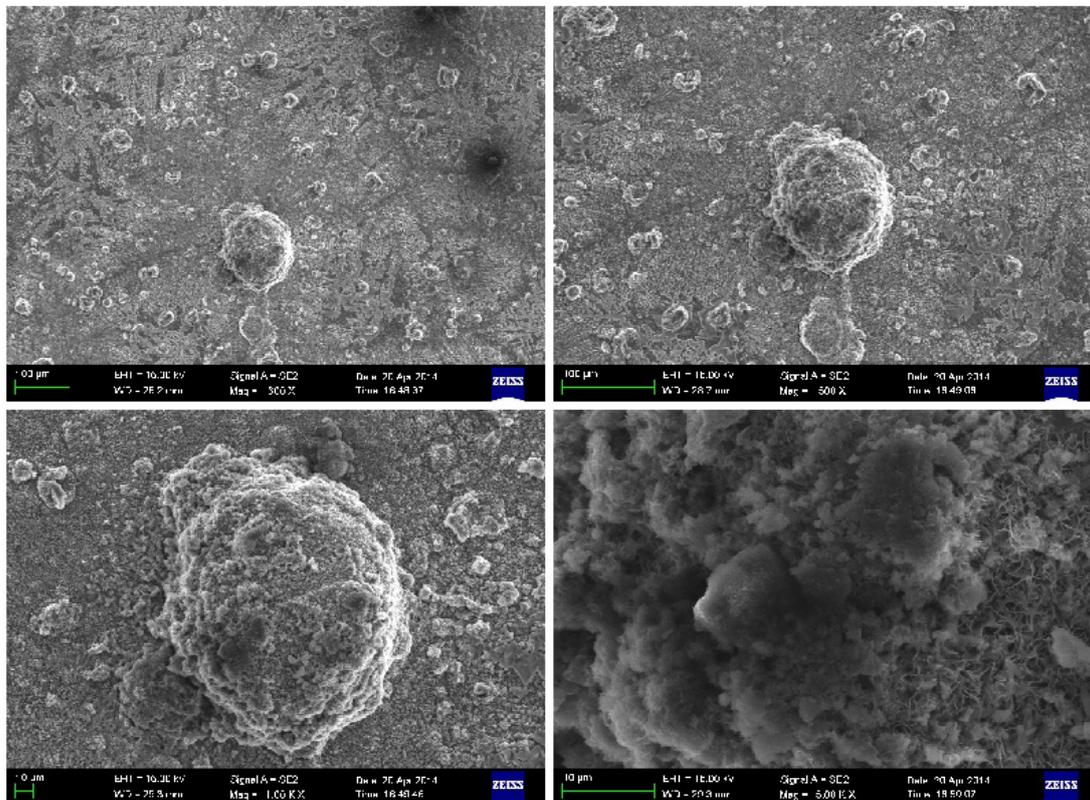
Fig. 7. The SEM images under the tube surface temperature of 60°C, the seawater concentration of 3.5%, and the spray density of 0.06 kg/(m<sup>2</sup>·s), 10 h running.
