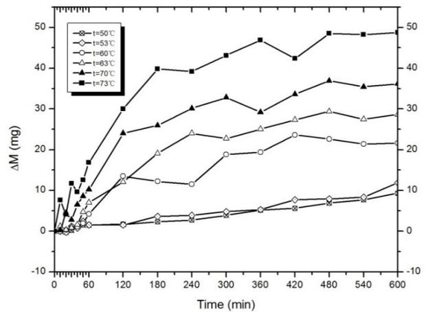
Fig. 5. The growing curves of scale under different tube surface temperatures with the spray density of 0.03 kg/(m•s) and the seawater concentration of 7%.
