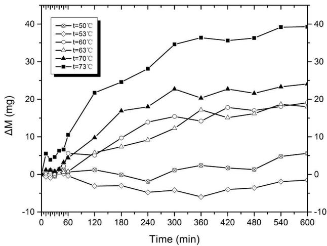
Fig. 2. The growing curves of scale under different tube surface temperatures with the spray density of 0.03 kg/(m•s) and the seawater concentration of 3.5%.
