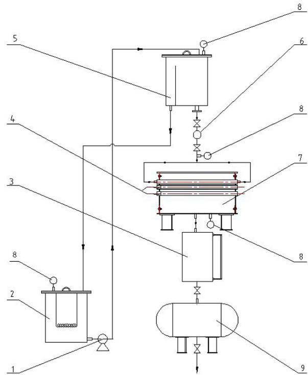
Fig. 1. Diagram of experimental system: 1, Pump; 2, heating tank; 3, measuring tank; 4, electrical heater; 5, upper tank; 6, flow meter; 7, evaporator; 8, thermocouples; and 9, storage tank.
