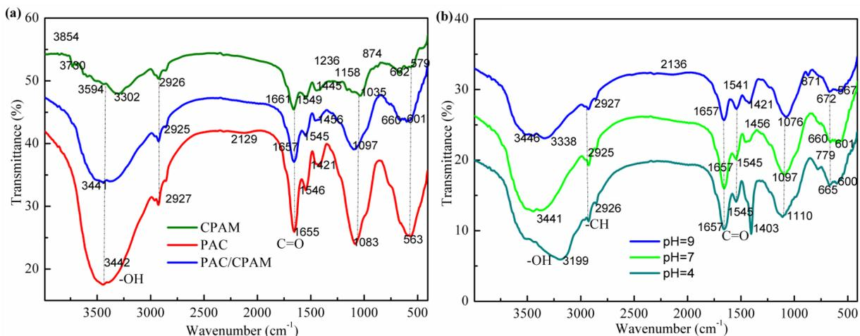
Fig. 6. The effect of (a) flocculants and (b) pH on FTIR spectra of flocs.
