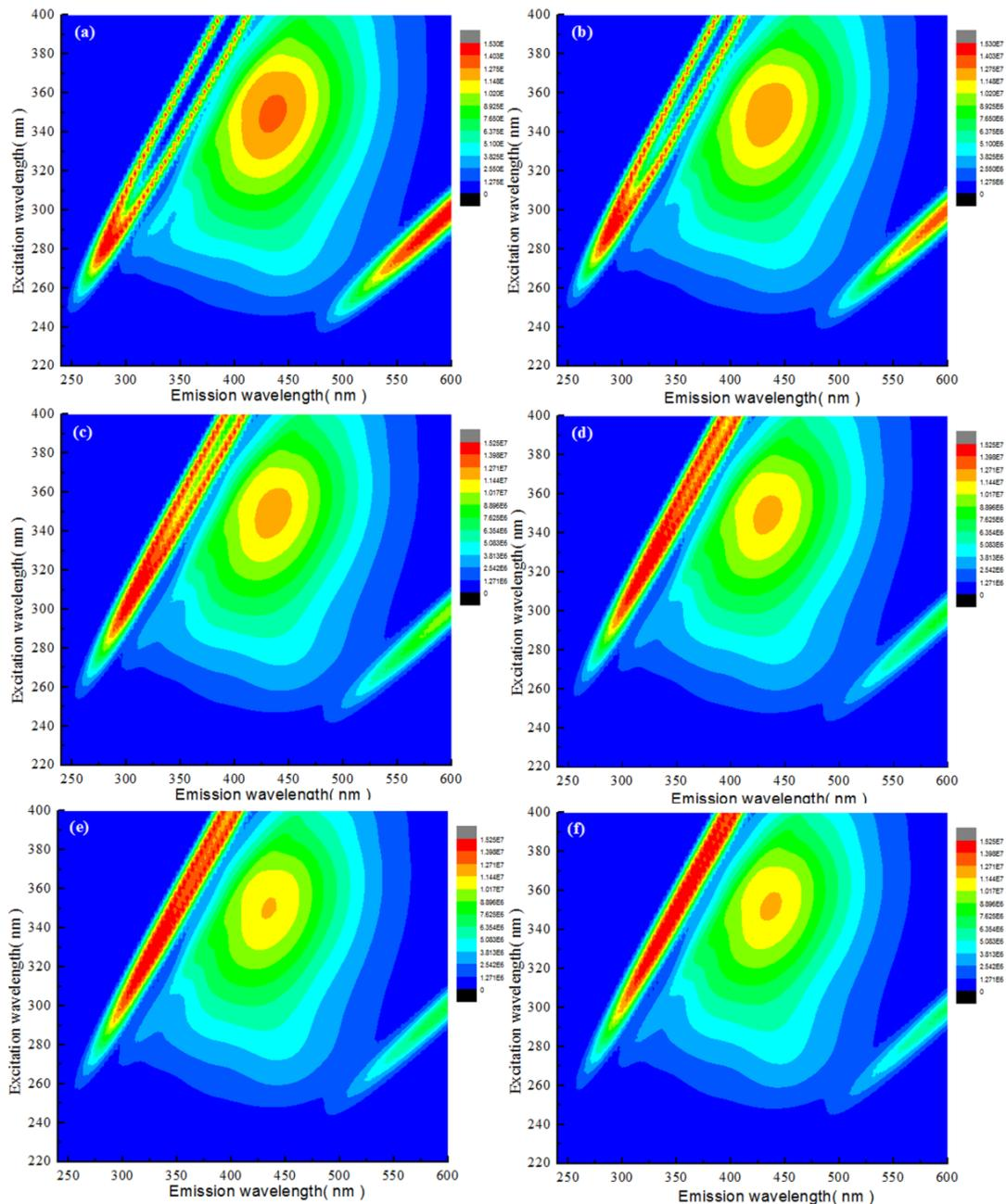
Fig. 8. The effect of PAC dosage on fluorescence spectra of supernatant after flocculation: (a) raw water, (b) 40 mg/L, (c) 60 mg/L, (d) 80 mg/L, (e) 100 mg/L, and (f) 120 mg/L.
