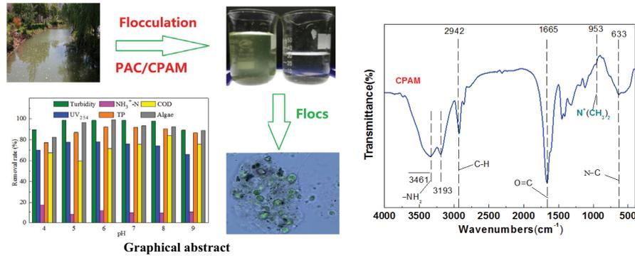
Fig. S1. FTIR spectrum of CPAM used in this study.
