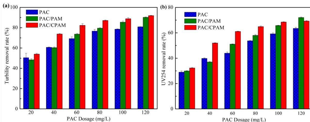
Fig. 1. The effect of flocculants on (a) turbidity removal rate and (b) UV<sub>254</sub> removal rate.
