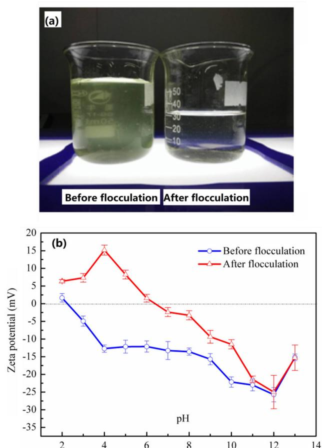
Fig. 9. comparison of (a) photograph and (b) zeta potential before and after flocculation.
