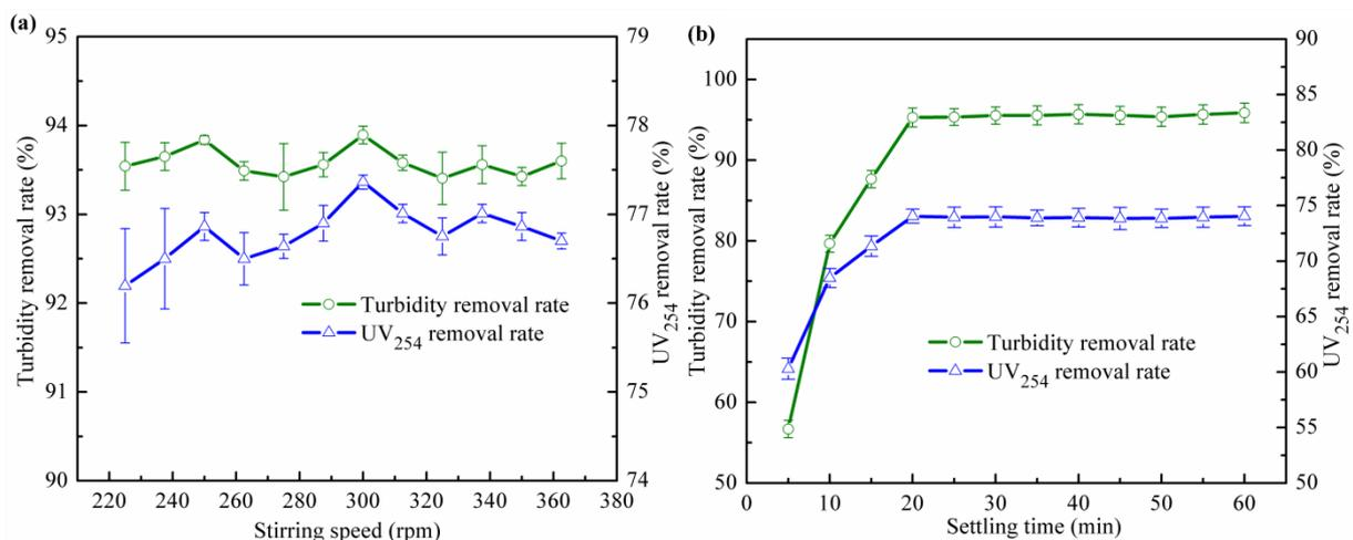
Fig. 3. The effect of (a) stirring speed and (b) settling time on turbidity removal rate and  $UV_{254}$  removal rate.
