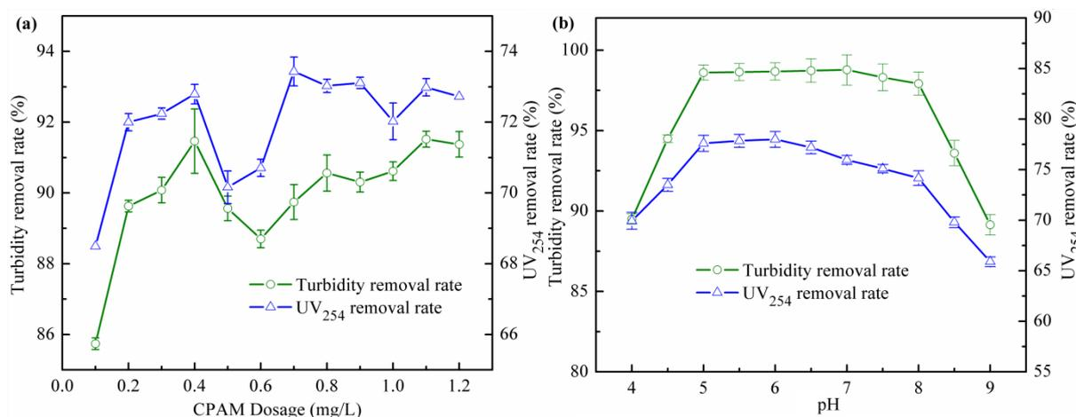
Fig. 2. The effect of (a) CPAM dosage and (b) pH on turbidity removal rate and UV<sub>254</sub> removal rate.
