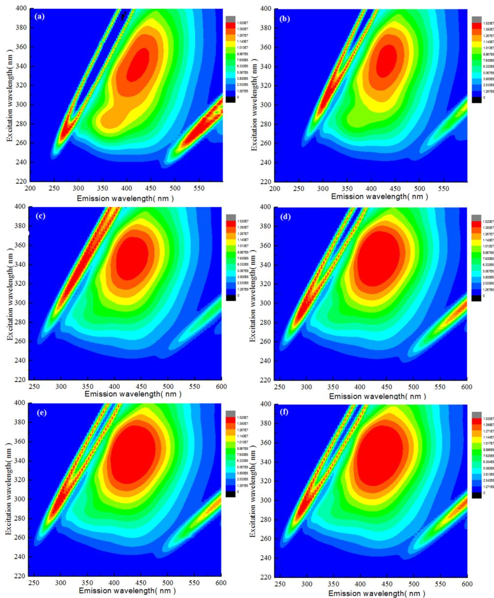
Fig. 7. The effect of pH on fluorescence spectra of supernatant after flocculation: (a) raw water, (b) pH=4, (c) pH=5, (d) pH=6, (e) pH=7, and (f) pH=8.
