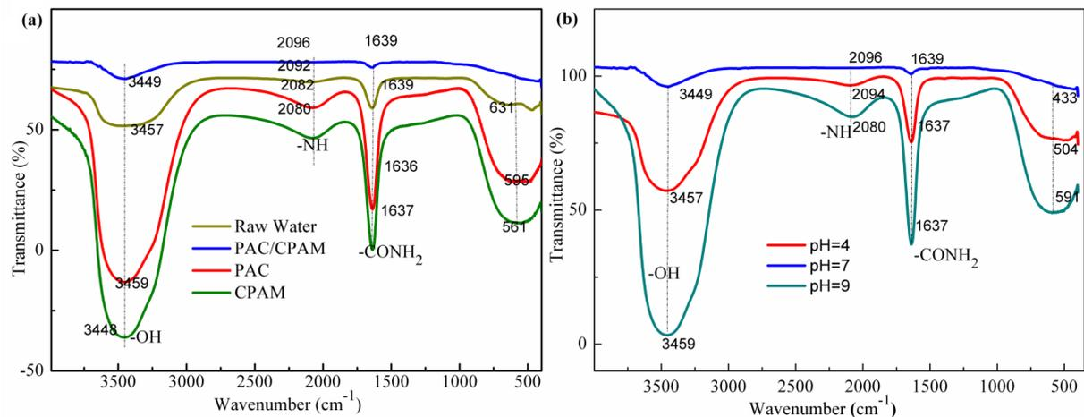
Fig. 5. The effect of (a) flocculants and (b) pH on FTIR spectra of supernatant.
