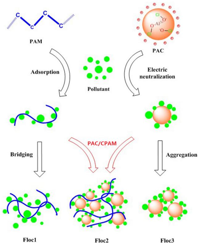
Fig. 11. Flocculation mechanism of CPAM, PAC, and PAC/CPAM.
