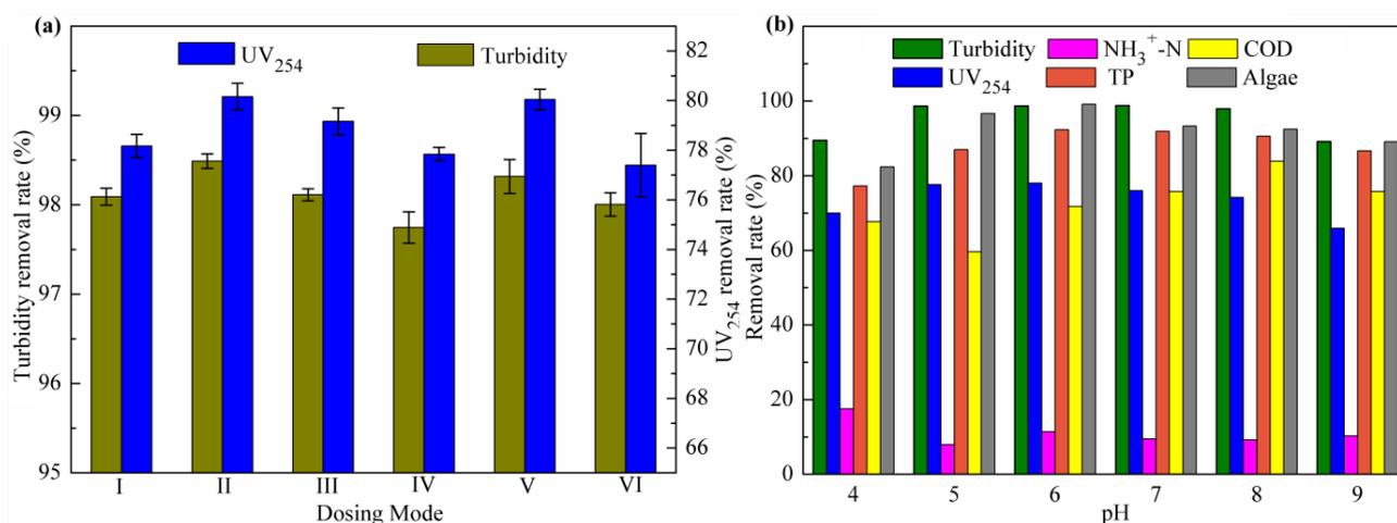
Fig. 4. The effect of (a) dosing mode on turbidity removal rate and  $UV_{254}$  removal rate and (b) removal rate of various water quality parameters.
