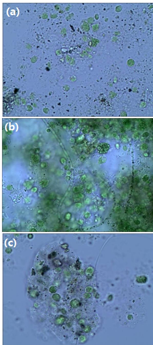
Fig. 10. The photograph of flocs at a magnification of  $\times 100$  by using flocculants of (a) PAC, (b) CPAM, and (c) PAC/CPAM.
