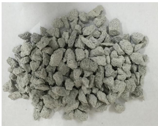
Fig. 1. Crushed autoclaved aerated concrete (CAAC).
