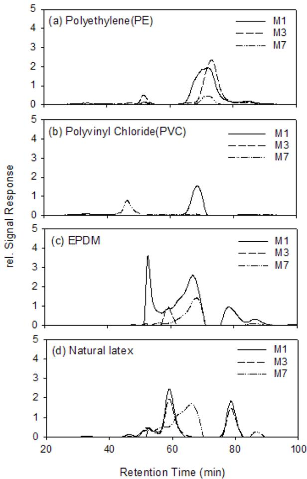
Fig. 4. SEC-DOC chromatograms of the target material for water from MP (migration potential) test.
