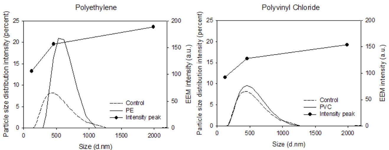
Fig. 5. Size distribution of retained water for 3 da (72 h) under MP (migration potential) test condition (60°C).
