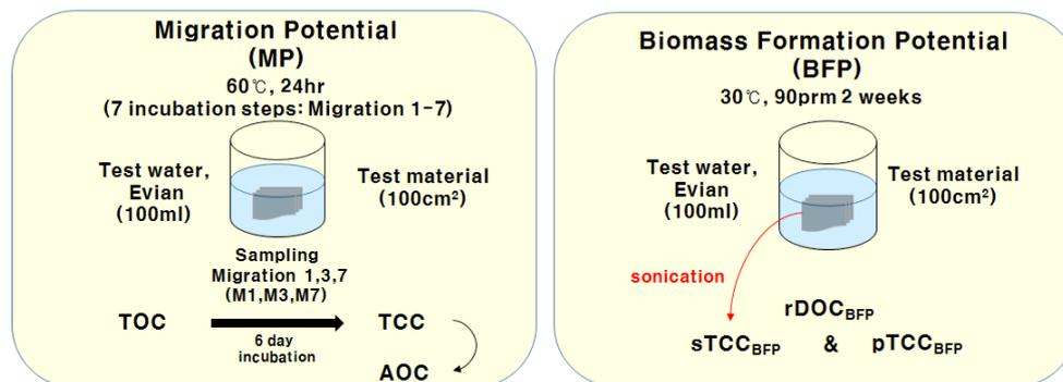
Fig. 1. Schematic overview of BioMig test method migration potential (MP) test and biomass formation potential (BFP) test.
