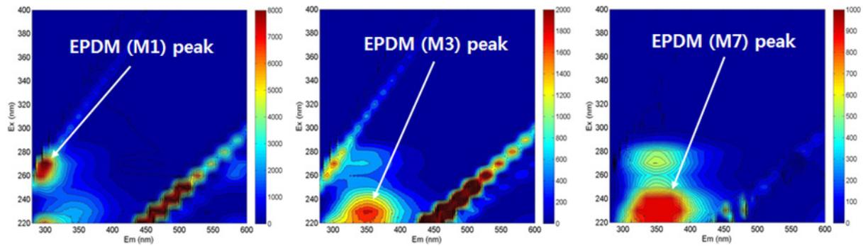
Fig. 6. EEM peak of the EPDM for water from MP (migration potential) test (M1, M3, M7).
