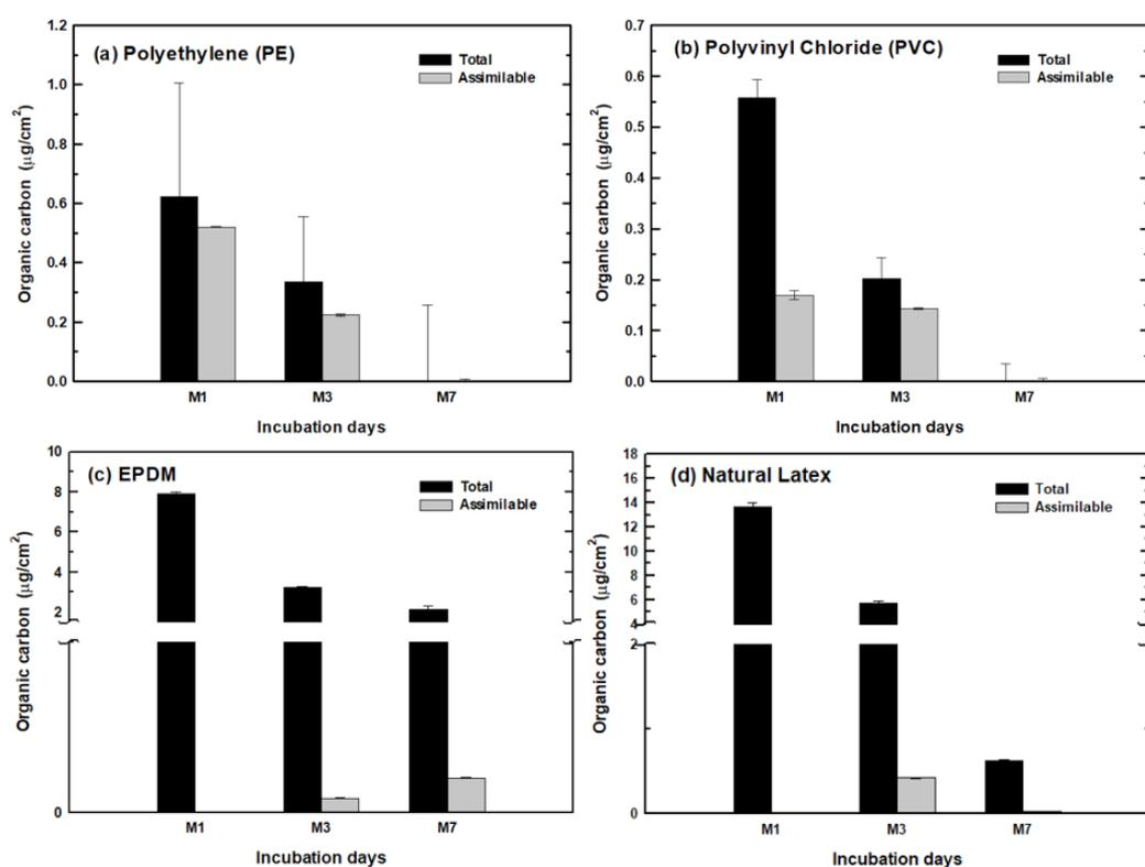
Fig. 2. MP test: total organic carbon (total) and assimilable organic carbon (assimilable) of quantified on result from incubation days (M1, M3, and M7).
