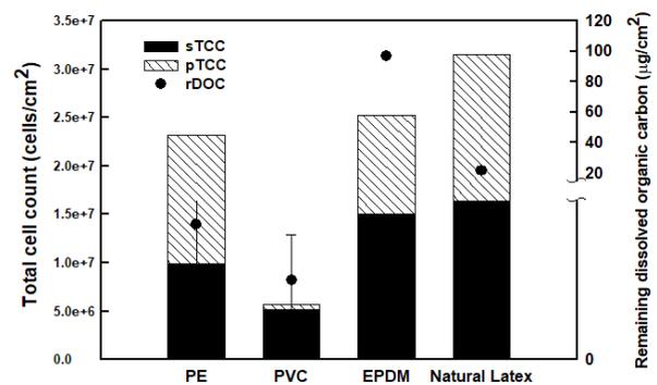
Fig. 7. BFP: the planktonic and sessile total cell count (pTCC and sTCC) and the remaining DOC (rDOC).
