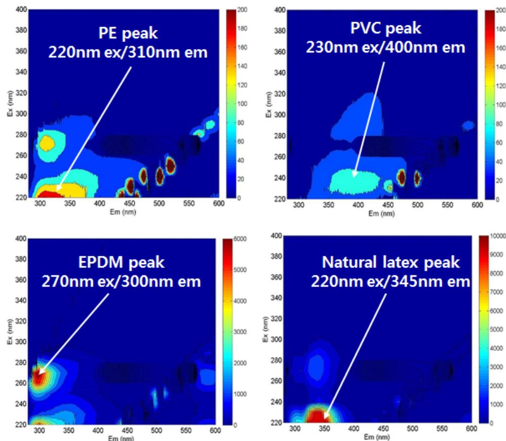
Fig. 3. EEM peak of the target material for water from M1 via migration potential.
