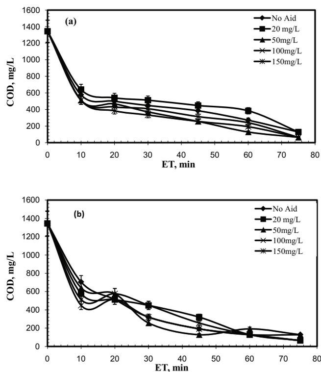
Fig. 2. COD degradation curves for varying dosage of coagulant aid PAA using Fe and Al electrodes for 6 V: (a) iron electrodes and (b) aluminum electrodes (COD<sub>0</sub>: 1,350 mg/L, pH: 6.85, number of electrodes: 4).
