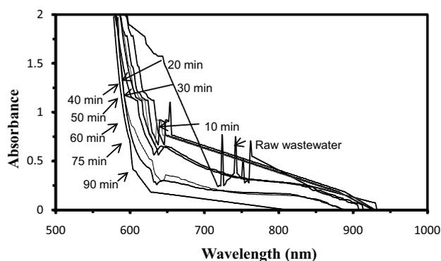
Fig. 8. UV-visible spectra before and after ECT of raw silk textile wastewater.
