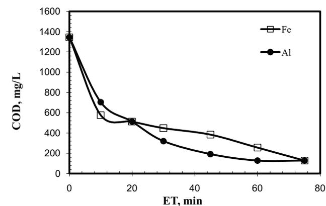
Fig. 3. Comparison of COD degradation curve for iron and aluminum electrodes for 6 V and four electrodes at a specific electrode area to volume (SEA/V): 24 m<sup>2</sup>/m<sup>3</sup> and COD<sub>0</sub>: 1,350 mg/L.
