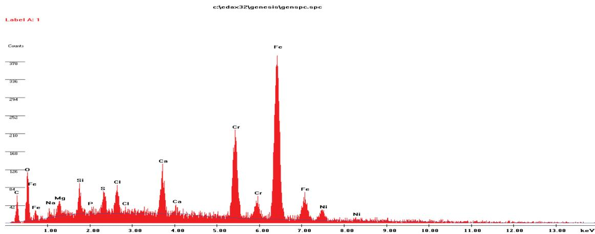
Fig. 9. Dry sludge composition after ECC using EDS for an applied cell voltage of 6 V.
