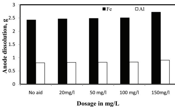
Fig. 5. Anode dissolution for iron and aluminum electrodes for 6 V and four electrodes at specific electrode area to volume (SEA/V): 24 m<sup>2</sup>/m<sup>3</sup> and COD<sub>0</sub>: 1,350 mg/L.
