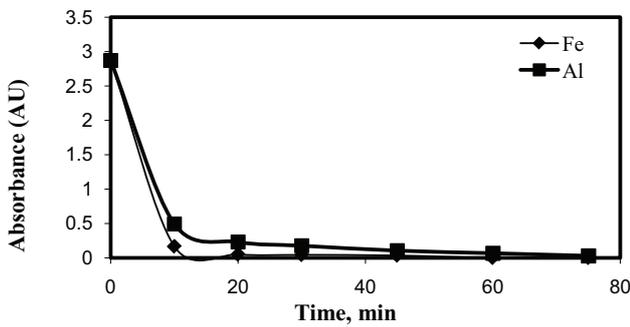
Fig. 4. Comparison of absorbance of iron and the aluminum electrodes for 6 V and four electrodes at specific electrode area to volume (SEA/V): 24 m<sup>2</sup>/m<sup>3</sup> and COD<sub>0</sub>: 1,350 mg/L.
