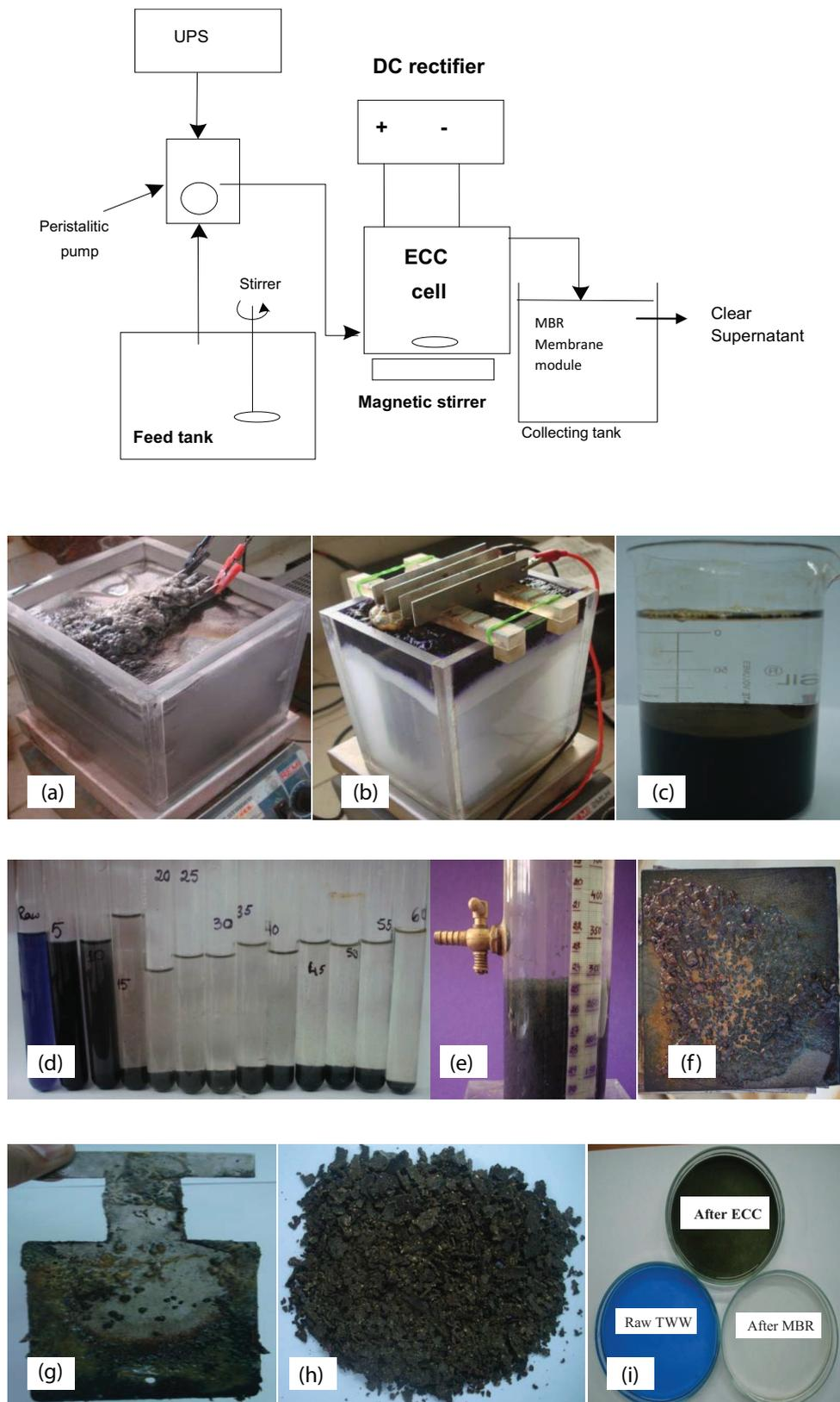
Fig. 1. Schematic of the experimental setup showing ECC + submerged MBR: (a) during ECC of TWW, (b) after ECC (see sludge flotation showing clear water reclaimable) (c) water reclamation after ECC, (d) samples retrieved during ECC of TWW, (e) post ECC slurry in settling column, (f) electrode condition after ECC, (g) flake deposits on anode plates just after ECC, (h) dry sludge after ECC, (i) raw TWW, after ECC, after MBR.
