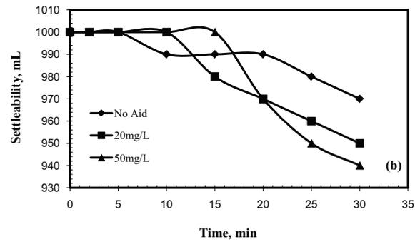
Fig. 6. Settleability of ECC slurry for varying dosage of PAA during batch ECC at optimal operating conditions of four electrodes and 6 V for Fe electrodes and Al electrodes: (a) settling curves for iron electrodes and (b) settling curves for aluminum electrodes.
