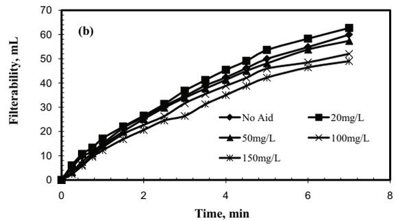
Fig. 7. Gravity filtration of post ECC slurry for varying PAA doses using Fe and Al electrodes at optimal operating conditions of four electrodes and 6 V: (a) filterability of post ECC slurry with iron electrodes and (b) filterability of post ECC slurry with aluminum electrodes.
