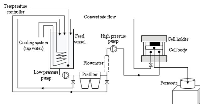
Fig. 2. Schematic flow diagram of the experimental setup.
