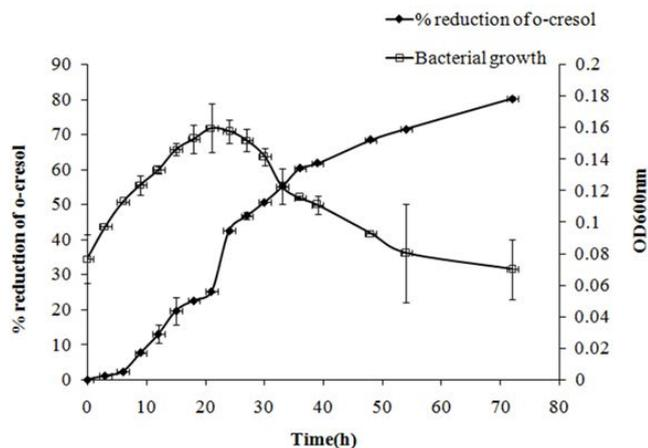
Fig. 3. Correlation between the growth of *P. fluorescens* NITDPY and its potential in degradation of 200 mg L<sup>-1</sup> of *o*-cresol in batch study at optimized condition.
