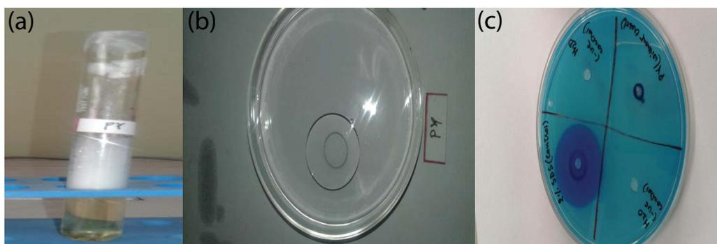
Fig. 5. Qualitative assays for biosurfactant from *P. fluorescens* NITDPY. (a) Foaming height assay, (b) Oil displacement test, (c) CTAB MB agar assay.
