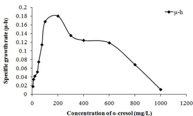
Fig. 2. Specific growth rate of *P. fluorescens* NITDPY in MSM supplemented with different initial concentrations of *o*-cresol (5–1,000 mg L<sup>-1</sup>) as sole source of carbon at 30°C, pH 7, with continuous agitation (120 rpm).
