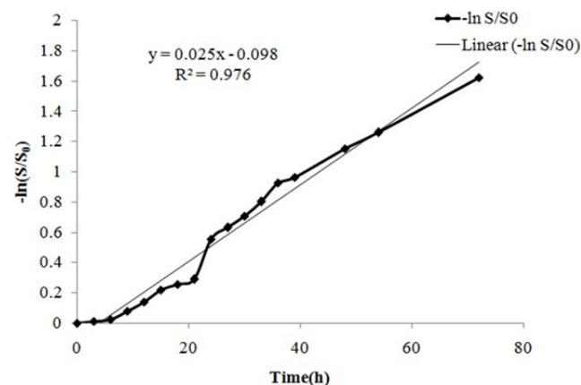
Fig. 4. Plot between time (h) versus  $-\ln(S/S_0)$  for determination of  $q$  at the initial *o*-cresol concentration of 200 mg L<sup>-1</sup>.
