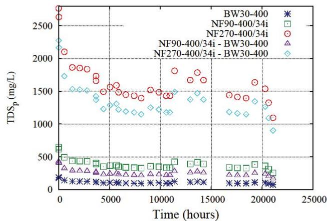
Fig. 14. TDS in the permeate for the different arrangements.
