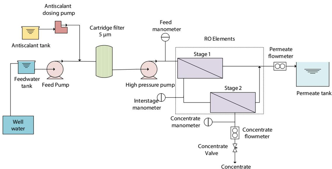
Fig. 1. Desalination plant flow diagram.
