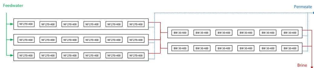
Fig. 13. Hybrid RO system with NF270-400/34i and BW30-400 membranes.
