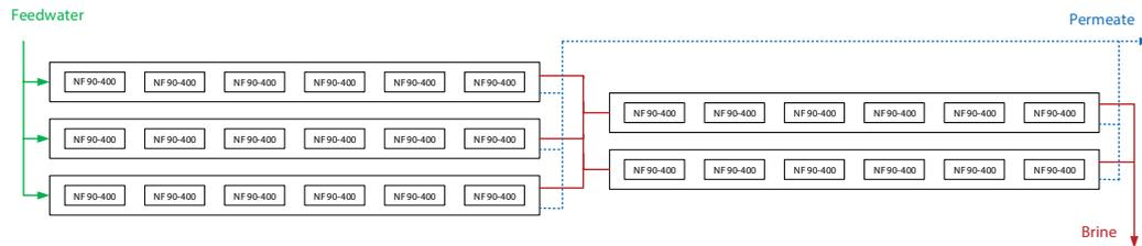
Fig. 10. RO system with NF90-400/34i membrane.
