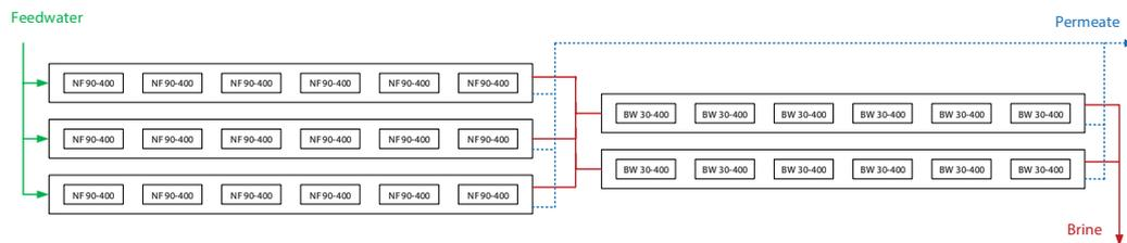
Fig. 12. Hybrid RO system with NF90-400/34i and BW30-400 membranes.
