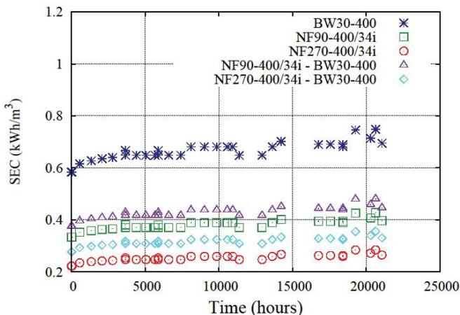
Fig. 15. SEC for the different arrangements.
