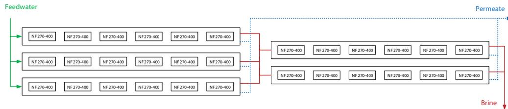
Fig. 11. RO system with NF270-400/34i membrane.
