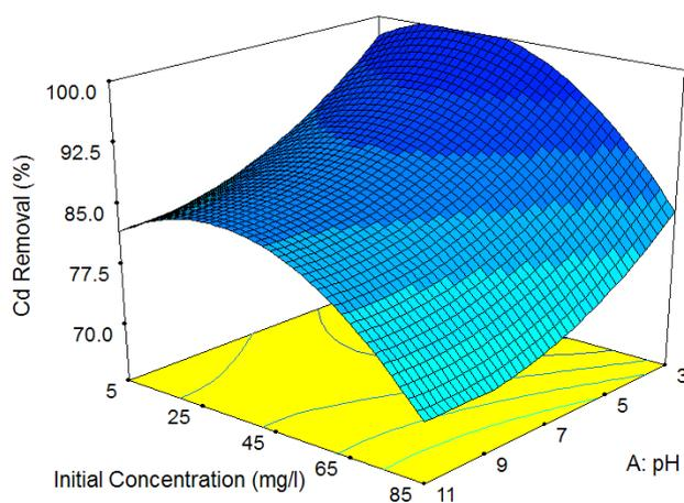
Fig. 3. Response surface plot showing the effect on Cd ions concentration and pH and their mutual effect on the metal uptake.
