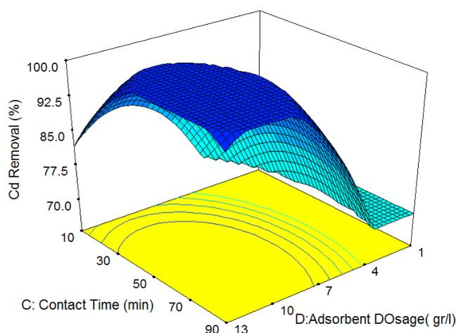
Fig. 4. 3D plot showing effect of adsorbent dose and contact time on percentage adsorption of Cd(II) ions.
