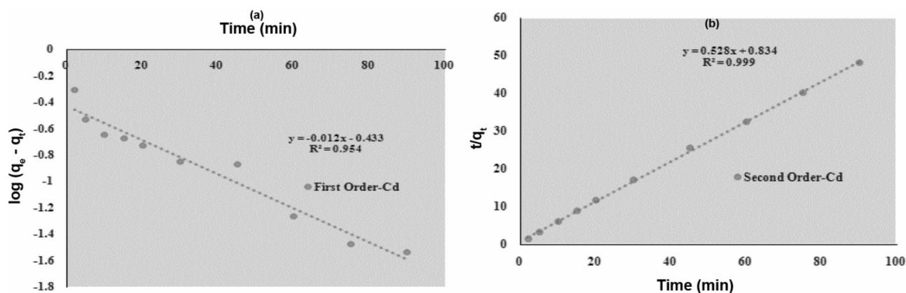
Fig. 7. Pseudo-first-order (a), and Pseudo-second-order (b) kinetic plot for the adsorption of Cd(II) Conditions.
