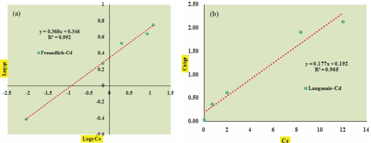
Fig. 6. Freundlich Isotherm (a) and Langmuir isotherm (b) for the adsorption of Cd onto prepared AC.
