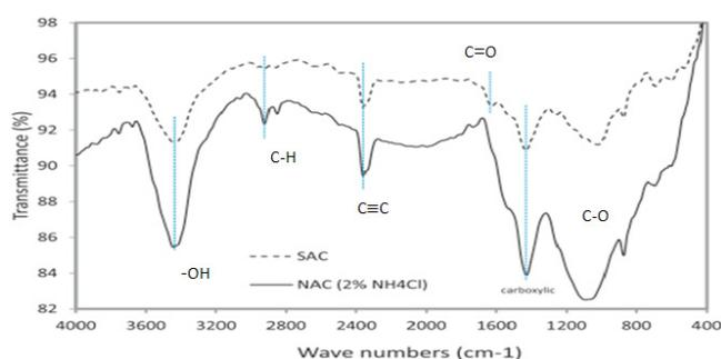
Fig. 1. FT-IR spectrum of India's shrub produced activated carbon (NAC or PAC) and standard activated carbon (SAC).
