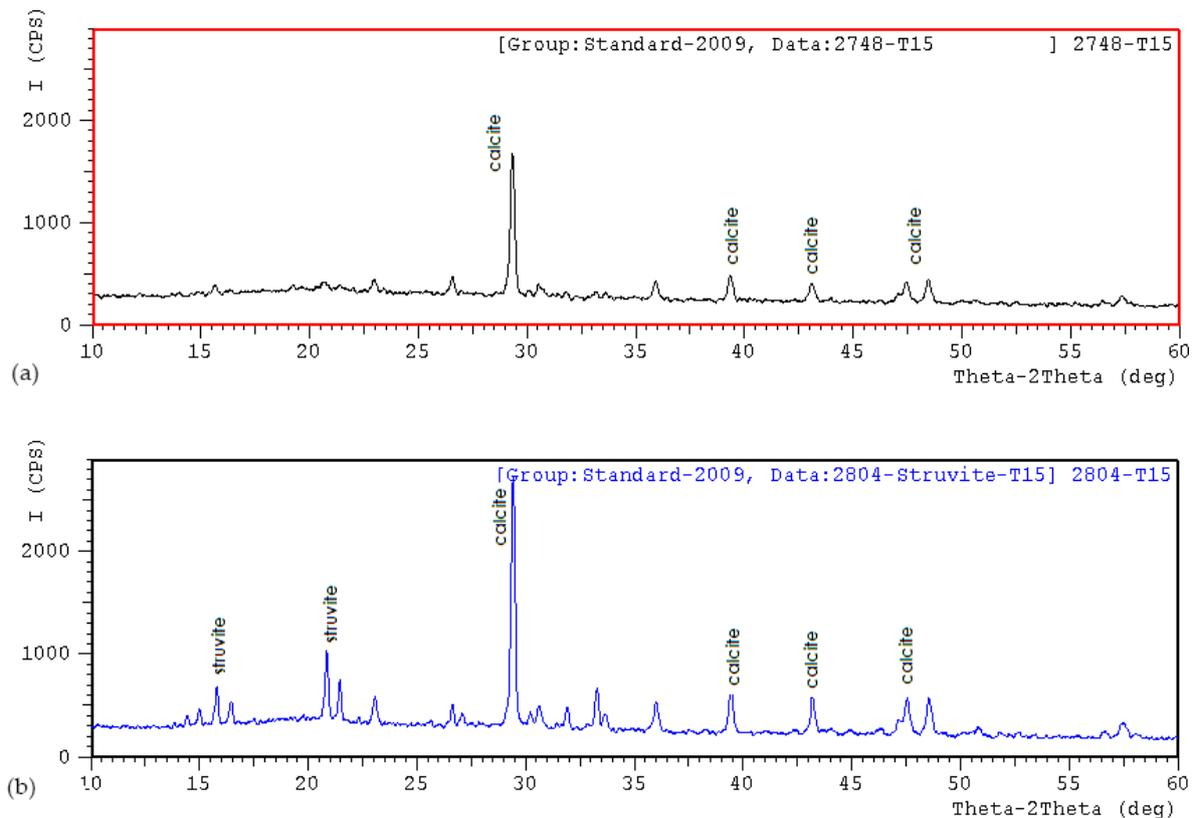
Fig. 9. XRD analyses for (a) raw sludge supernatant liquor before starting struvite crystallization experiment, and (b) settled solids after finishing struvite crystallization experiment.
