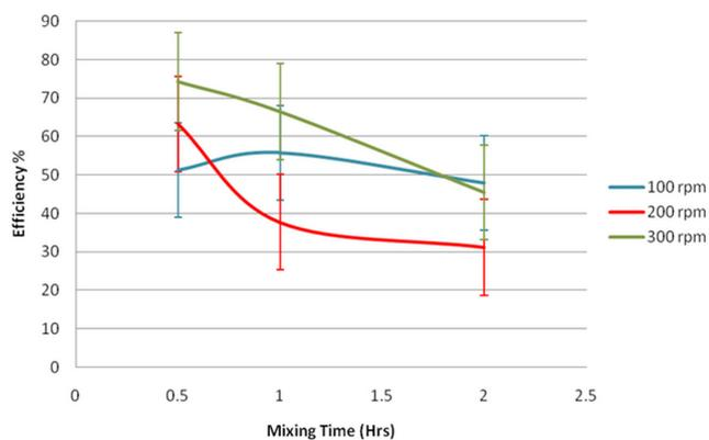
Fig. 3. Efficiency of  $\text{PO}_4$  removal at variable mixing time, variable mixing speed and 8 h settling time.
