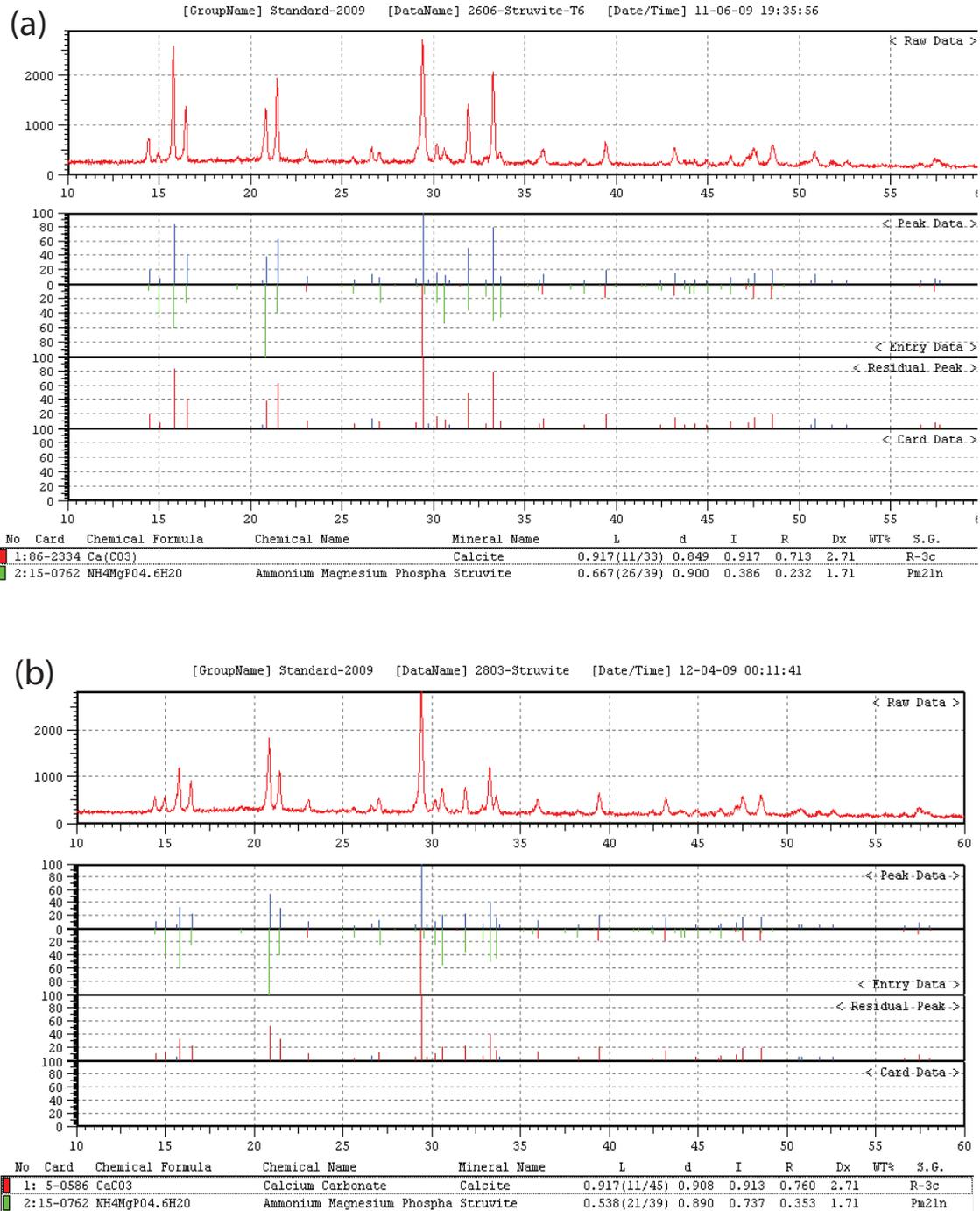
Fig. 8. XRD analyses showing the presence of struvite and calcite only in the tested sample for (a) 1.0 h mixing time, 300 rpm, 8 h settling time, and (b) 1.0 h mixing time, 300 rpm and 24 h settling time.
