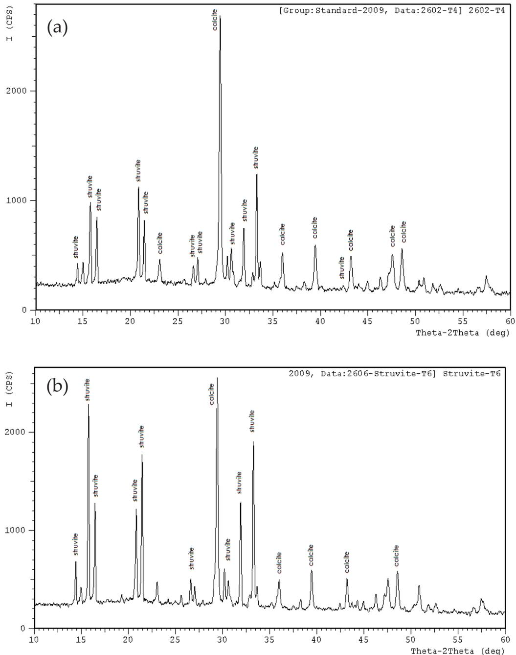
Fig. 7. XRD graph struvite formation at (a) 1.0 h mixing time, 100 rpm, 8 settling time, (b) 1.0 h mixing time, 300 rpm, 8 settling time.
