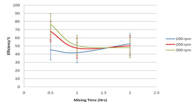
Fig. 4. Efficiency of  $\text{PO}_4$  removal at variable mixing time, variable mixing speed and 16 h settling time.
