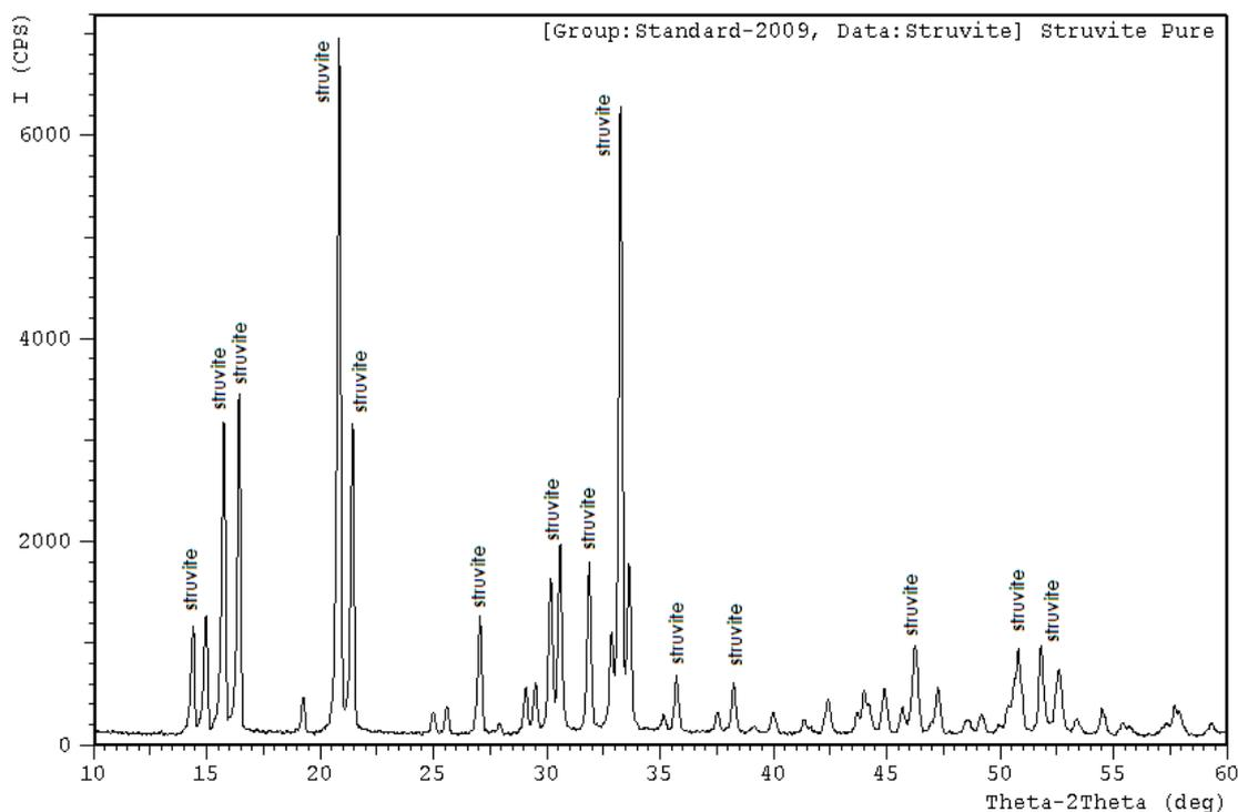
Fig. 6. XRD graph for pure struvite sample collected from Al Samra WWTP.
