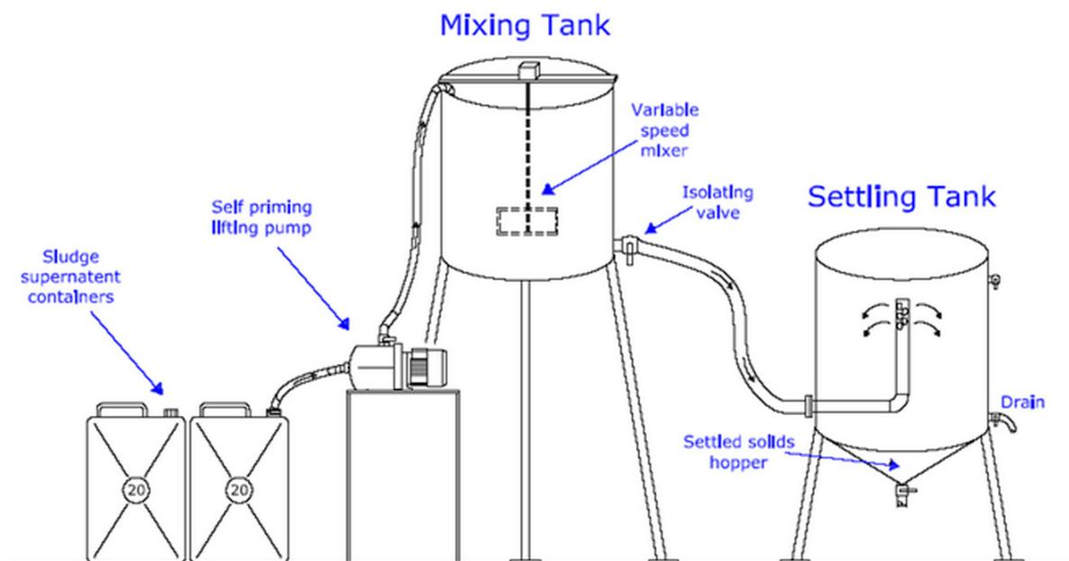
Fig. 1. Struvite precipitation pilot-scale reactor main components.
