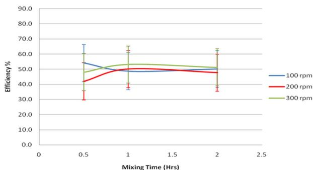
Fig. 5. Efficiency of  $\text{PO}_4$  removal at variable mixing time, variable mixing speed and 24 h settling time.
