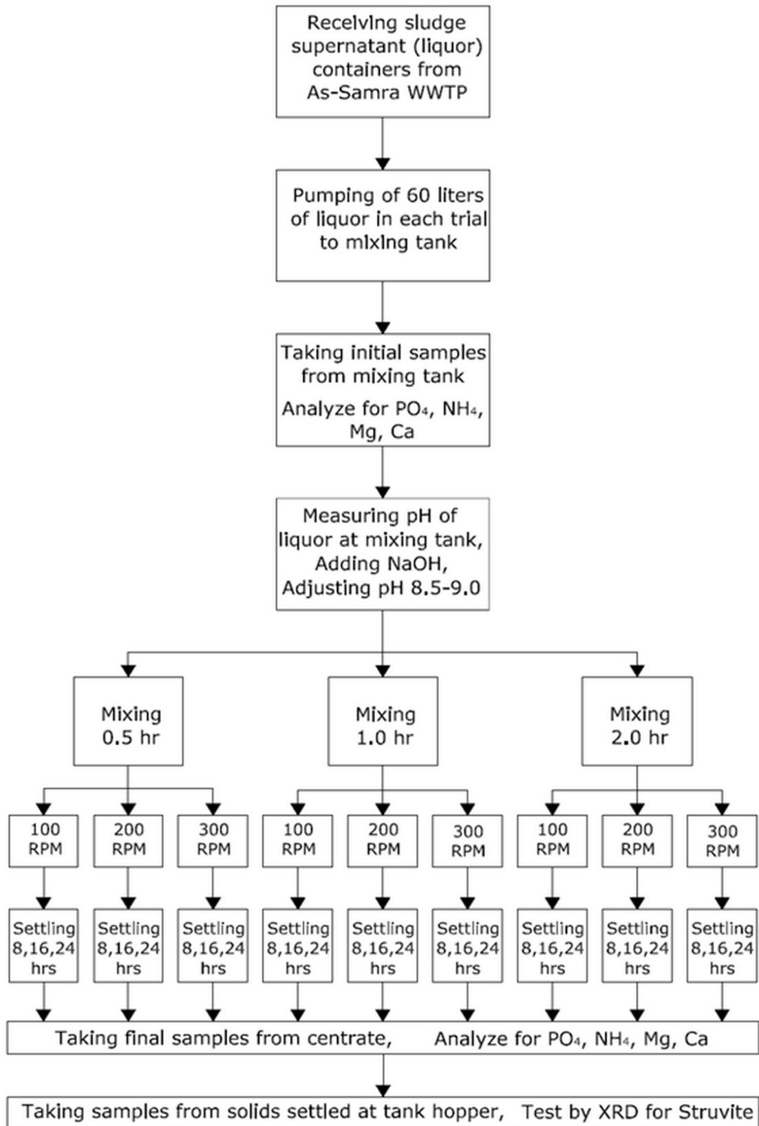
Fig. 2. Struvite precipitation experiment flow chart.
