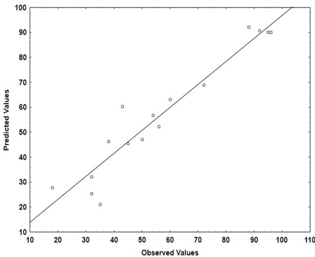
Fig. 6. Observed and predicted values for COD removal.
