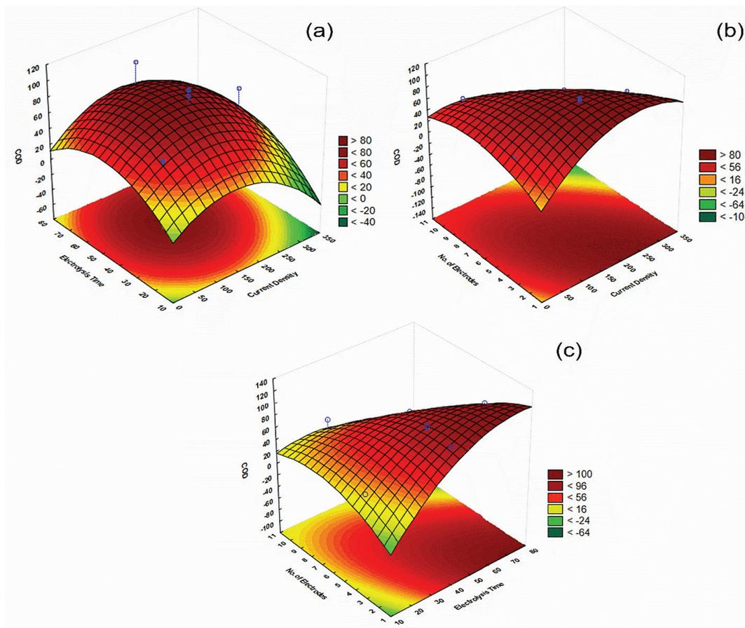
Fig. 3. Optimization of color removal with ECC.
