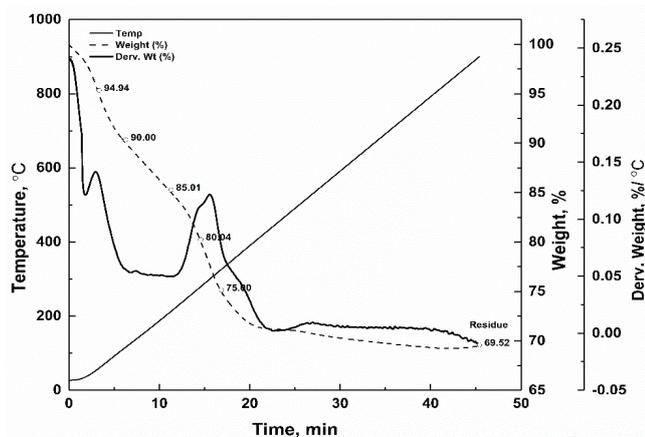
Fig. 10. Thermogravimetric analysis (TGA) and derivative thermogravimetric analysis (DTG) curves for 4 SS post ECC sludge.
