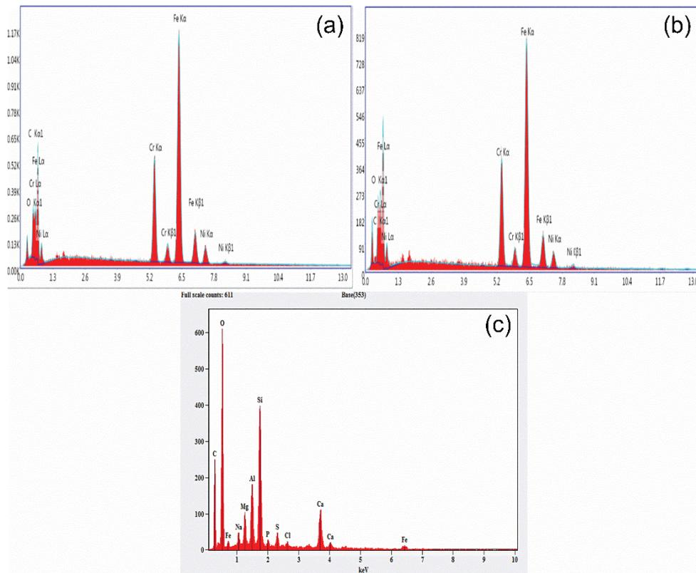
Fig. 9. EDX images of electrodes and post ECC solid sludge residues of 4 SS electrodes. (a) EDX images of SS electrode before use in ECC, (b) EDX of same SS electrode after 20 runs and (c) EDX of 4 SS electrode post ECC sludge.
