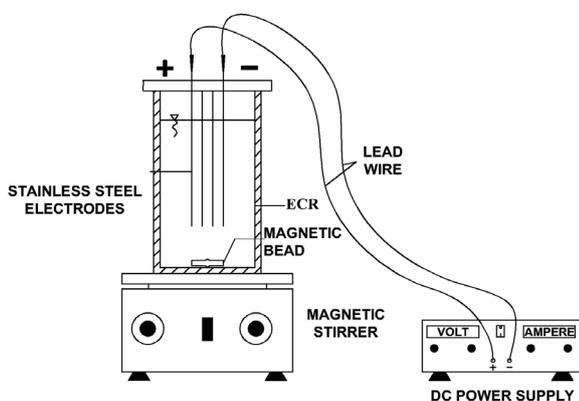
Fig. 1. Bipolar electrode arrangements using stainless steel (SS) electrodes.
