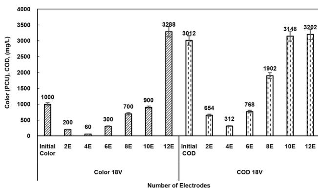
Fig. 2. Color and COD removals for different electrode numbers using SS plate electrodes. Operating conditions: ECR: 1.5 L; electrode arrangements: bipolar; color<sub>0</sub>: 1,000 PCU; COD<sub>0</sub>: 3,012 mg L<sup>-1</sup>; ET: 75 min; agitation speed: 400 rpm; CD: 180 A/m<sup>2</sup>.
