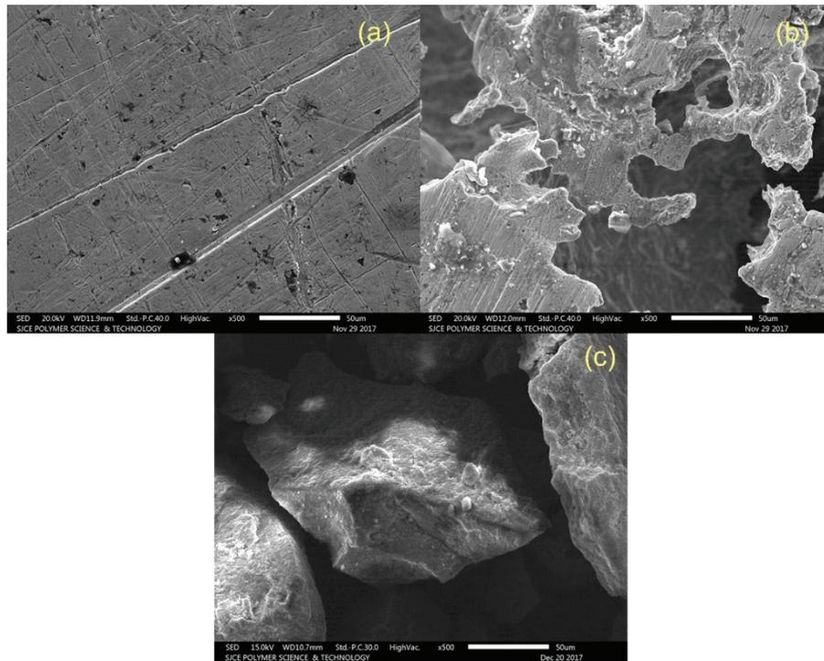
Fig. 8. SEM images of electrode and post ECC solid sludge residues of 4 SS electrodes. (a) SS electrode before use of ECC, (b) large dents after 20 runs of ECC and (c) 4 SS post ECC sludge.
