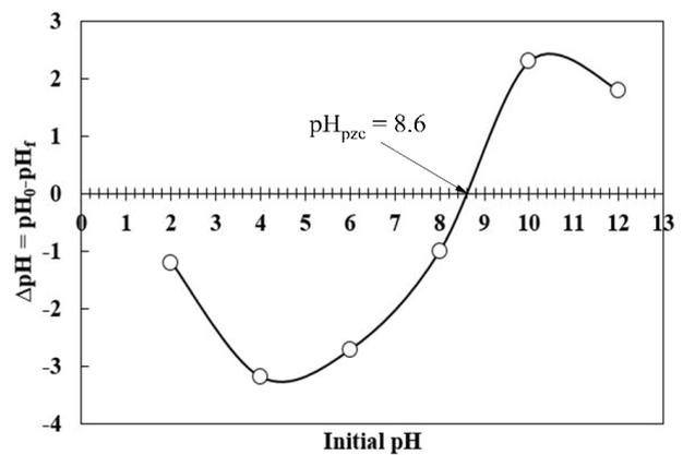
Fig. 7. Point of zero charge ( $pH_{pzc}$ ) of ECC generated sludge using 4 SS electrodes.
