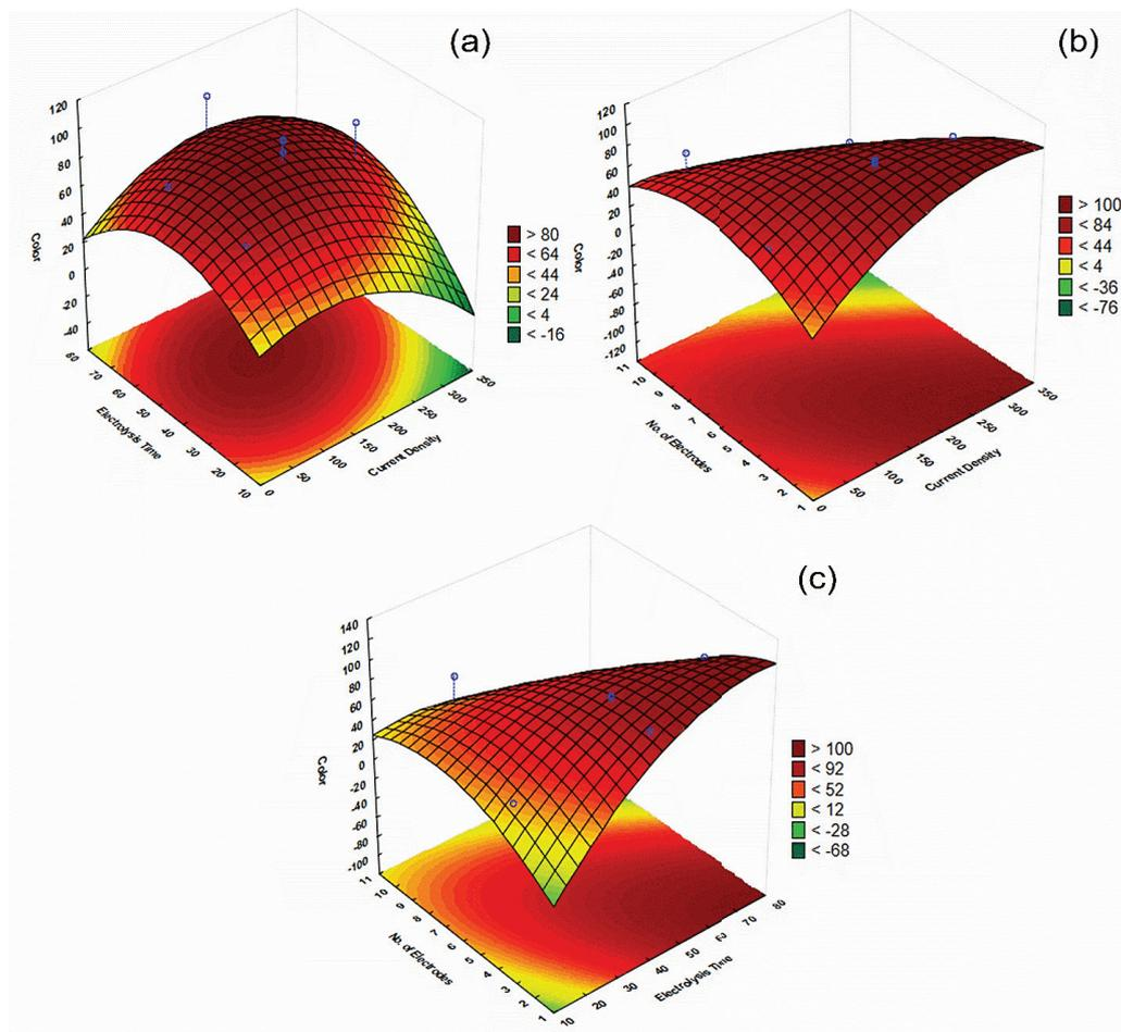
Fig. 5. Optimization of COD removal with BECC.
