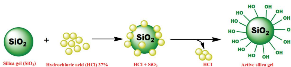
Fig. 1. Activation of silica gel surface.
