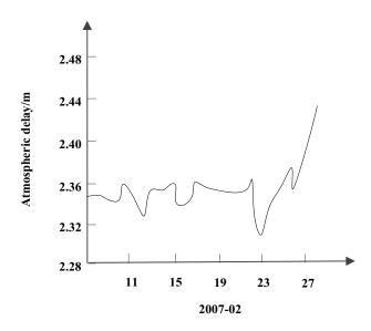
Fig. 2. Total zenith tropospheric delay at INSAR station in February 2007.
