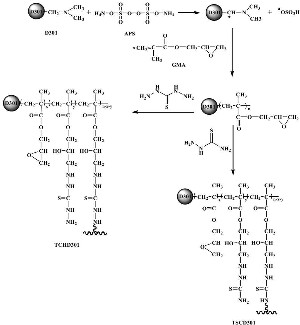
Fig. 1. Preparation process of TSCD301 and TCHD301.
