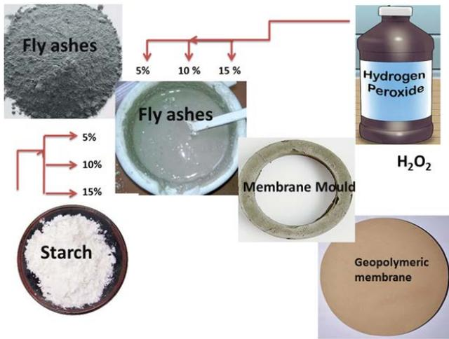
Fig. 2. Synthesis and additives addition for porosity of geopolymeric membrane.
