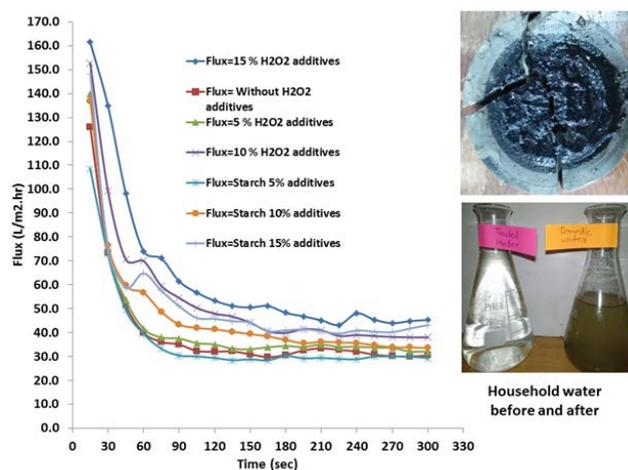
Fig. 6. Household wastewater treatment through inorganic geopolymeric membrane.
