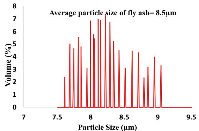
Fig. 3. Uniform particle size distribution of fly ashes.
