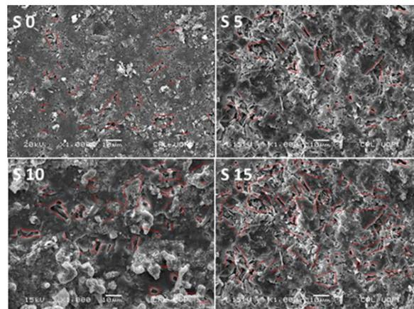
Fig. 5. SEM images of inorganic geopolymeric membrane: (S 0) without starch additives, (S 5) with 5% starch additives, (S 10) with 10% starch additives (S 15) with 15% starch additives.
