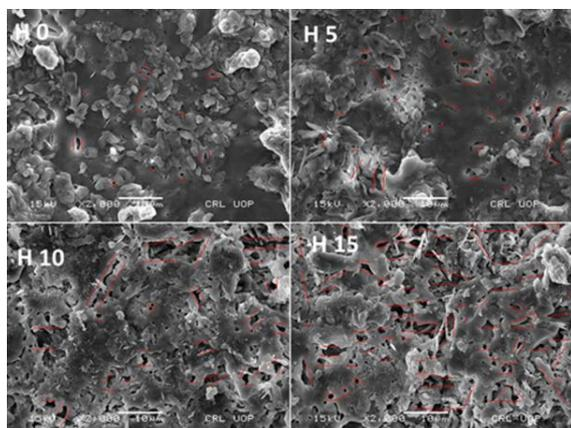
Fig. 4. SEM of inorganic geopolymeric membrane: (H 0) without additive, (H 5) with 5%  $\text{H}_2\text{O}_2$  additive, (H 10) with 10%  $\text{H}_2\text{O}_2$  additive (H 15) with 15%  $\text{H}_2\text{O}_2$  additive.
