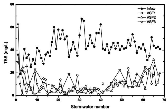
Fig. 2. Comparison of the TSS concentrations in the influent and effluent.
