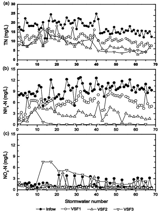
Fig. 5. Comparison of the TN,  $\text{NH}_4\text{-N}$  and  $\text{NO}_3\text{-N}$  concentrations in the influent and effluent (a) TN; (b)  $\text{NH}_4\text{-N}$ ; (c)  $\text{NO}_3\text{-N}$ .
