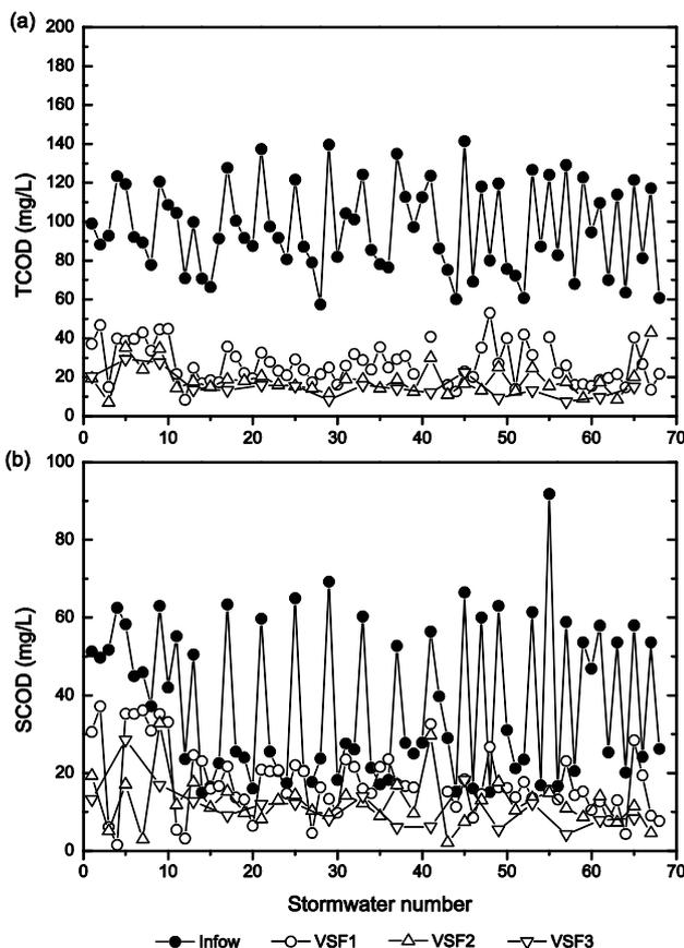
Fig. 3. Comparison of the COD concentrations in the influent and effluent (a) TCOD; (b) SCOD.
