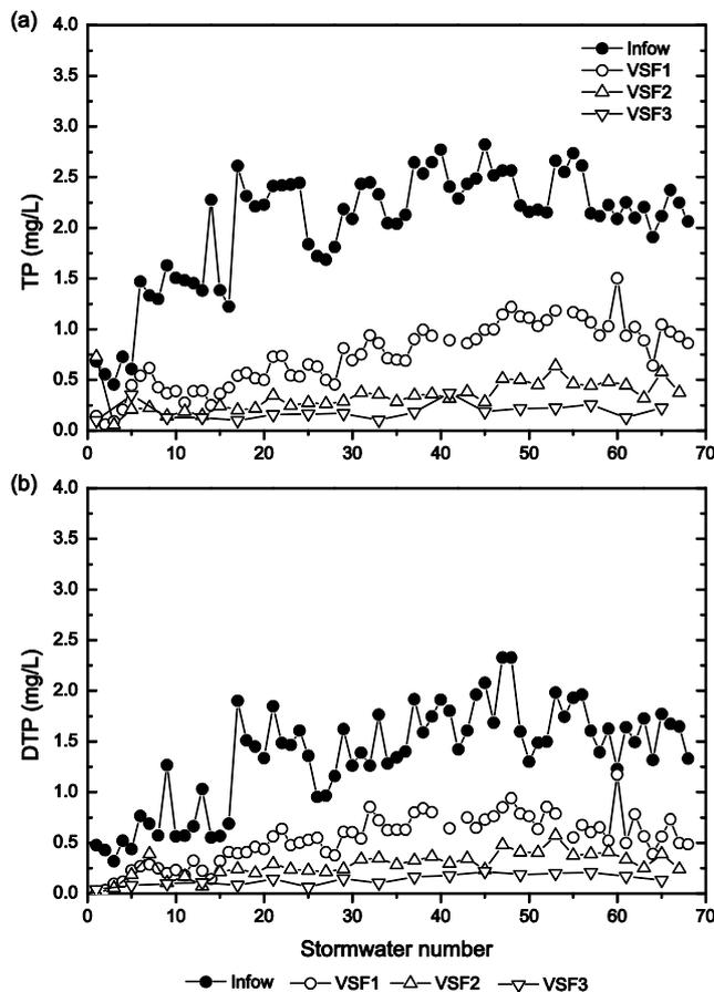
Fig. 6. Comparison of the phosphorus concentrations in the influent and effluent (a) TP; (b) DTP.
