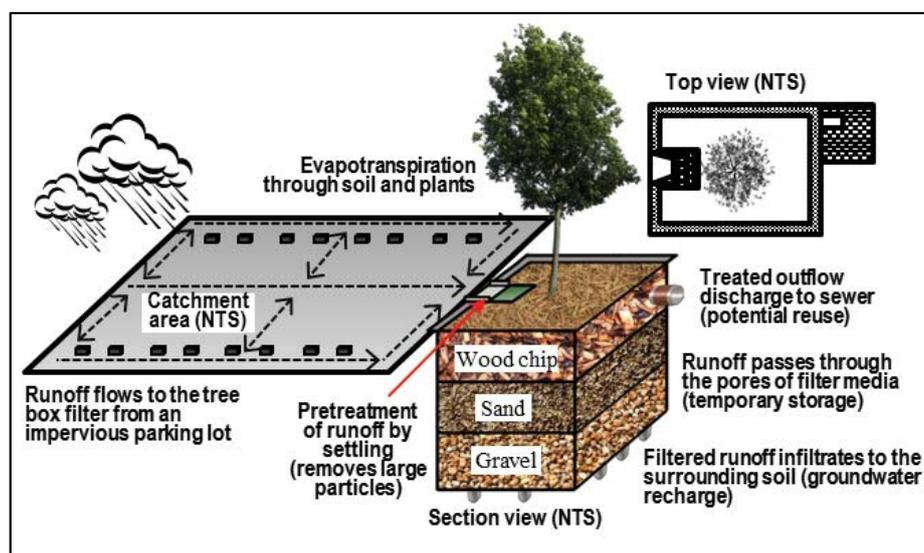
Fig. 1. Schematic diagram of the tree box filter.
