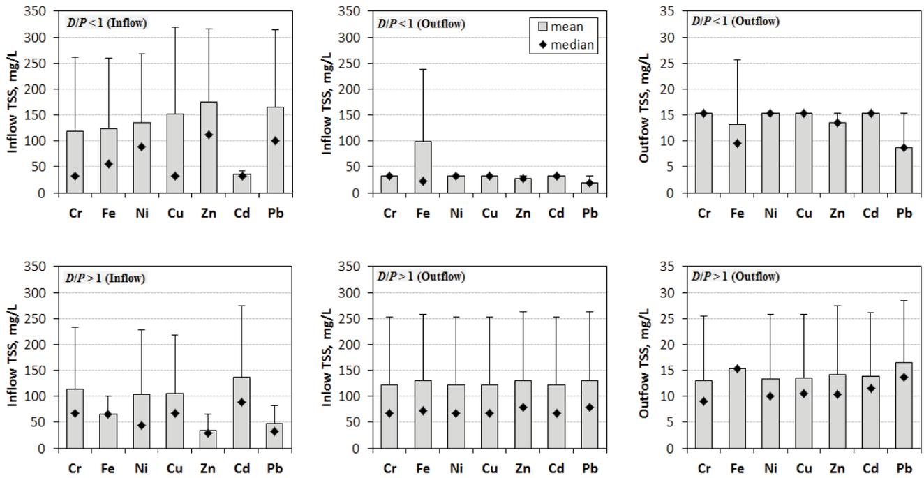
Fig. 4. Average (mean ± standard deviation and median) inflow and outflow TSS EMC for each heavy metal that correspond to various *D/P* criteria.
