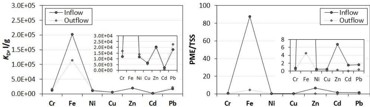
Fig. 5. Comparison of the distribution coefficient ( $K_D$ ) and particulate-bound metal element mass (PME/TSS) in the inflow and outflow.
