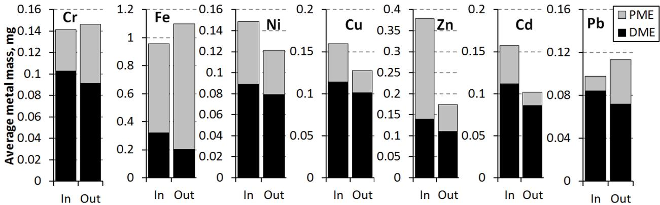
Fig. 2. Average mass loading of metal elements in inflow and outflow fractionated into particulate-bound (PME) and dissolved (DME) forms.
