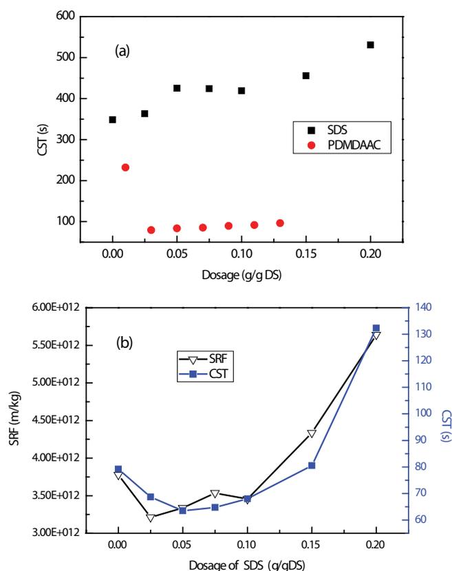
Fig. 1. Effect of SDS and PDMDAAC on sludge dewaterability: (a) SDS only and PDMDAAC only and (b) combined SDS with 0.03 g g<sup>-1</sup> DS PDMDAAC.
