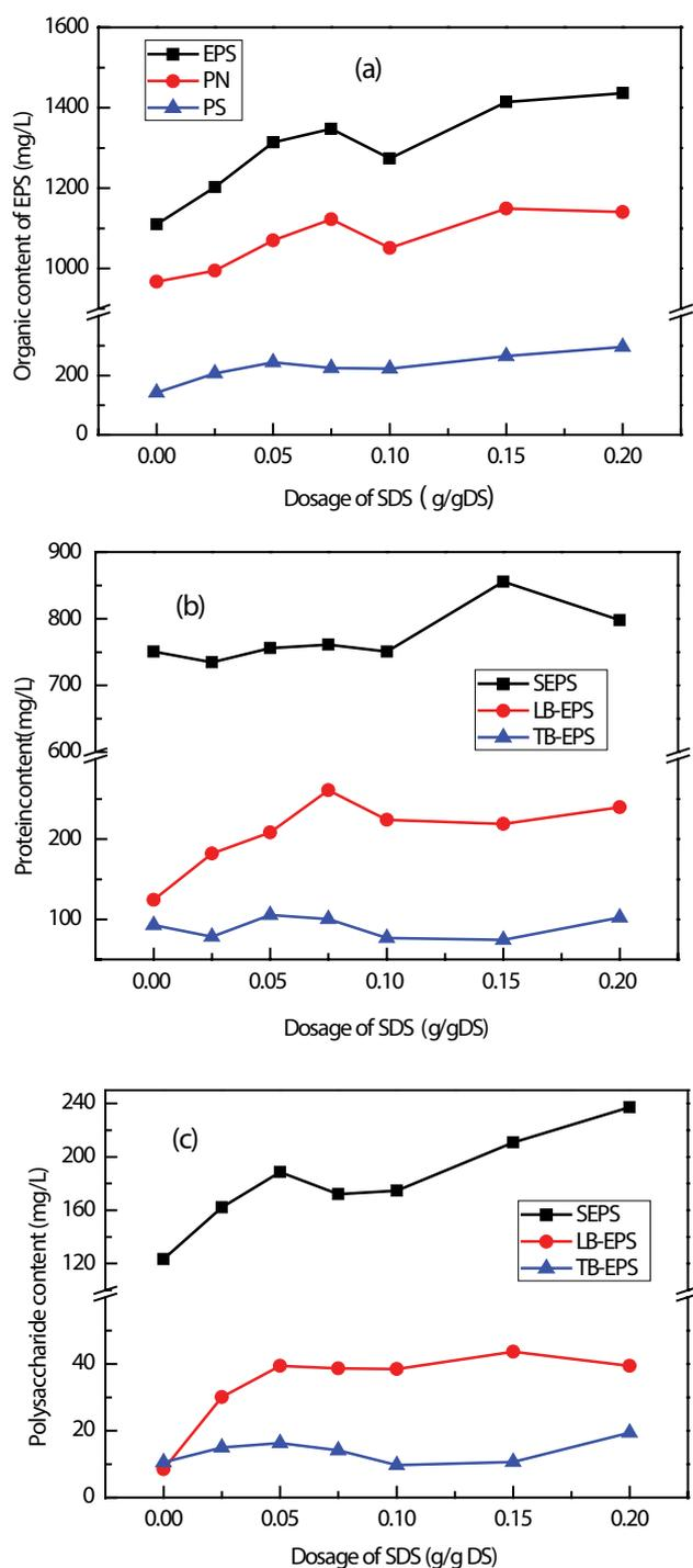
Fig. 3. Effect of combined SDS with PDMDAAC ( $0.03 \text{ g g}^{-1} \text{ DS}$ ) on content of (a) different EPS fractions, (b) proteins, and (c) polysaccharides.
