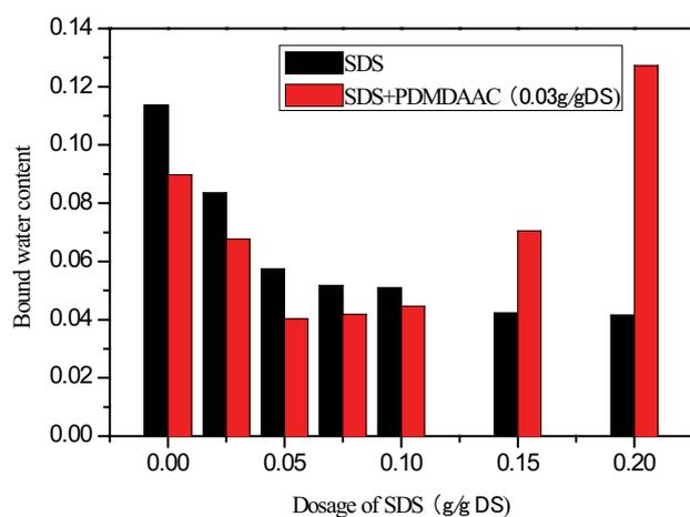
Fig. 6. Effect of SDS, combined SDS with PDMDAAC ( $0.03 \text{ g g}^{-1}$  DS) on bound water content of sludge.
