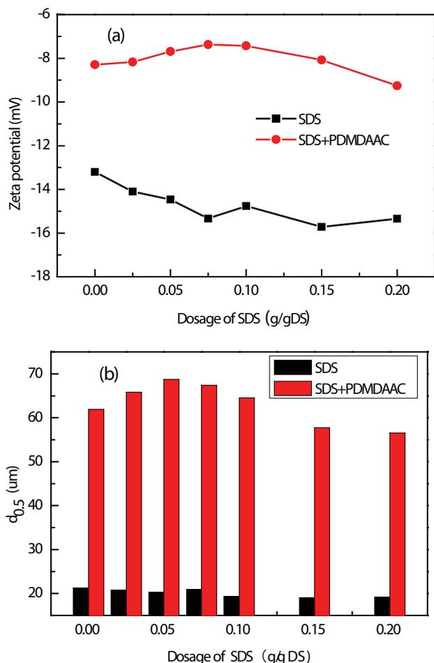
Fig. 5. Effect of SDS, combined SDS with PDMDAAC ( $0.03 \text{ g g}^{-1}$  DS) on (a) zeta potentials and (b) particle size of sludge.
