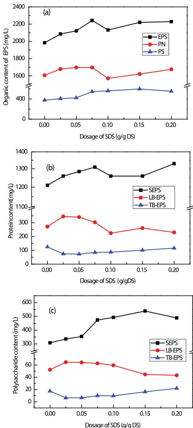
Fig. 2. Effect of SDS dosage on content of (a) different EPS fractions, (b) protein, and (c) polysaccharide.
