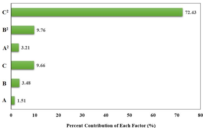
Fig. 2. Pareto chart of the percent contribution of each factor on COD removal (A = H<sub>2</sub>O<sub>2</sub> concentration, B = ferric concentration, C = pH).
