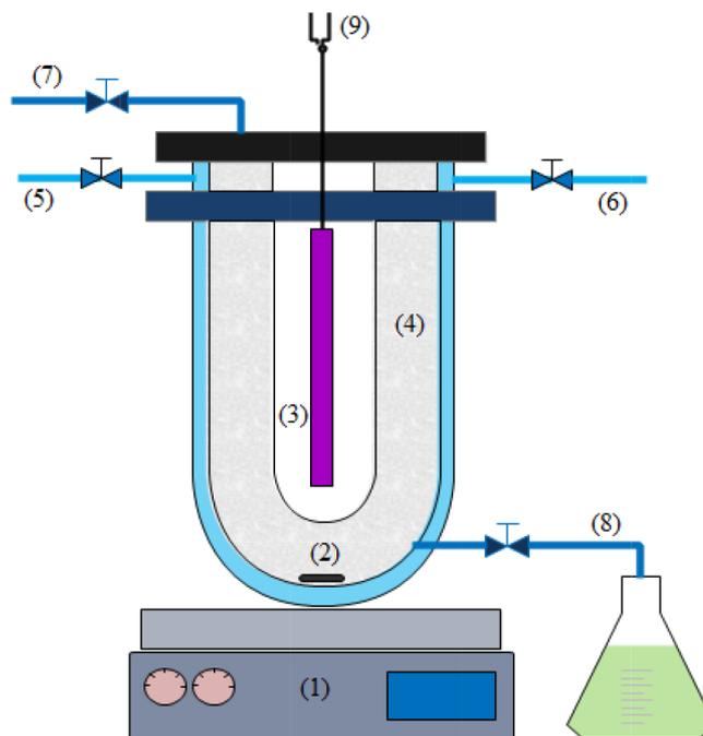
Fig. 1. Graphical diagram of the experimental reactor system: (1) Magnetic stirrer, (2) Magnetic stirrer bar, (3) UV lamp (it was switched off in this work), (4) Glass reactor, (5) Cooling water supply, (6) Cooling water return, (7) wastewater inlet, (8) Treated wastewater, (9) Electrical connection.
