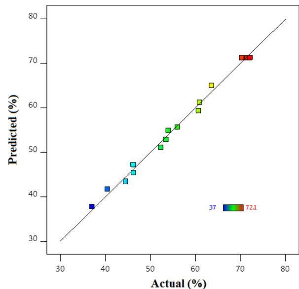
Fig. 3. Predicted vs. experimental values for the removal of COD in Fenton-like process.
