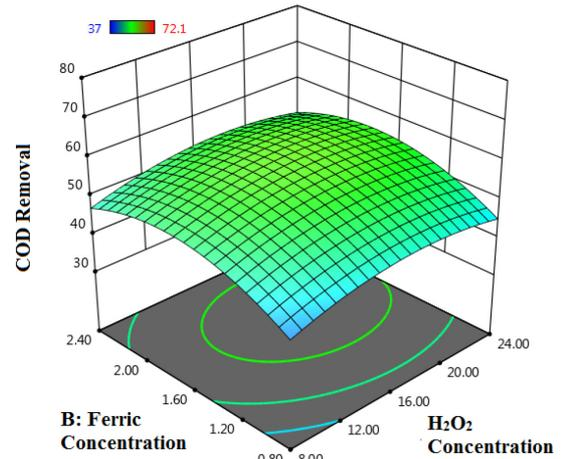
Fig. 5. (A) Surface plot in the removal of COD against: the ferric concentration ( $X_f$ ) and the concentration of  $H_2O_2$  ( $X_{CHP}$ ) at pH = 3.
