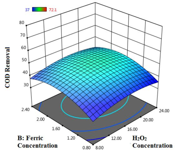
Fig. 5. (B) Surface of response for the removal efficiency of COD against: the ferric concentration ( $X_f$ ) and the concentration of  $H_2O_2$  ( $X_{CHP}$ ) at pH = 9.
