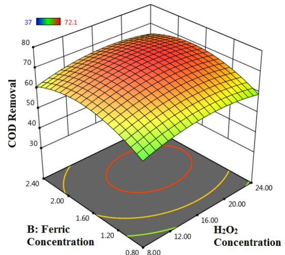
Fig. 5. (C) Surface of response in the removal efficiency of COD against: the dosage of ferric ions ( $X_{CF}$ ) and concentration of  $H_2O_2$  ( $X_{CHP}$ ) at pH = 6.
