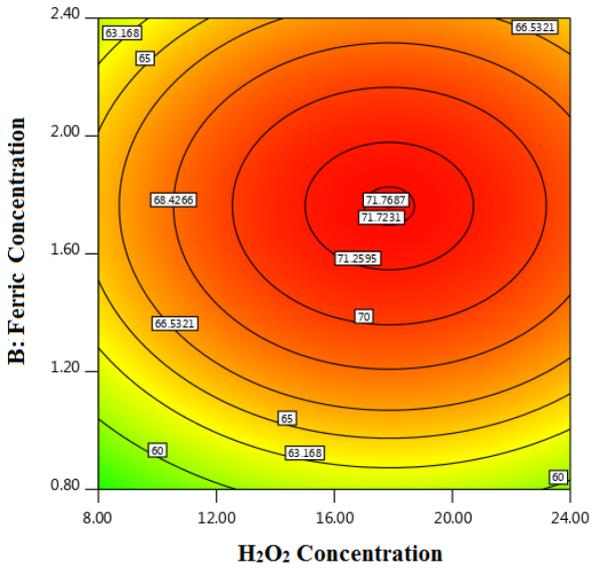
Fig. 4. Counter plot in the removal of COD against: the concentration of  $H_2O_2$  ( $X_{CHP}$ ) and ferric ions ( $X_{CF}$ ).
