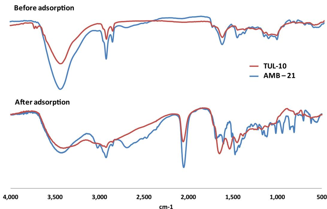
Fig. 9. FTIR spectra of resins.
