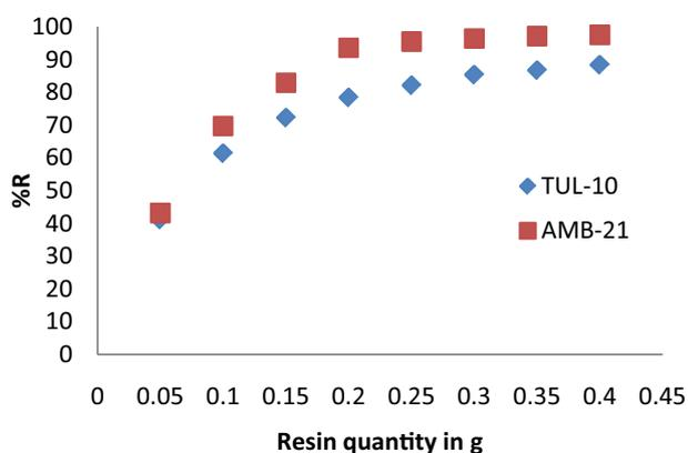
Fig. 4. Effect of resin dosage on the removal of thiocyanate.
