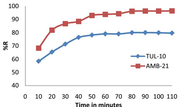
Fig. 3. Effect of contact time on the removal of thiocyanate.
