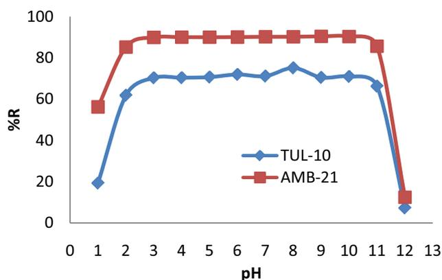
Fig. 1. Effect of pH on removal of thiocyanate using resins.
