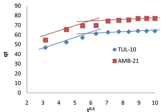
Fig. 7. Intra particle diffusion model of removal of thiocyanate.
