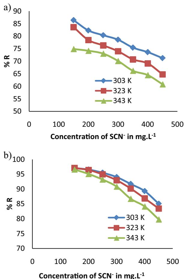
Fig. 2. Effect of thiocyanate concentration and temperature on removal of thiocyanate (a) On TUL-10 and (b) On AMB-21.
