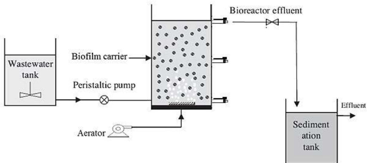
Fig. 1. Schematic of lab-scale MBBR.
