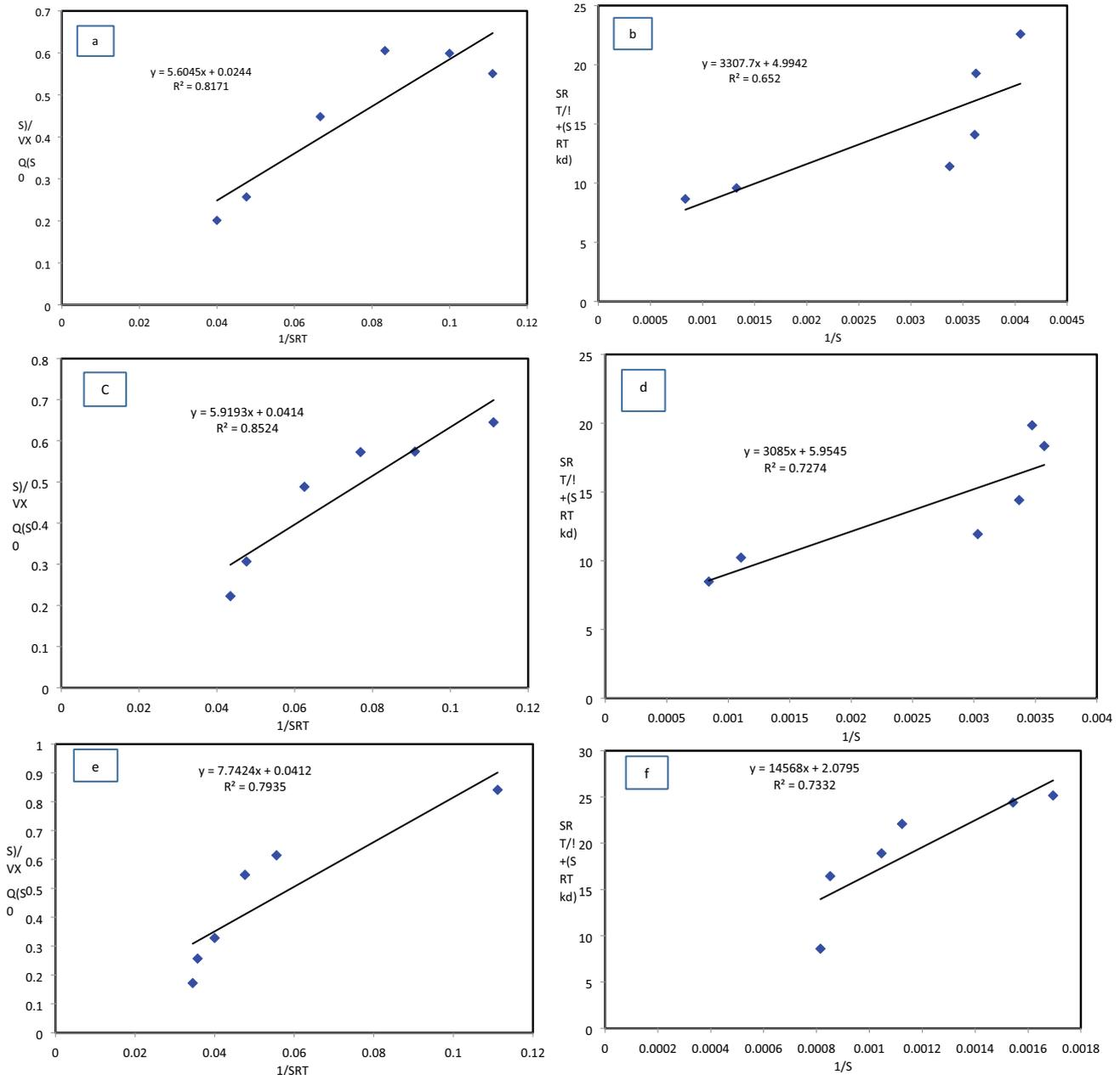
Fig. 6. Determination of biokinetic coefficients of halo-tolerant consortium in MBBR, (a)  $Y$  and  $k_d$  and (b)  $\mu$  and  $K_s$  for TDS concentration 25,000 mg L<sup>-1</sup>, (c)  $Y$  and  $k_d$  and (d)  $\mu$  and  $K_s$  for TDS concentration 30,000 mg L<sup>-1</sup>, (e)  $Y$  and  $k_d$  and (f)  $\mu$  and  $K_s$  for TDS concentration 35,000 mg L<sup>-1</sup>.
