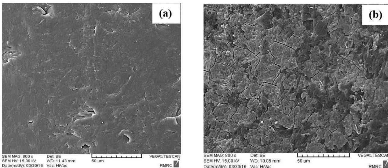
Fig. 2. Scanning electron microscopy (SEM) image of MBBR carrier before (a) and after (b) biofilm growth.
