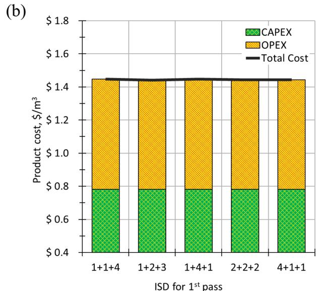
Fig. 13. CAPEX, OPEX and total product cost for ISD in the first pass using (a) two different membrane elements and (b) three different membrane elements.
