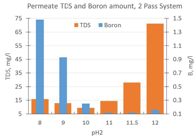
Fig. 6. Effect of the pH of the second pass on permeate TDS and boron contents.
