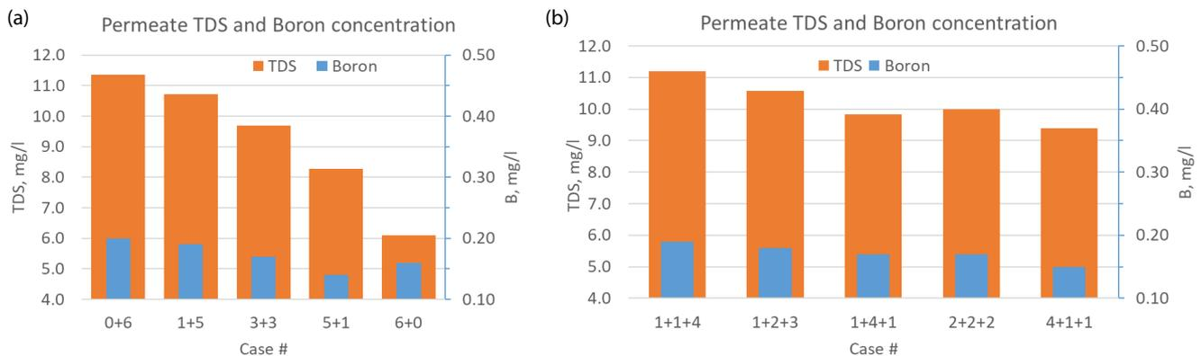
Fig. 8. TDS and boron concentration for ISD in the first pass only. (a) ISD with two types of membrane elements and (b) ISD using three types of membrane elements.
