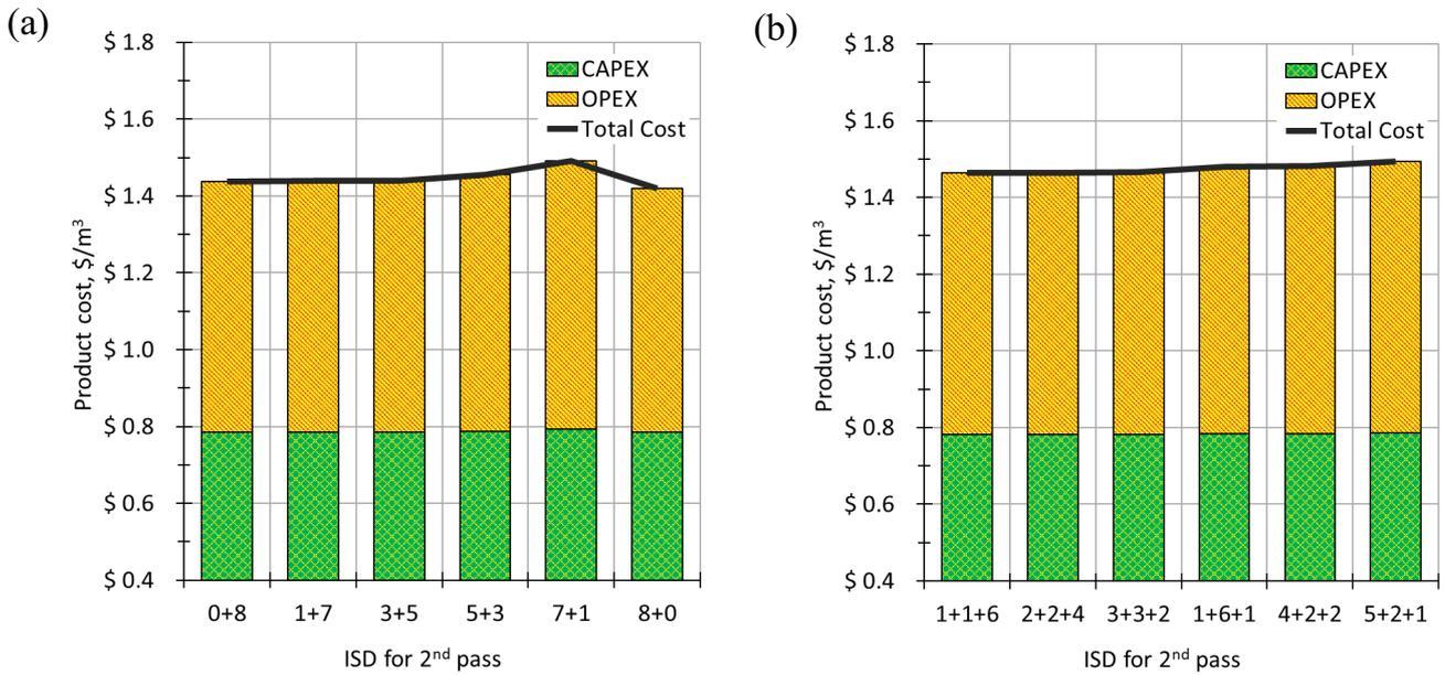
Fig. 14. CAPEX, OPEX and total product cost for ISD in the second pass using (a) two different membrane elements and (b) three different membrane elements.
