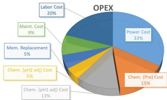
Fig. 12. OPEX breakdown for ISD in the first pass.
