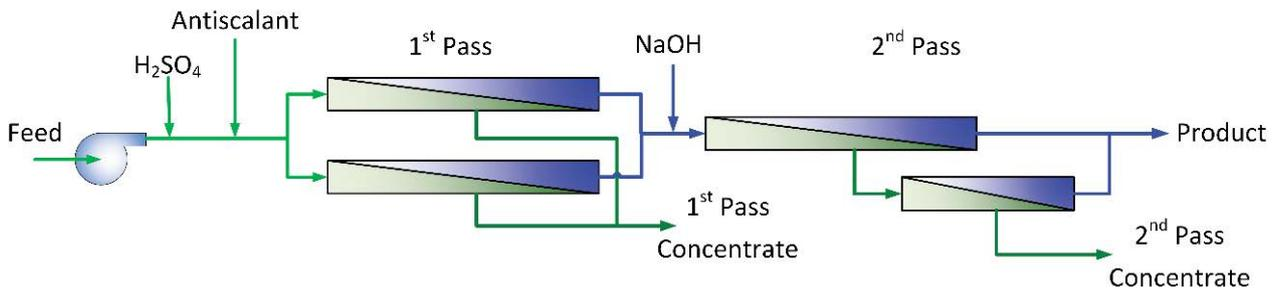
Fig. 3. Two passes system with pH control for the second pass.
