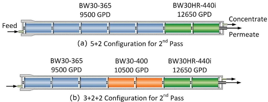
Fig. 2. ISD in the second pass, using two and three types of BW membrane elements in seven elements PV, (a) 5 + 2 configuration and (b) 3 + 2 + 2 configuration.
