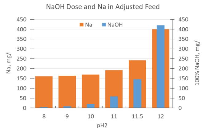
Fig. 7. NaOH dose and amount of Na in the adjusted feed.
