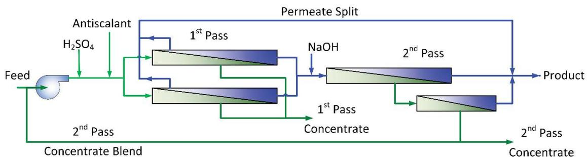
Fig. 5. Two passes system with permeate split and 2nd pass concentrate blending with 1st pass feed.
