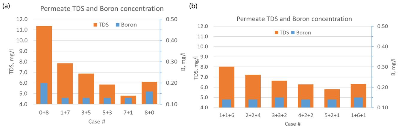
Fig. 9. TDS and boron concentration for ISD in the second pass only. (a) ISD with two types of membrane elements and (b) ISD using three types of membrane elements.
