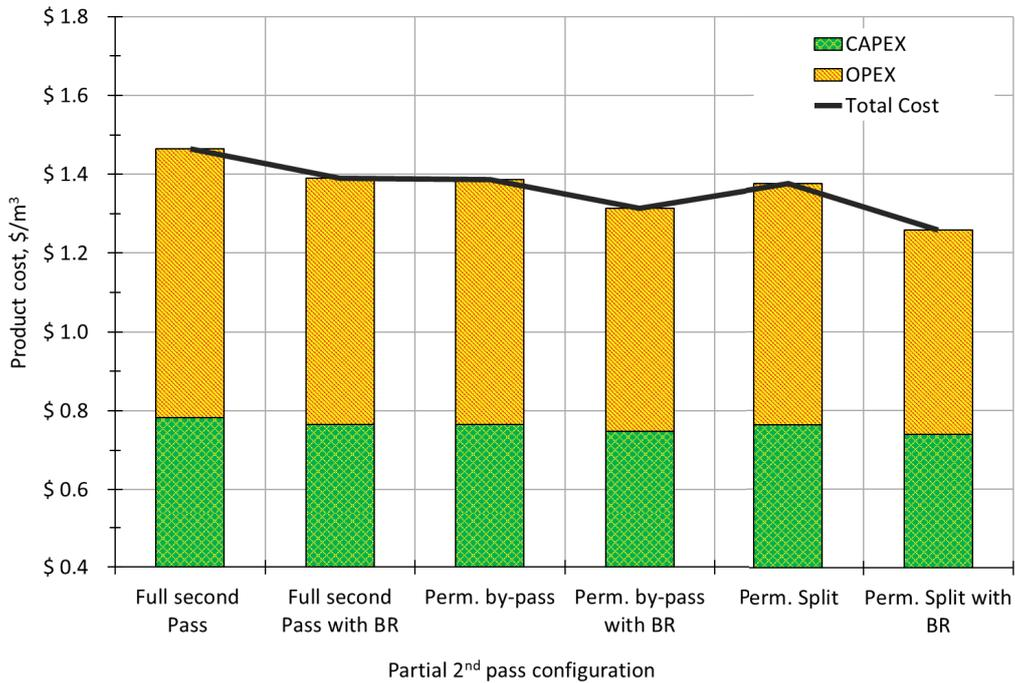
Fig. 15. CAPEX, OPEX and total product cost for different partial-second-pass configurations.
