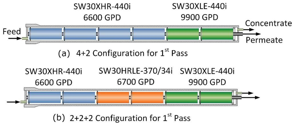
Fig. 1. ISD in the first pass, using two and three types of SW membrane elements in six elements PV, (a) 4 + 2 configuration and (b) 2 + 2 + 2 configuration.
