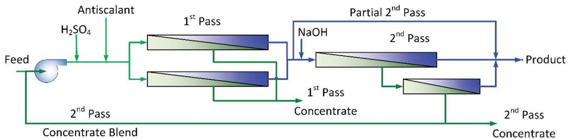
Fig. 4. Partial second pass system and concentrate blending.
