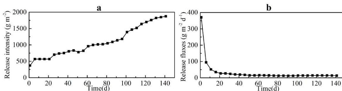
Fig. 6. Cumulative sediment release intensity and fluxes of Beitang Reservoir. (a) Cumulative sediment release intensity; (b) sediment release fluxes.
