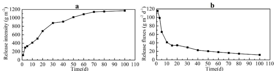
Fig. 5. Cumulative sediment release intensity and fluxes in the tested pool. (a) cumulative sediment release intensity; (b) sediment release fluxes.
