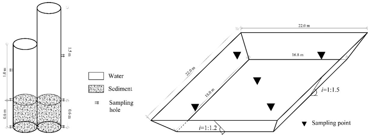
Fig. 2. Schematic diagram of laboratory experiments and pool experiments. (a) The column 5# (left) and 5# (right). The settings of other columns were similar to 5#; (b) The depth of the tested pool was 1.67 m.
