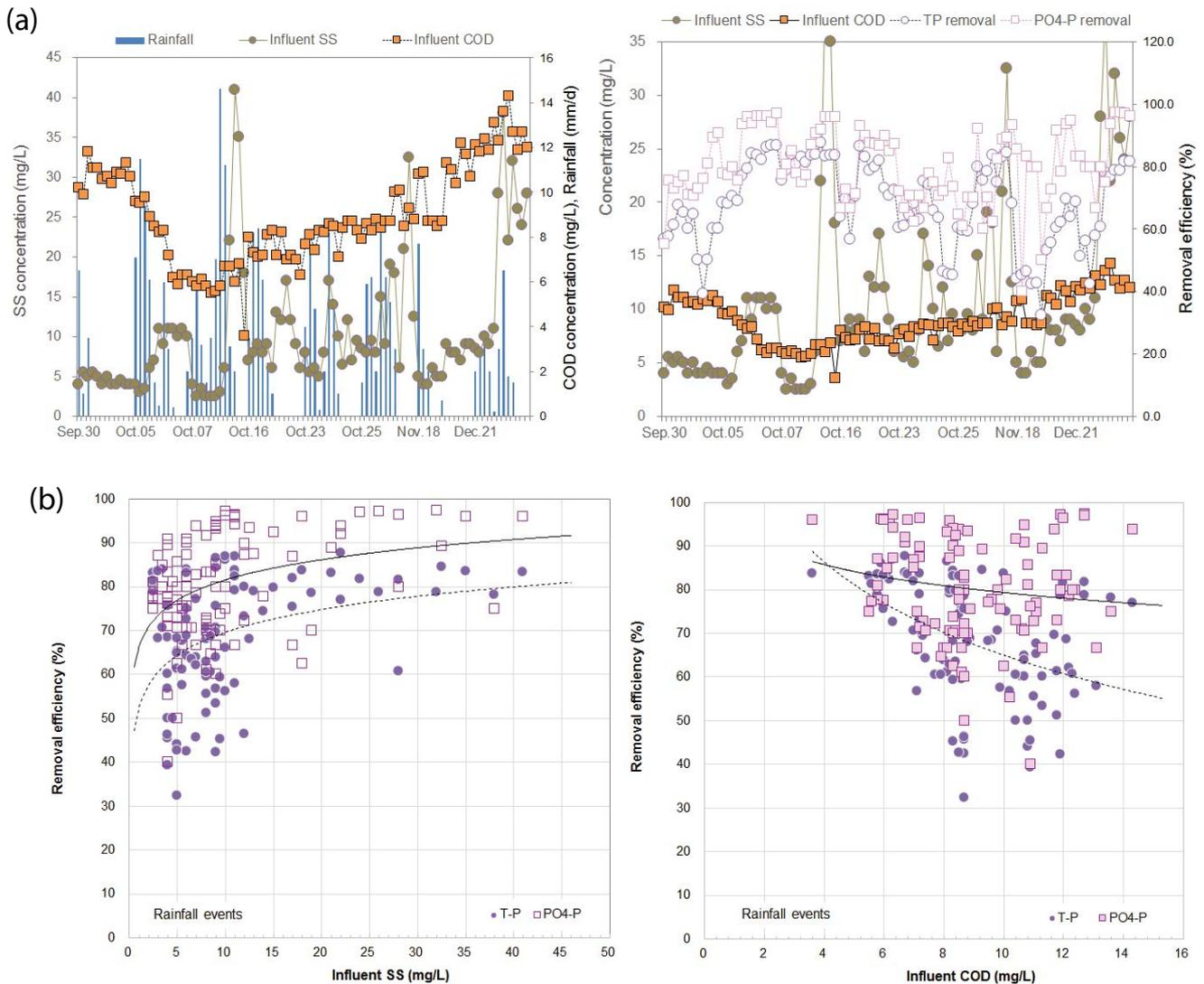
Fig. 6. Variation in P removal efficiency with water quality during rainfall events. (a) P removal efficiency and water quality of influent for rainfall events and (b) P removal efficiency vs. influent SS and COD concentrations.
