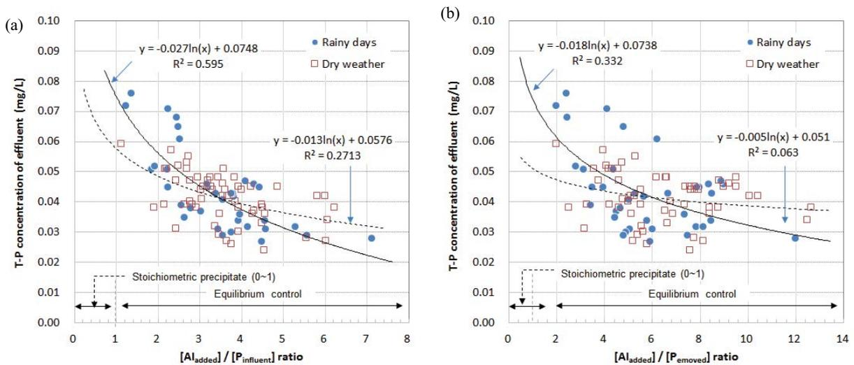
Fig. 8. Empirical values of molar ratios  $[Al]/[P]$  based on the PTPP operation data. (a) Molar ratios of added Al:influent P and (b) molar ratios of added Al:removed P.
