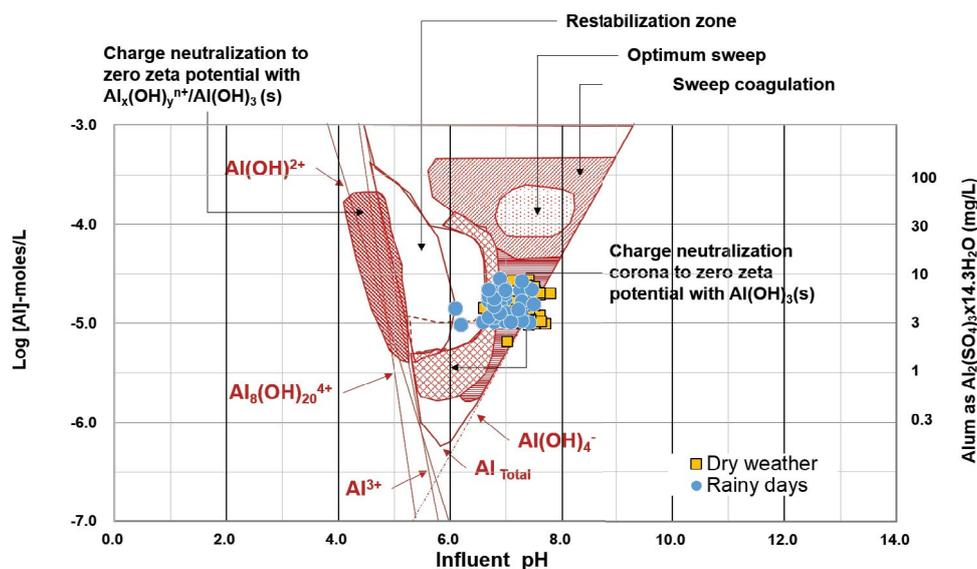
Fig. 9. Operated regime of coagulant dose in PTPP for P removal, based on Johnson and Amirtharajah [22], and Amirtharajah and Mills diagram [23].
