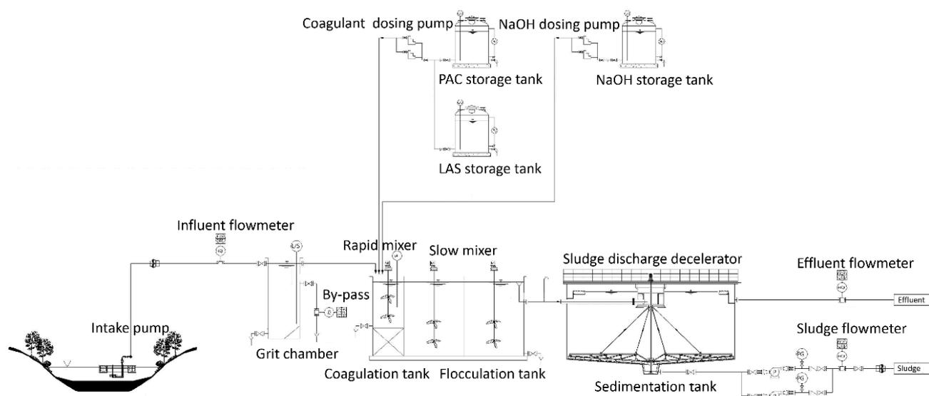
Fig. 2. Schematic diagram of the phosphorus treatment pilot plant (PTPP).
