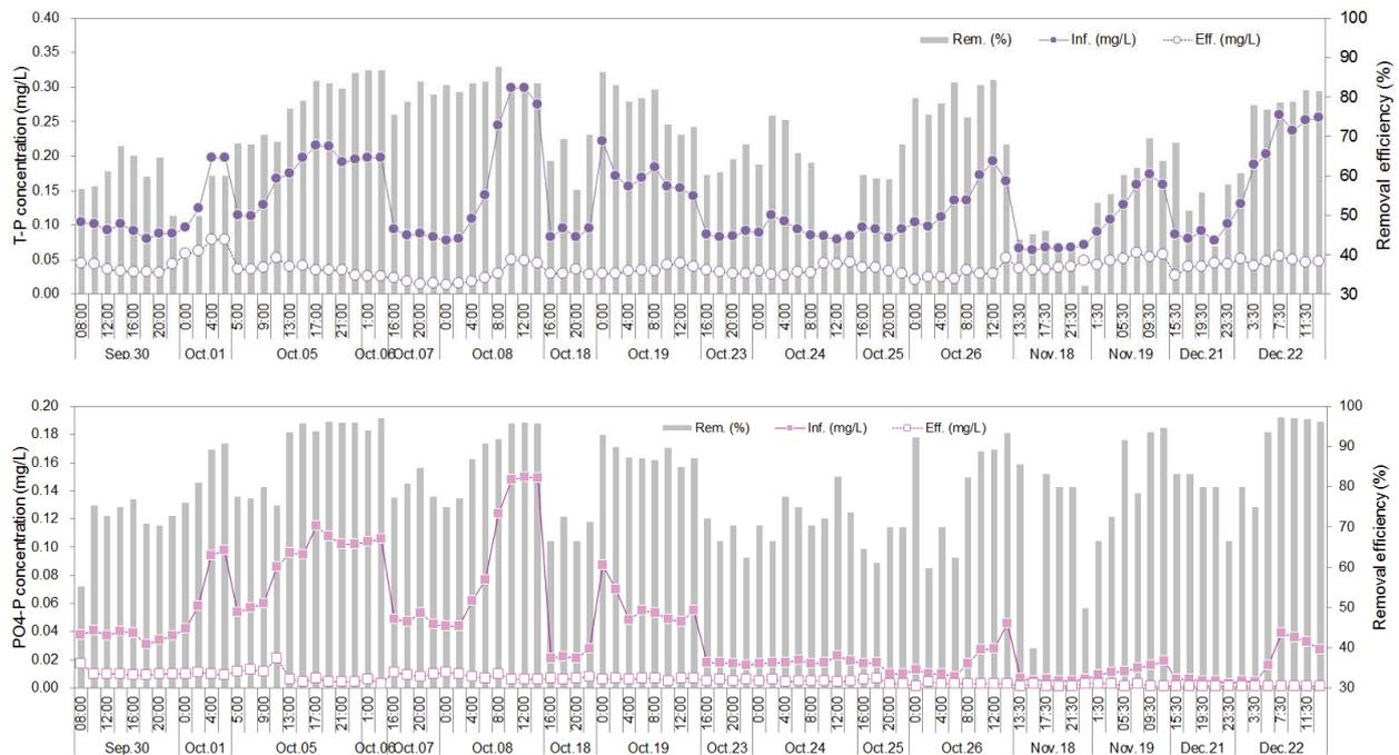
Fig. 4. P concentration and removal efficiency during rainfall events.
