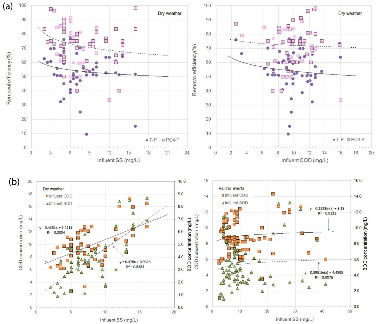
Fig. 7. Variation in P treatment efficiency and change in water quality for dry weather and rainfall events.
