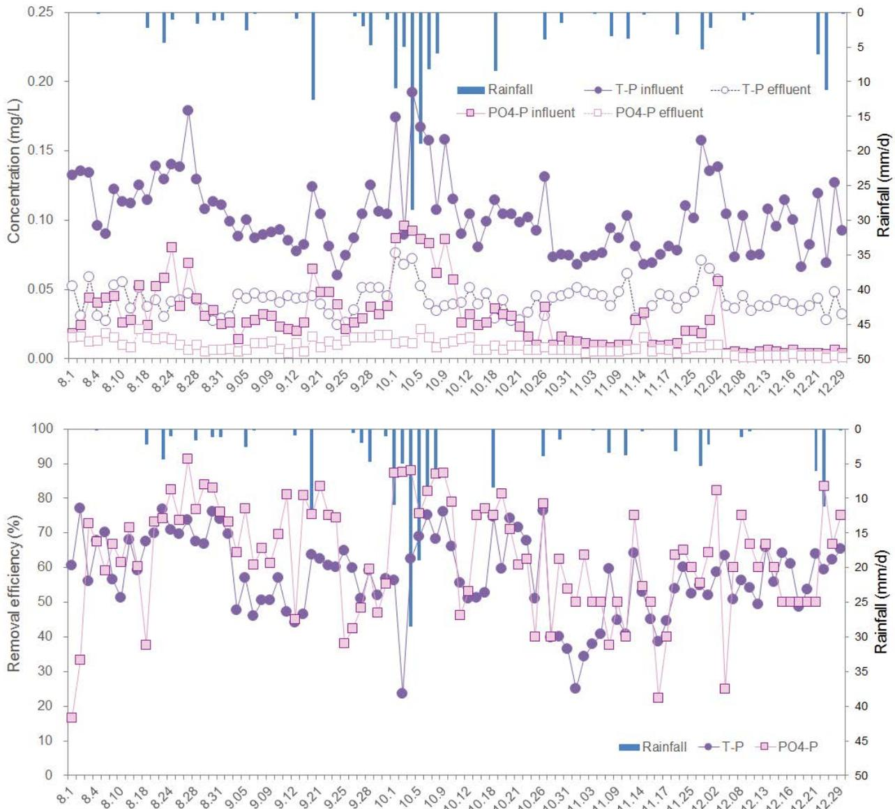
Fig. 3. Changes in phosphorus concentration and removal efficiency vs. operation time for PTPP.
