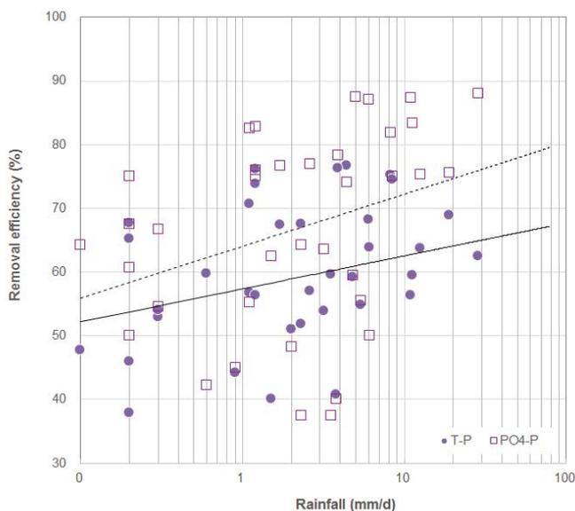
Fig. 5. P removal efficiency vs. rainfall intensity.
